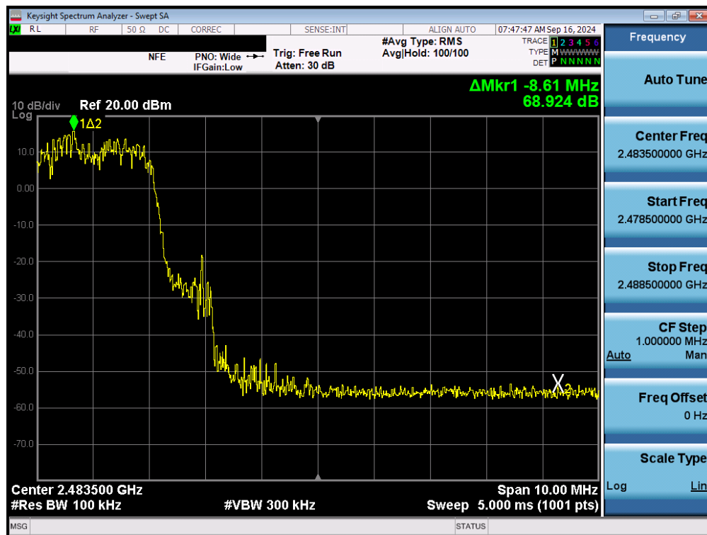
Plot 7-118. Band Edge Plot (Bluetooth with Hopping Enabled, 3 Mbps) – Ant 2
