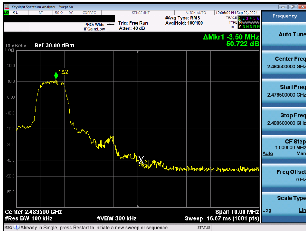
Plot 7-120. Band Edge Plot (Bluetooth with Hopping Disabled, 3 Mbps – Ch. 78) – Dual Ant 1
