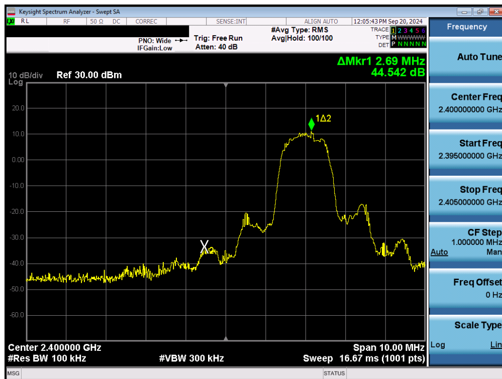
Plot 7-119. Band Edge Plot (Bluetooth with Hopping Disabled, 3 Mbps – Ch. 0) – Dual Ant 1
