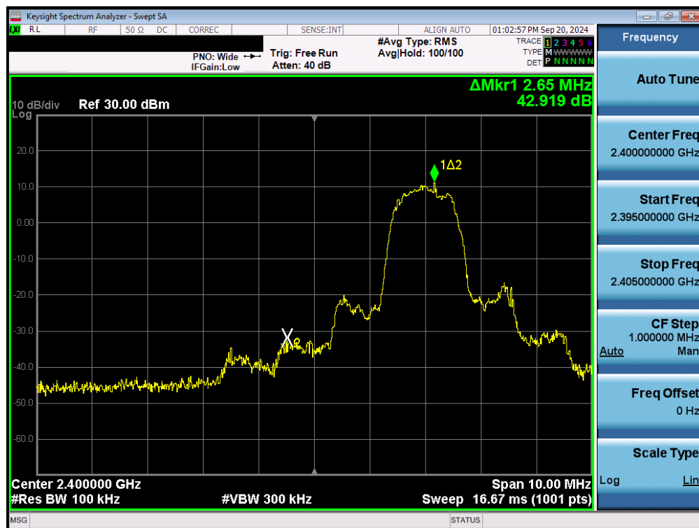
Plot 7-123. Band Edge Plot (Bluetooth with Hopping Disabled, 3 Mbps – Ch. 0) – Dual Ant 2
