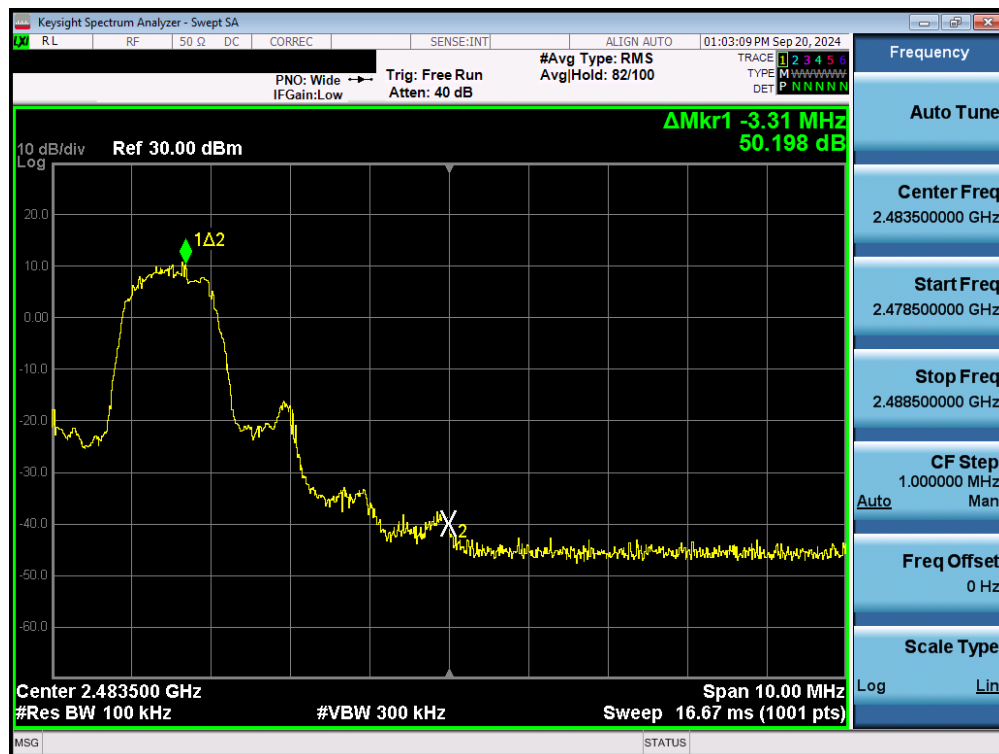
Plot 7-124. Band Edge Plot (Bluetooth with Hopping Disabled, 3 Mbps – Ch. 78) – Dual Ant 2
