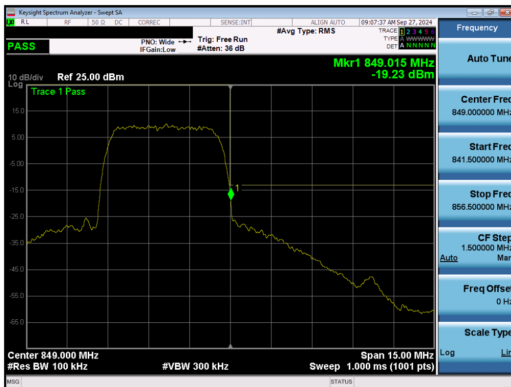
Plot 7-75. Upper Band Edge Plot (WCDMA Cell – Ch. 4233 – Ant1)
