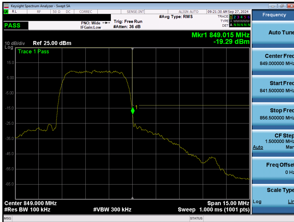
Plot 7-83. Upper Band Edge Plot (WCDMA Cell – Ch. 4233 – Ant2)
