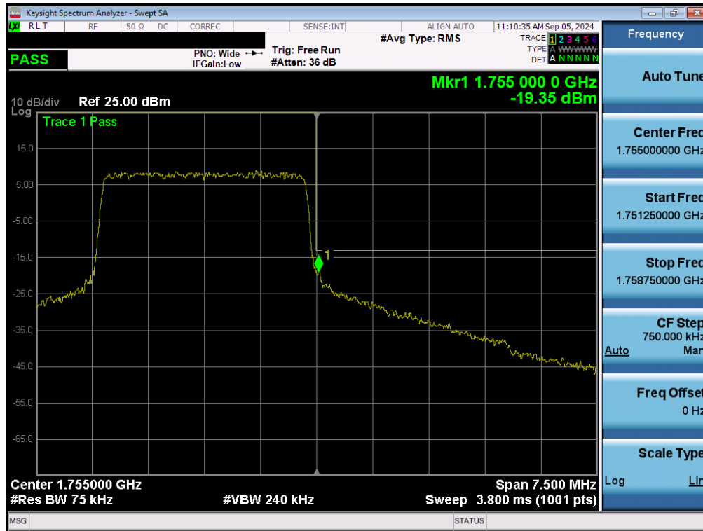
Plot 7-122. Upper Band Edge Plot (LTE Band 4 - 3MHz QPSK – Full RB - ANT1)
