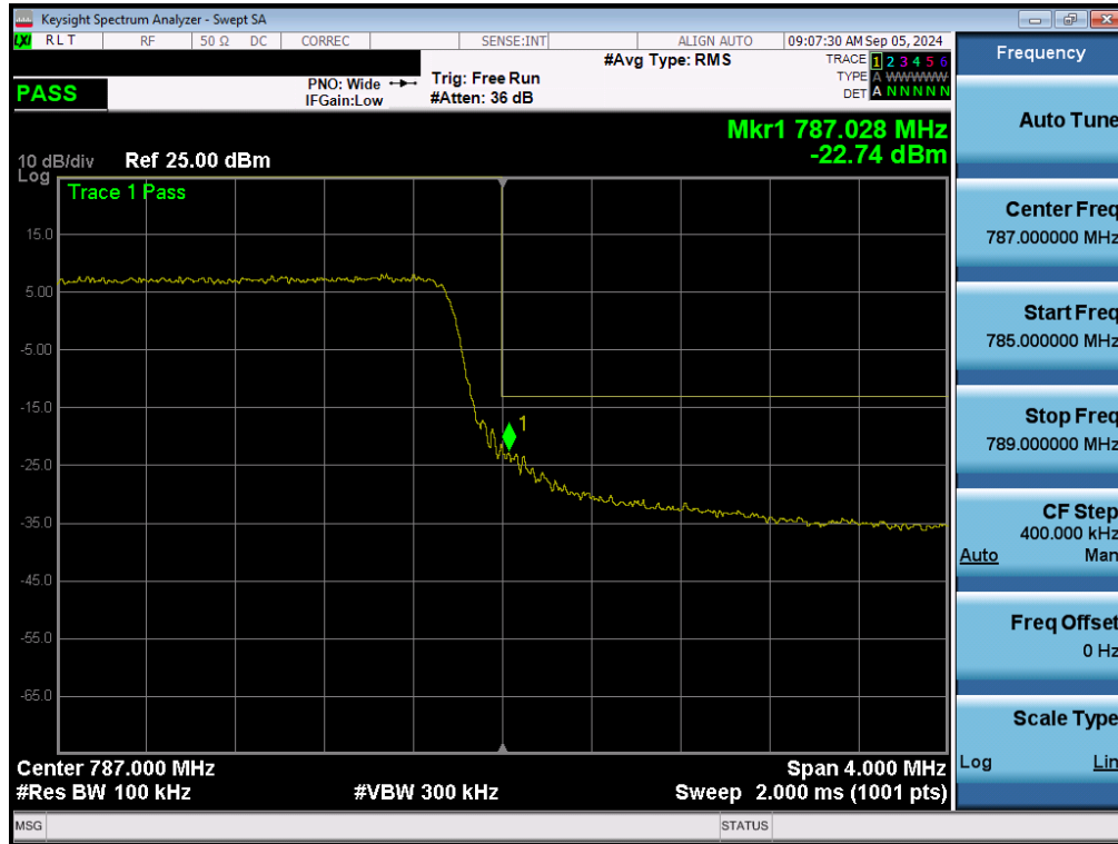
Plot 7-118. Upper Band Edge Plot (LTE Band 13 - 5MHz QPSK - Full RB - ANT1)
