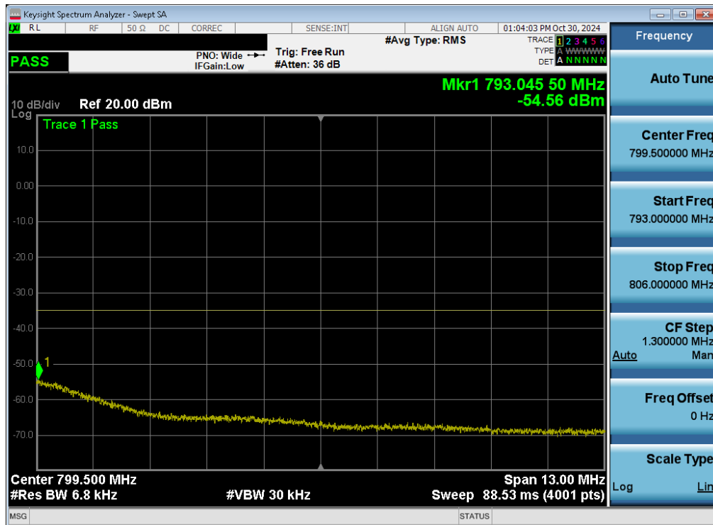
Plot 7-119. Upper Emission Mask Plot (LTE Band 13 - 5MHz QPSK - Full RB - ANT1)
