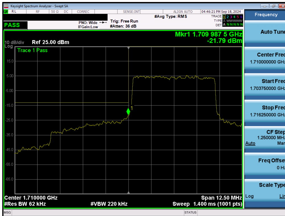
Plot 7-136. Lower Band Edge Plot (NR Band n66 – 5MHz - Full RB - ANT2)
