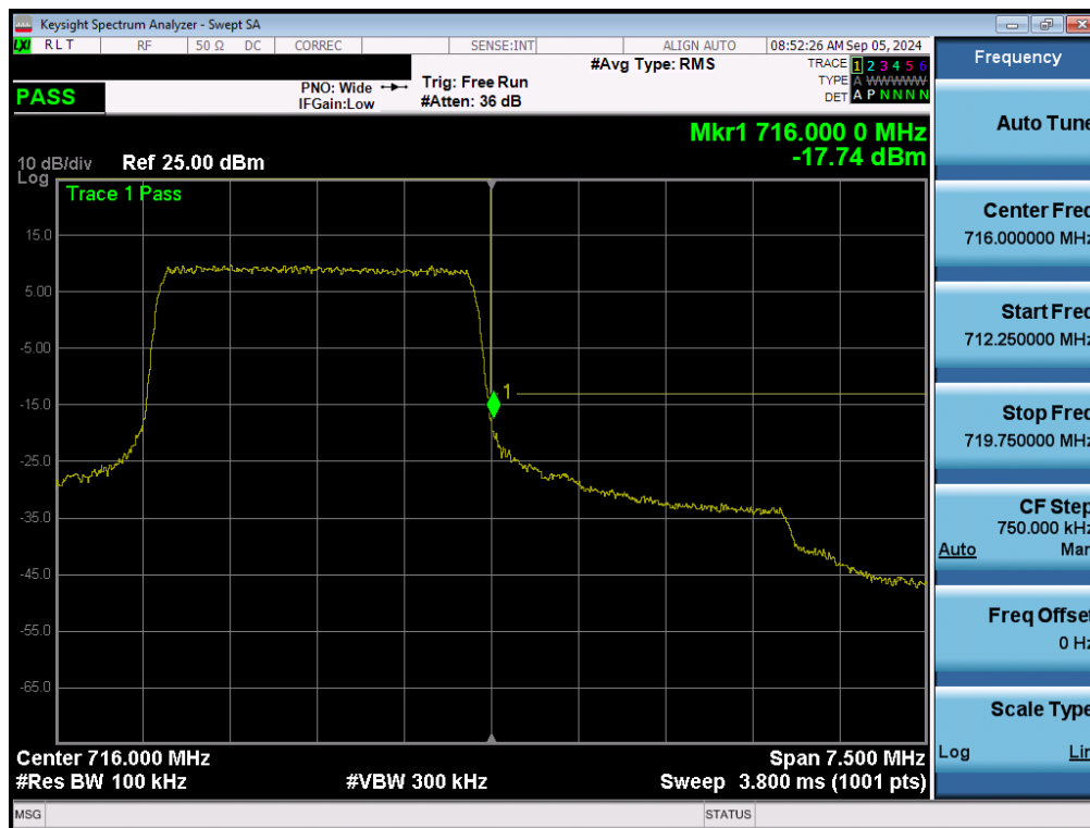
Plot 7-115. Upper Band Edge Plot (LTE Band 12 – 3MHz QPSK – Full RB - ANT1)
