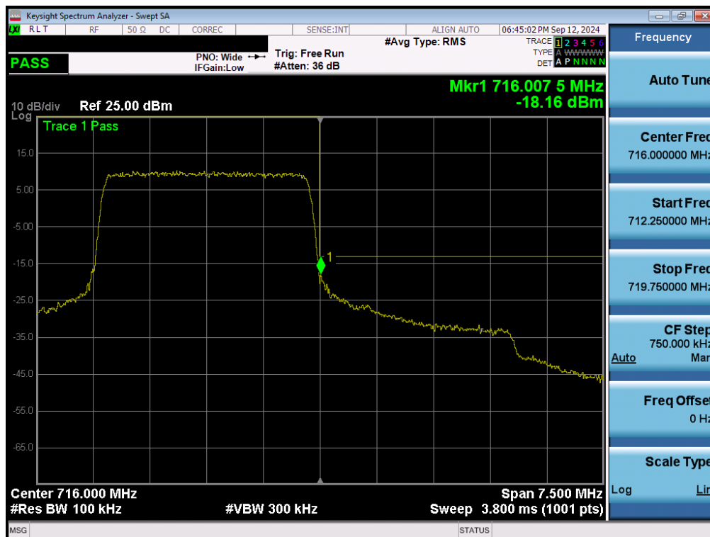
Plot 7-131. Upper Band Edge Plot (LTE Band 12 – 3MHz QPSK – Full RB - ANT2)
