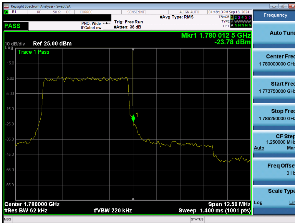
Plot 7-138. Upper Band Edge Plot (NR Band n66 – 5MHz - Full RB - ANT2)
