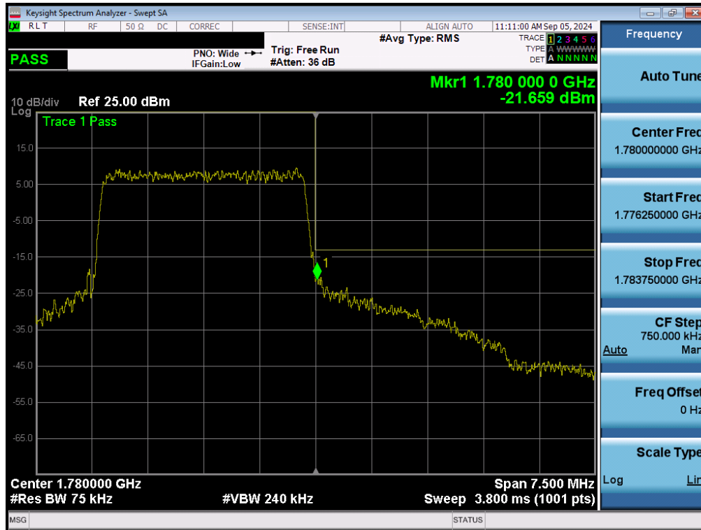
Plot 7-124. Upper Band Edge Plot (LTE Band 66 - 3MHz QPSK – Full RB - ANT1)
