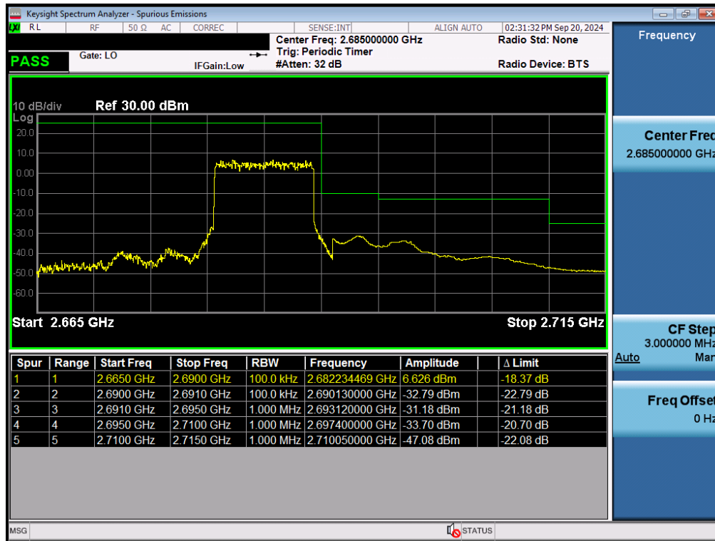
Plot 7-134. Upper Band Edge Plot (NR Band n41 - 10MHz DFT-s-OFDM-BPSK – Full RB - Ant B)
