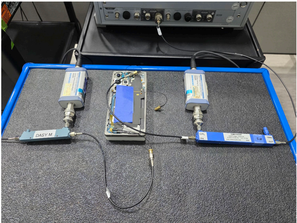
Test Setup Photo 4 – Conducted Test Setup (Figure 5-1c)
