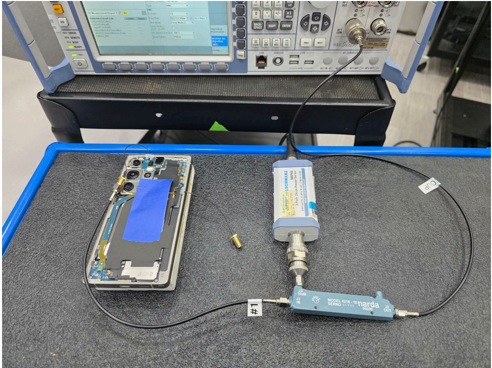
Test Setup Photo 3 – Conducted Test Setup (Figure 5-1a)
