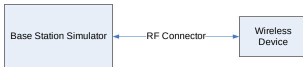
Figure 10-4 Power Measurement Setup – NR FDD
