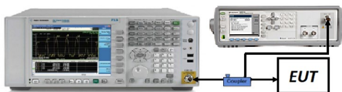
Figure 7-2. Test Instrument & Measurement Setup
