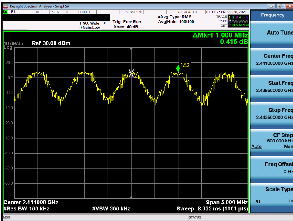
Plot 7-128. Channel Spacing Plot (Bluetooth) – Dual Ant 2
