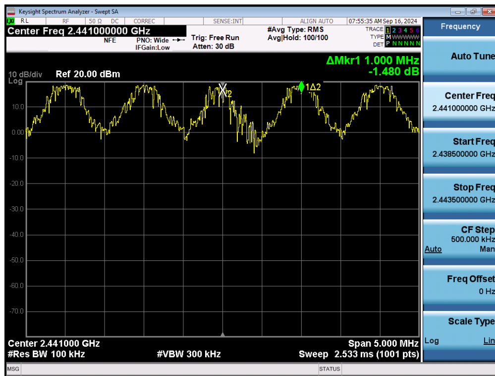
Plot 7-126. Channel Spacing Plot (Bluetooth) – Ant 2
