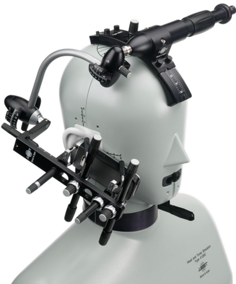
Figure 4-3 Heat and Torso Simulator (with Handset Positioner)
