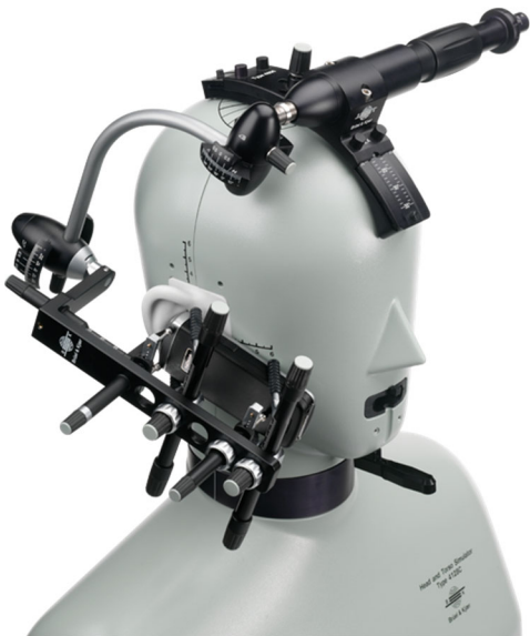
Figure 4-3 Heat and Torso Simulator (with Handset Positioner)
