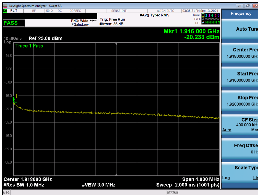
Plot 7-157. Extended Upper Band Edge Plot (NR Band n25 - 10MHz QPSK – Full RB - Ant2)
