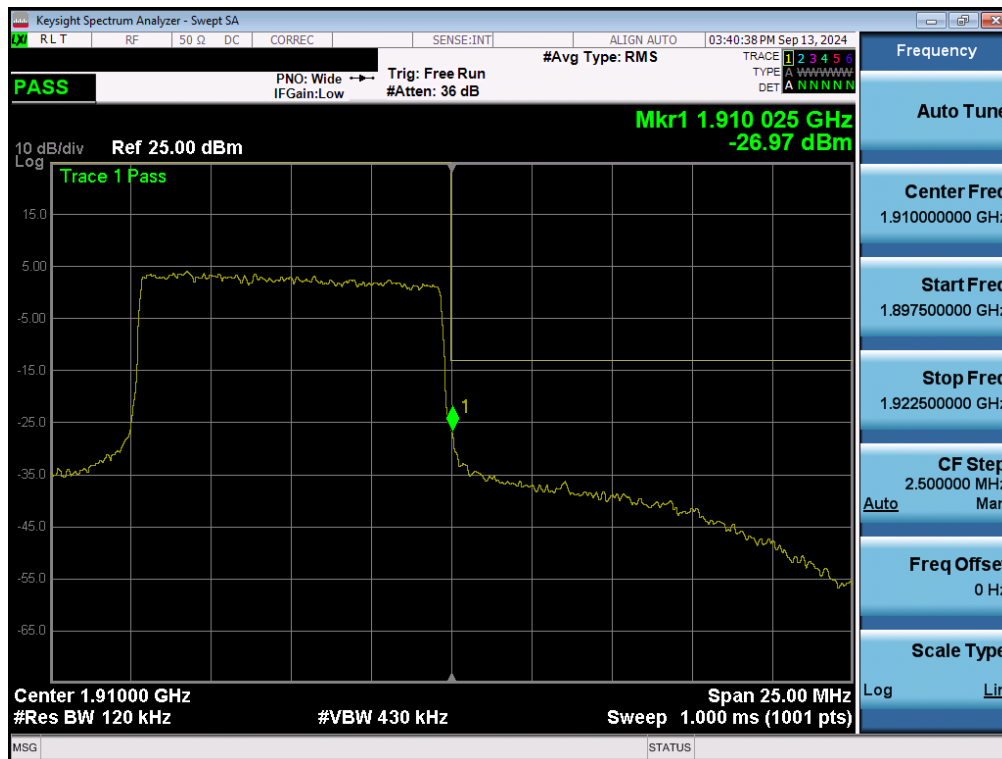
Plot 7-154. Upper Band Edge Plot (NR Band n2 - 10MHz QPSK – Full RB - Ant2)
