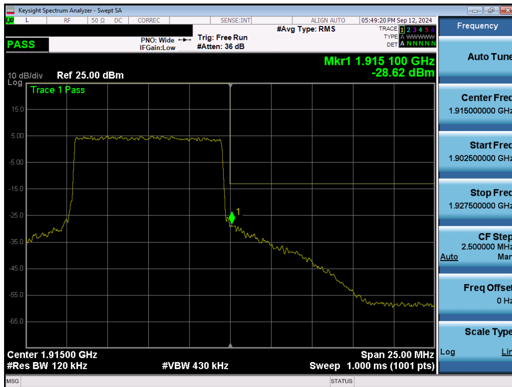
Plot 7-138. Upper Band Edge Plot (LTE Band 25 - 10MHz QPSK - Full RB - Ant1)
