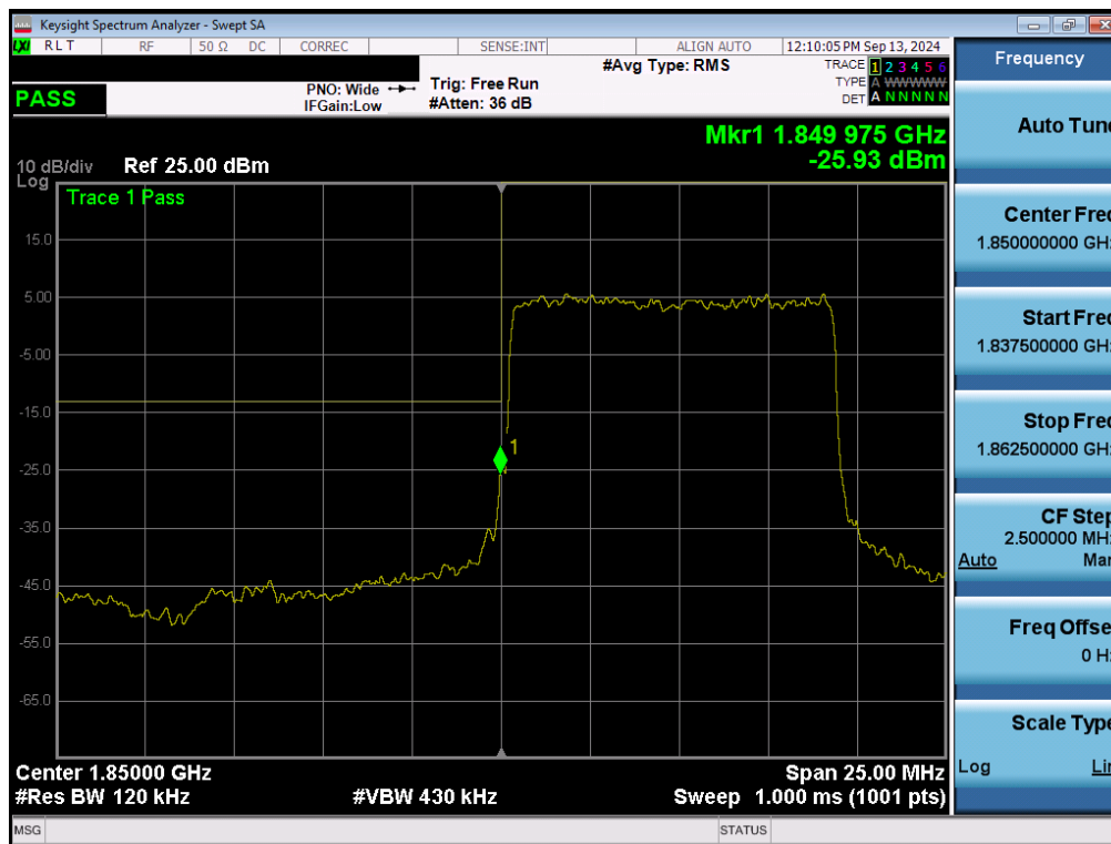
Plot 7-146. Lower Band Edge Plot (NR Band n25/2 - 10MHz QPSK – Full RB - Ant1)
