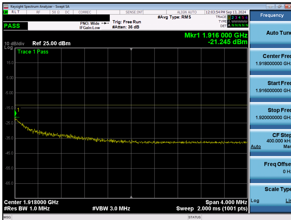
Plot 7-151. Extended Upper Band Edge Plot (NR Band n25 - 10MHz QPSK – Full RB - Ant1)
