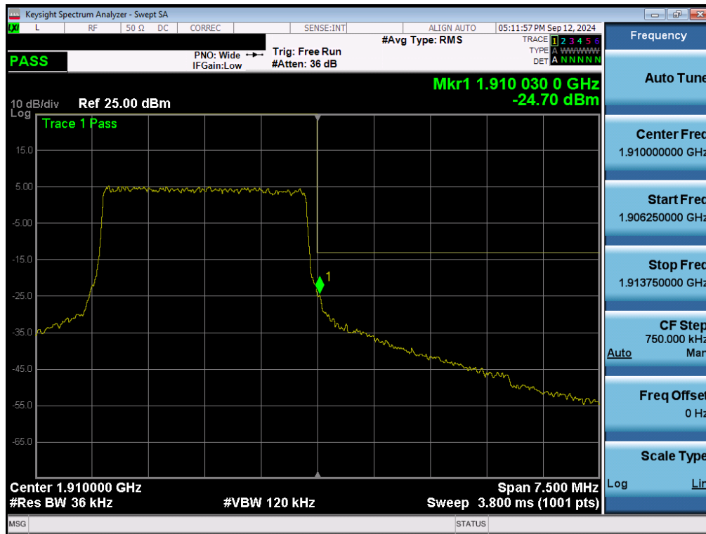
Plot 7-142. Upper Band Edge Plot (LTE Band 2 - 3MHz QPSK – Full RB - Ant2)
