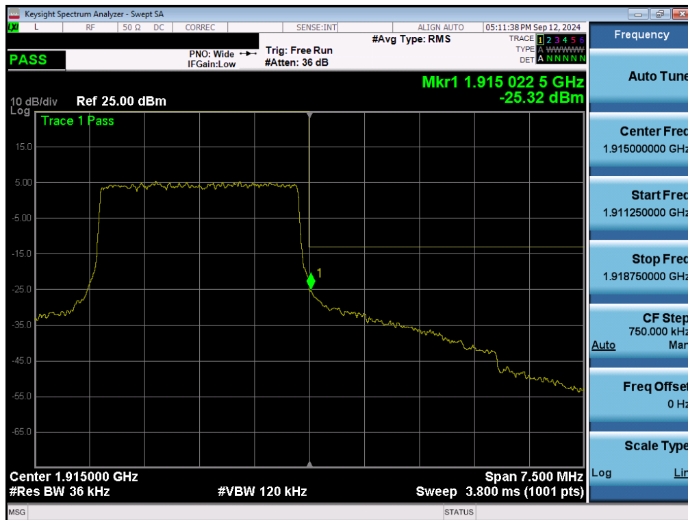
Plot 7-144. Upper Band Edge Plot (LTE Band 25 - 3MHz QPSK – Full RB - Ant2)
