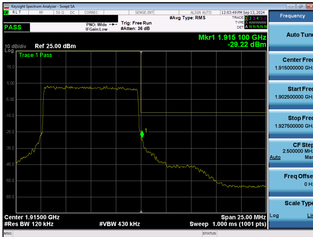
Plot 7-150. Upper Band Edge Plot (NR Band n25 - 10MHz QPSK – Full RB - Ant1)
