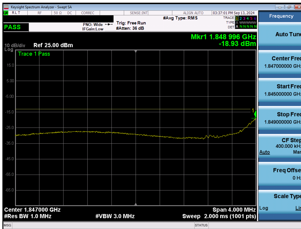
Plot 7-153. Extended Lower Band Edge Plot (NR Band n25/2 - 10MHz QPSK – Full RB - Ant2)
