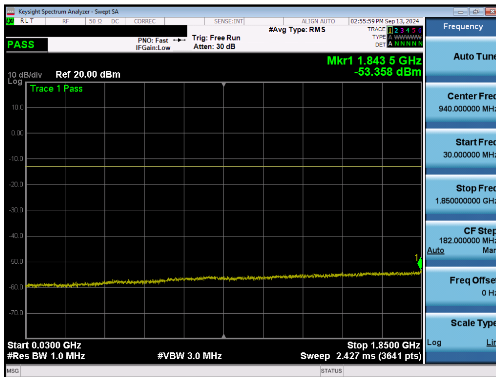
Plot 7-124. Conducted Spurious Plot (NR Band n25/2 - 40.0MHz - 1RB - Mid Channel - Ant2)
