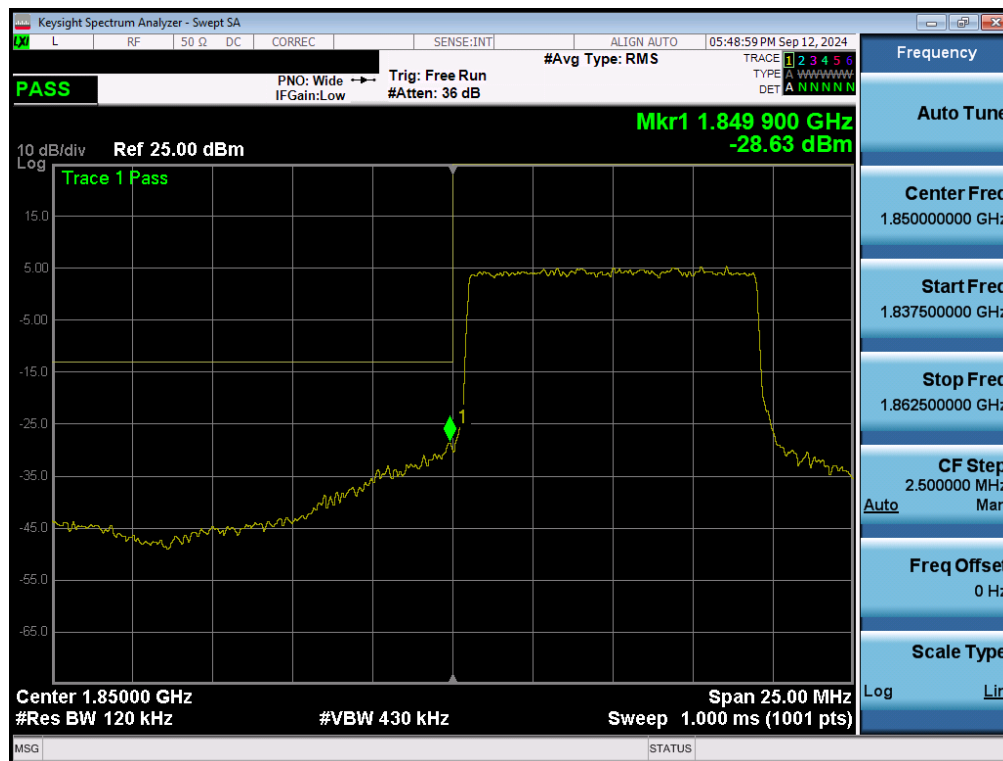
Plot 7-134. Lower Band Edge Plot (LTE Band 25/2 - 10MHz QPSK – Full RB - Ant1)
