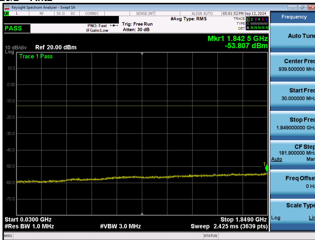
Plot 7-112. Conducted Spurious Plot (LTE Band 25/2 - 20MHz QPSK - 1RB - Low Channel - Ant2)
