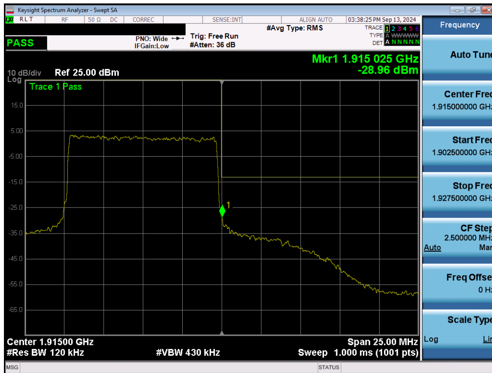
Plot 7-156. Upper Band Edge Plot (NR Band n25 - 10MHz QPSK – Full RB - Ant2)
