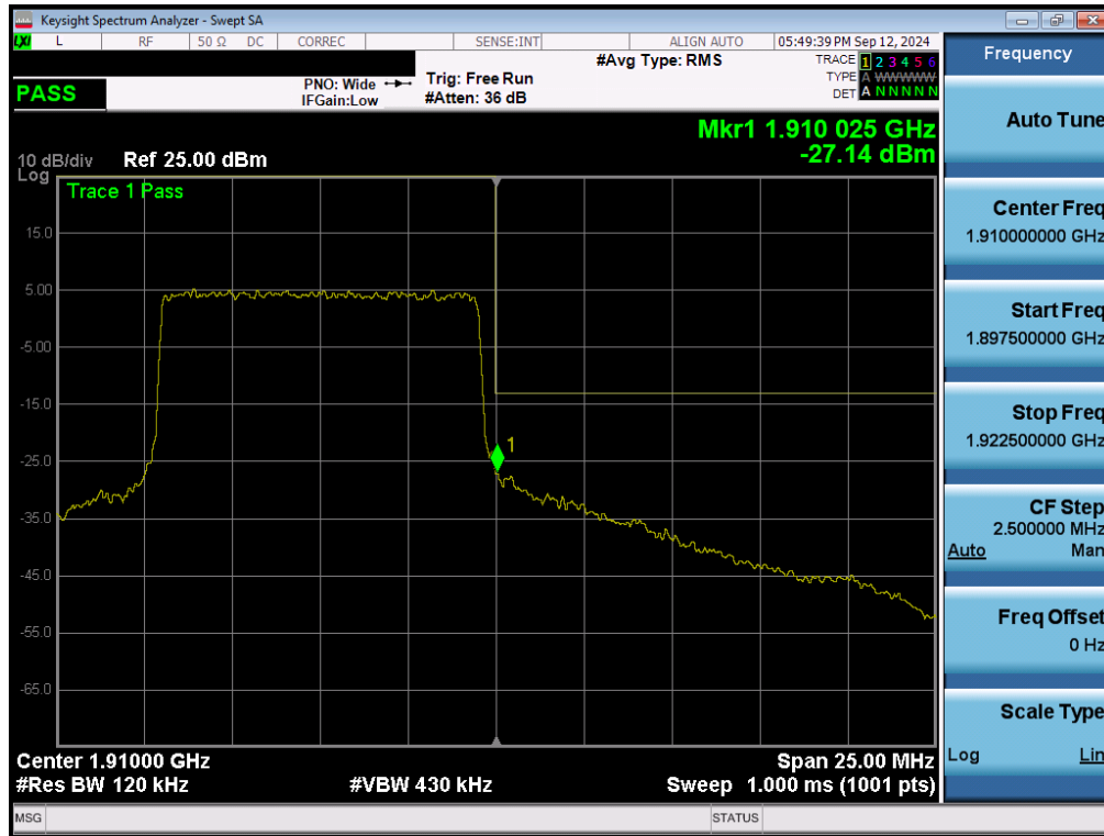
Plot 7-136. Upper Band Edge Plot (LTE Band 2 - 10MHz QPSK – Full RB - Ant1)
