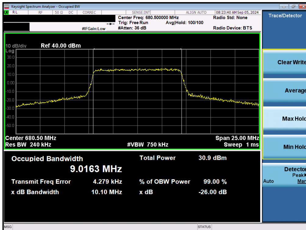
Plot 7-7. Occupied Bandwidth Plot (LTE Band 71 - 10MHz 16-QAM - Full RB – ANT1)
