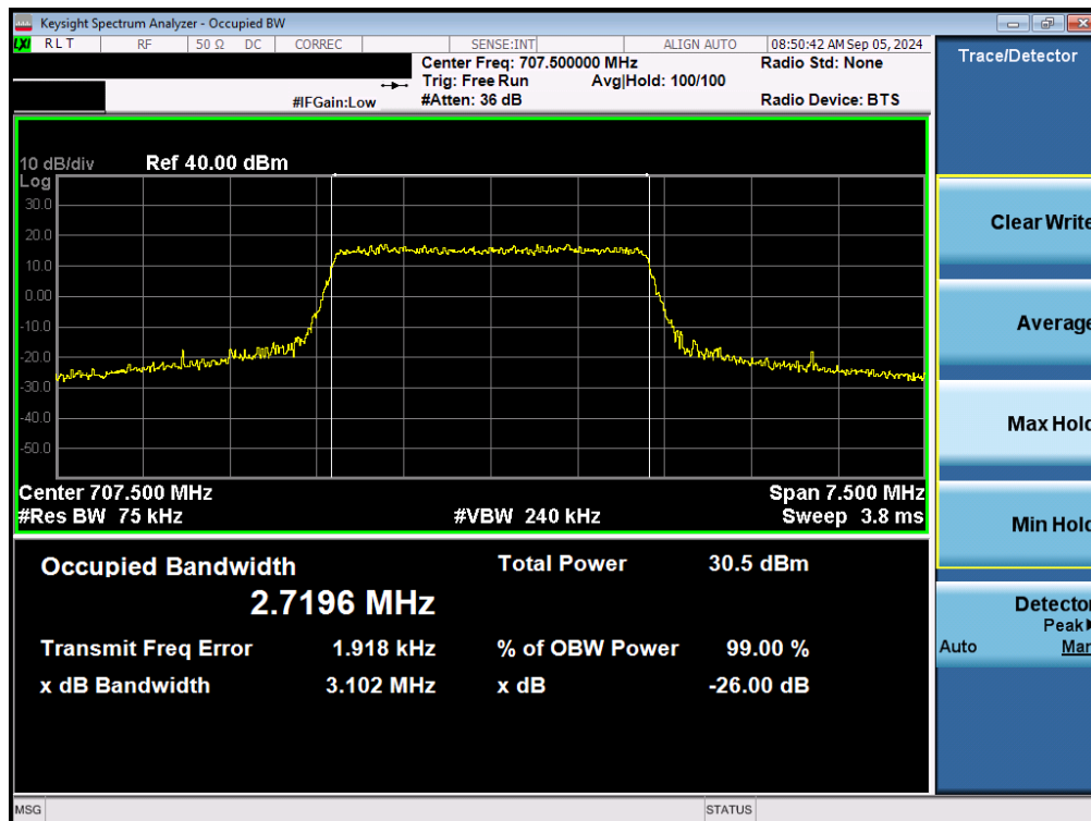
Plot 7-15. Occupied Bandwidth Plot (LTE Band 12 - 3MHz 16-QAM - Full RB – ANT1)
