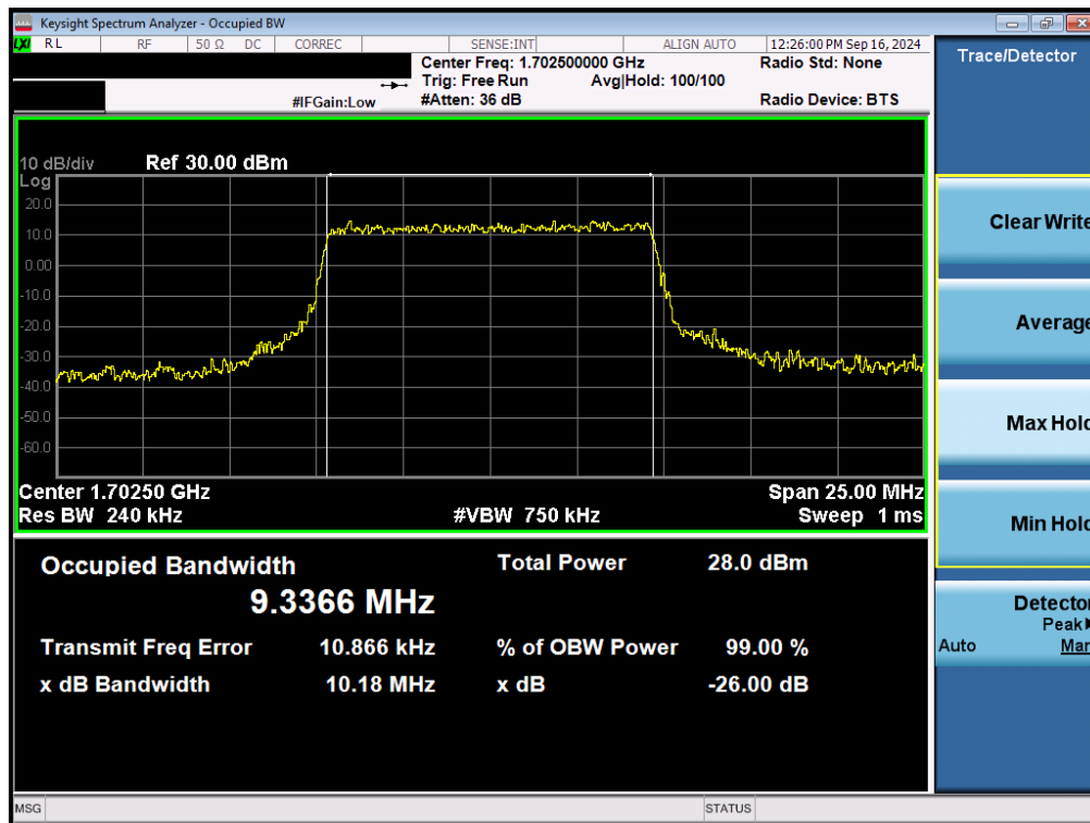
Plot 7-68. Occupied Bandwidth Plot (NR Band n70 - 10.0MHz CP-OFDM QPSK - Full RB – ANT1)
