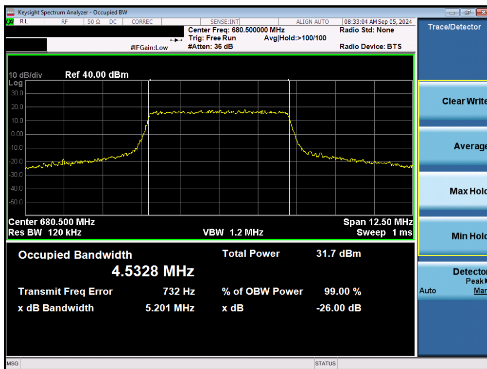
Plot 7-8. Occupied Bandwidth Plot (LTE Band 71 - 5MHz QPSK - Full RB – ANT1)
