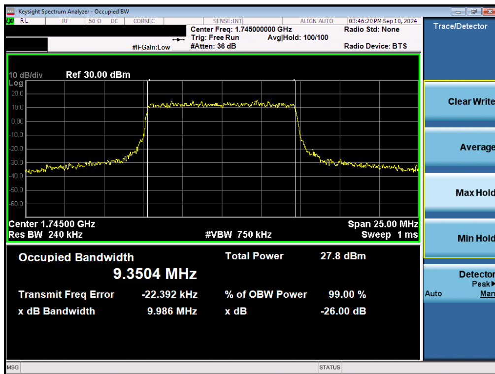
Plot 7-96. Occupied Bandwidth Plot (NR Band n66 - 10.0MHz CP-OFDM 16QAM - Full RB – ANT1)
