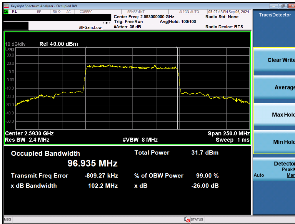
Plot 7-215. Occupied Bandwidth Plot (NR Band n41 - 100MHz \pi/2 BPSK - Full RB - Ant E)
