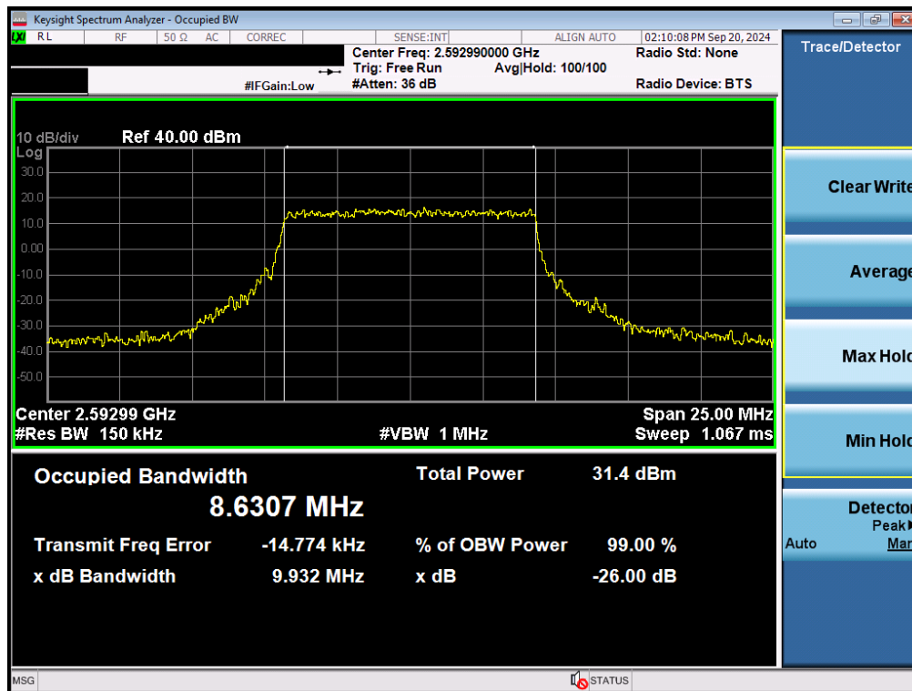
Plot 7-155. Occupied Bandwidth Plot (NR Band n41 - 10MHz 16-QAM - Full RB - Ant B)
