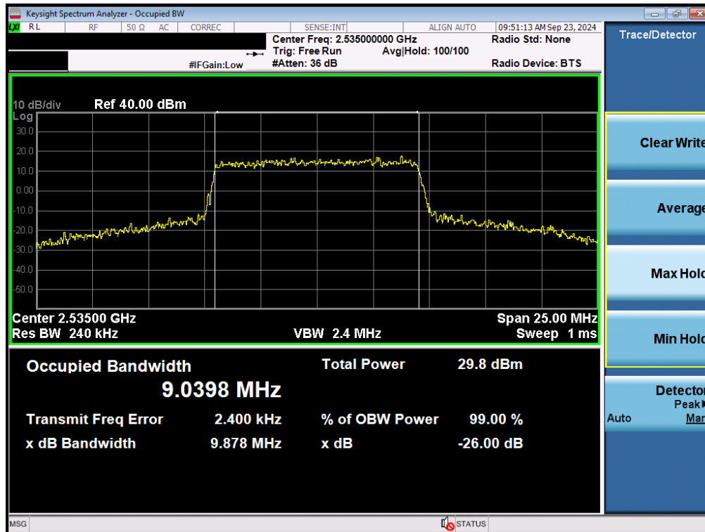
Plot 7-165. Occupied Bandwidth Plot (LTE Band 7 - 10MHz 16-QAM - Full RB - Ant B)
