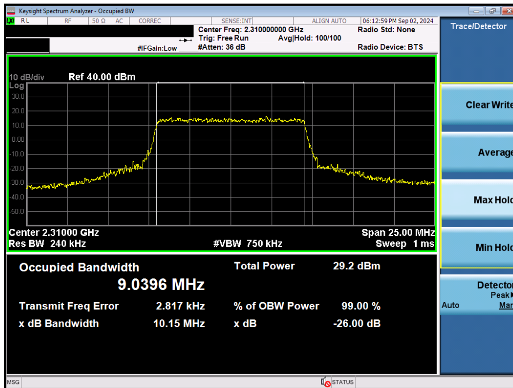
Plot 7-157. Occupied Bandwidth Plot (LTE Band 30 - 10MHz 16-QAM - Full RB - Ant F)
