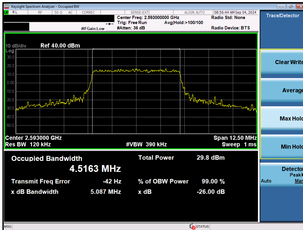
Plot 7-175. Occupied Bandwidth Plot (LTE Band 41(PCI)38 - 5MHz 16-QAM - Full RB - Ant B)
