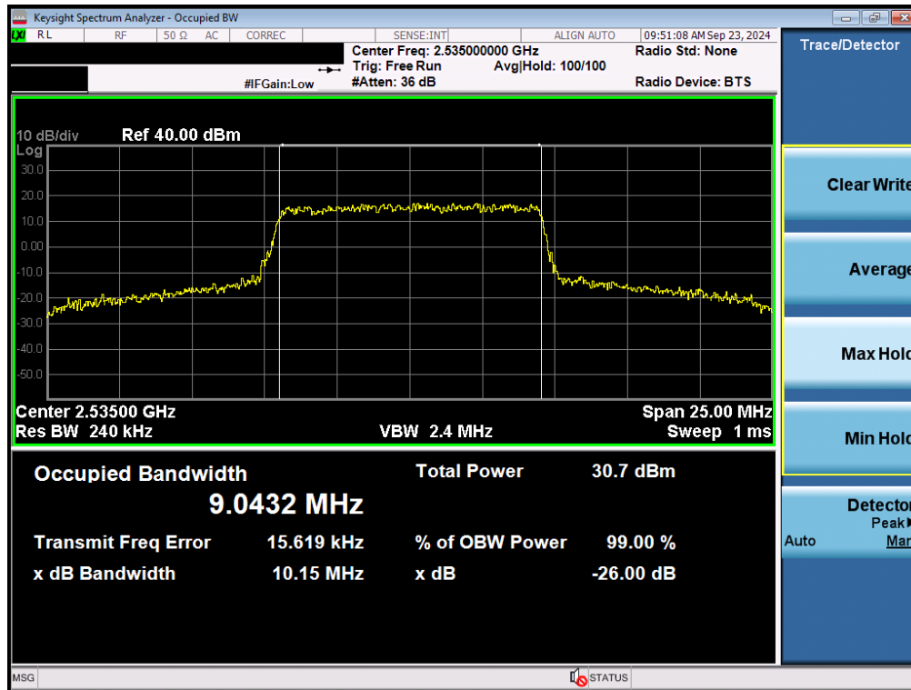
Plot 7-164. Occupied Bandwidth Plot (LTE Band 7 - 10MHz QPSK - Full RB - Ant B)
