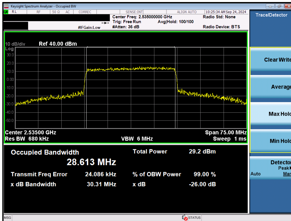
Plot 7-193. Occupied Bandwidth Plot (NR Band n7 - 30MHz 16-QAM - Full RB - Ant B)
