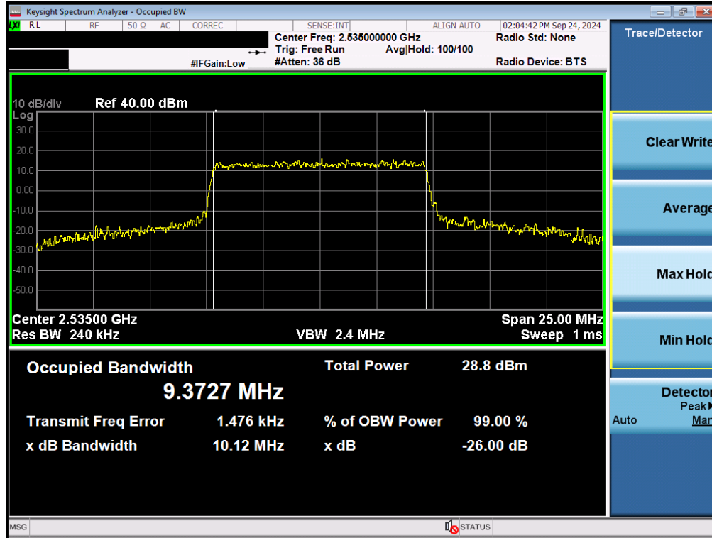
Plot 7-204. Occupied Bandwidth Plot (NR Band n7 - 10MHz QPSK - Full RB - Ant B)
