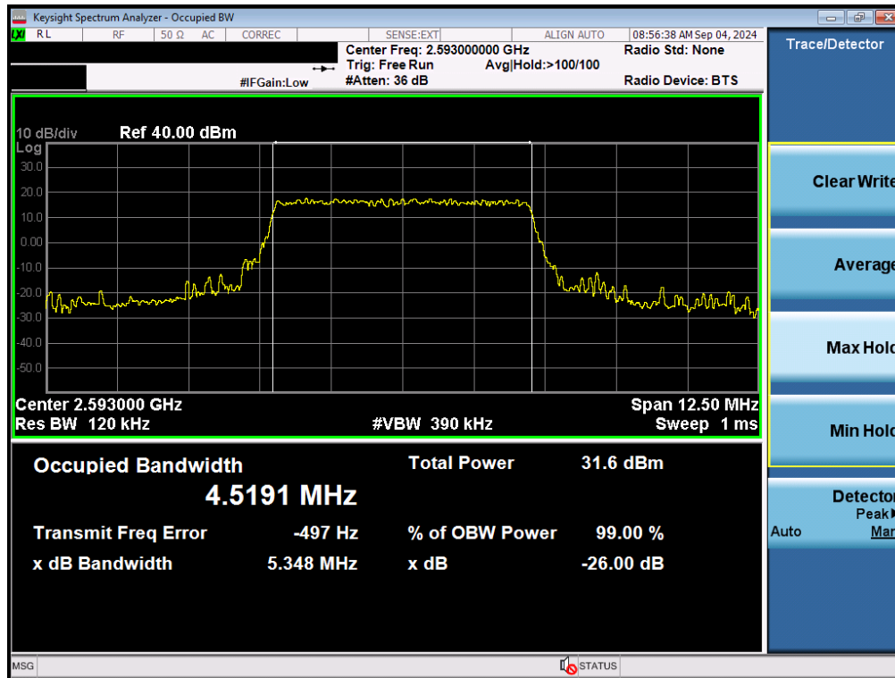
Plot 7-174. Occupied Bandwidth Plot (LTE Band 41(PCI)38 - 5MHz QPSK - Full RB - Ant B)
