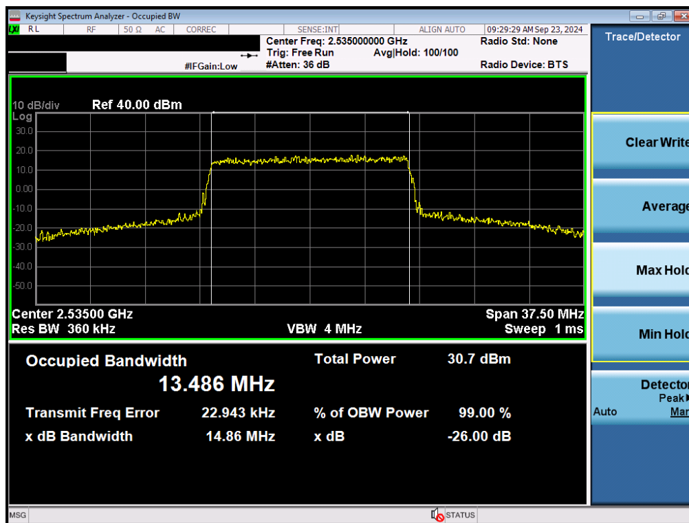
Plot 7-162. Occupied Bandwidth Plot (LTE Band 7 - 15MHz QPSK - Full RB - Ant B)
