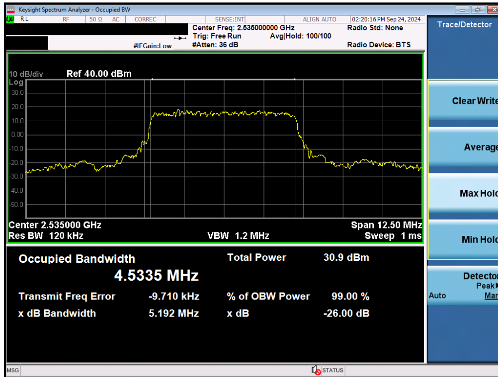
Plot 7-206. Occupied Bandwidth Plot (NR Band n7 - 5MHz \pi/2 BPSK - Full RB - Ant B)
