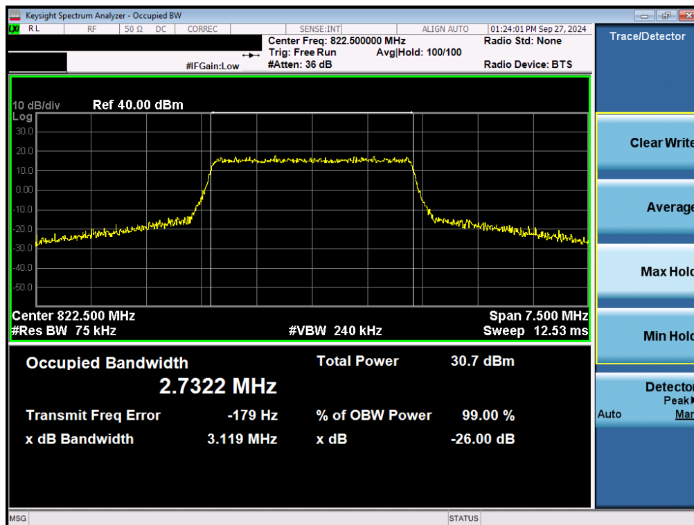
Plot 7-59. Occupied Bandwidth Plot (LTE Band 26 - 3MHz 16-QAM High Channel - Full RB)
