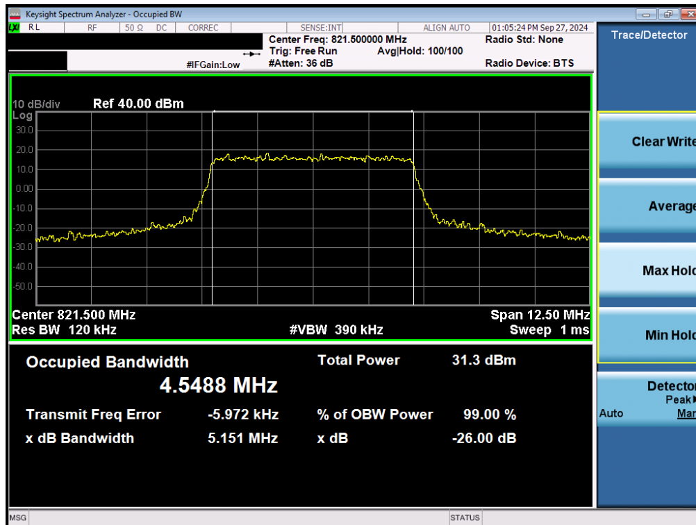
Plot 7-53. Occupied Bandwidth Plot (LTE Band 26 - 5MHz QPSK High Channel - Full RB)
