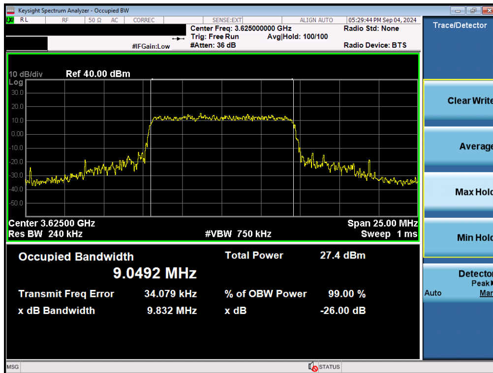
Plot 7-6. Occupied Bandwidth Plot (LTE Band 48 - 10MHz 16-QAM - Full RB Configuration - Ant F)
