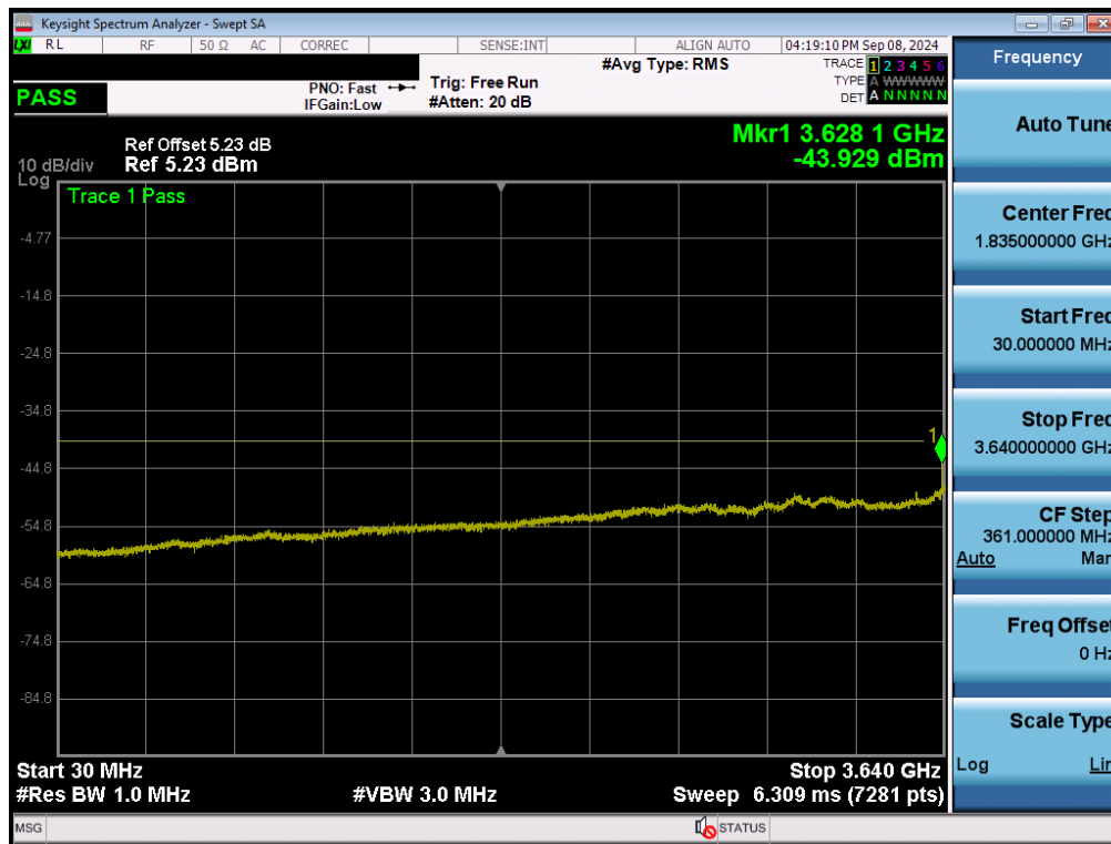
Plot 7-50. Conducted Spurious Plot (NR Band n48 - 40MHz QPSK - High Channel - Ant F)
