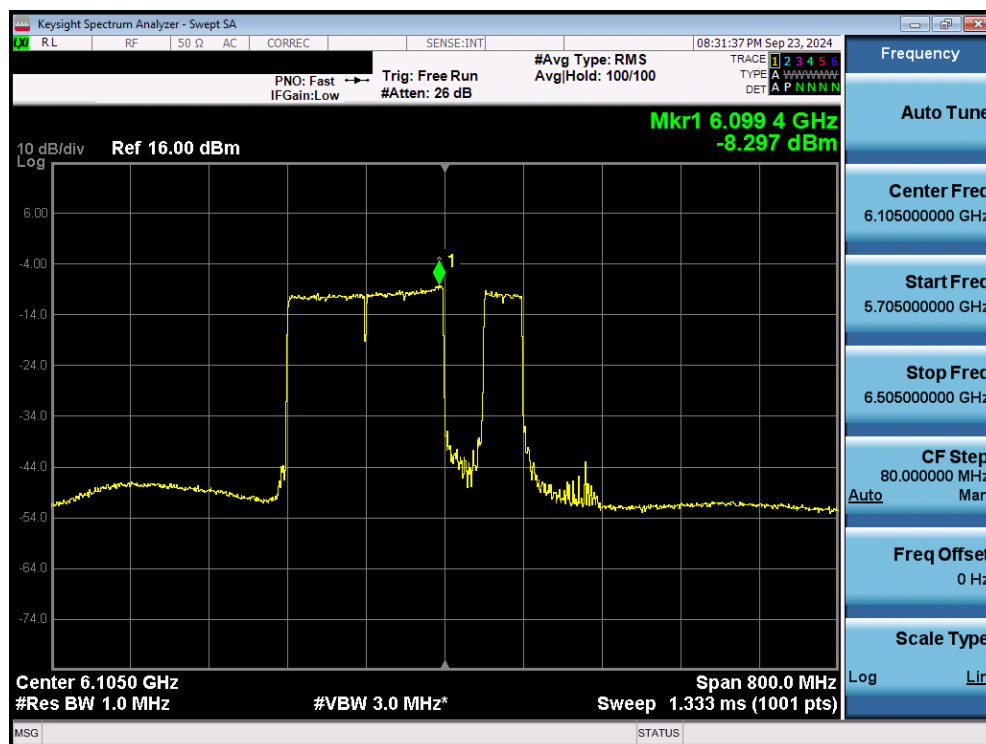
Plot 7-51. Power Spectral Density Plot MIMO ANT2 (320MHz 802.11be (UNII Band 5) – Ch. 31) VLP
