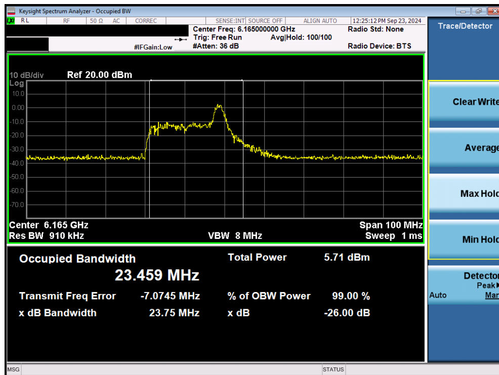
Plot 7-2. 26dB Bandwidth Plot MIMO ANT1 (40MHz 802.11ax/be (26 Tones) (UNII Band 5) – Ch. 43) - VLP
