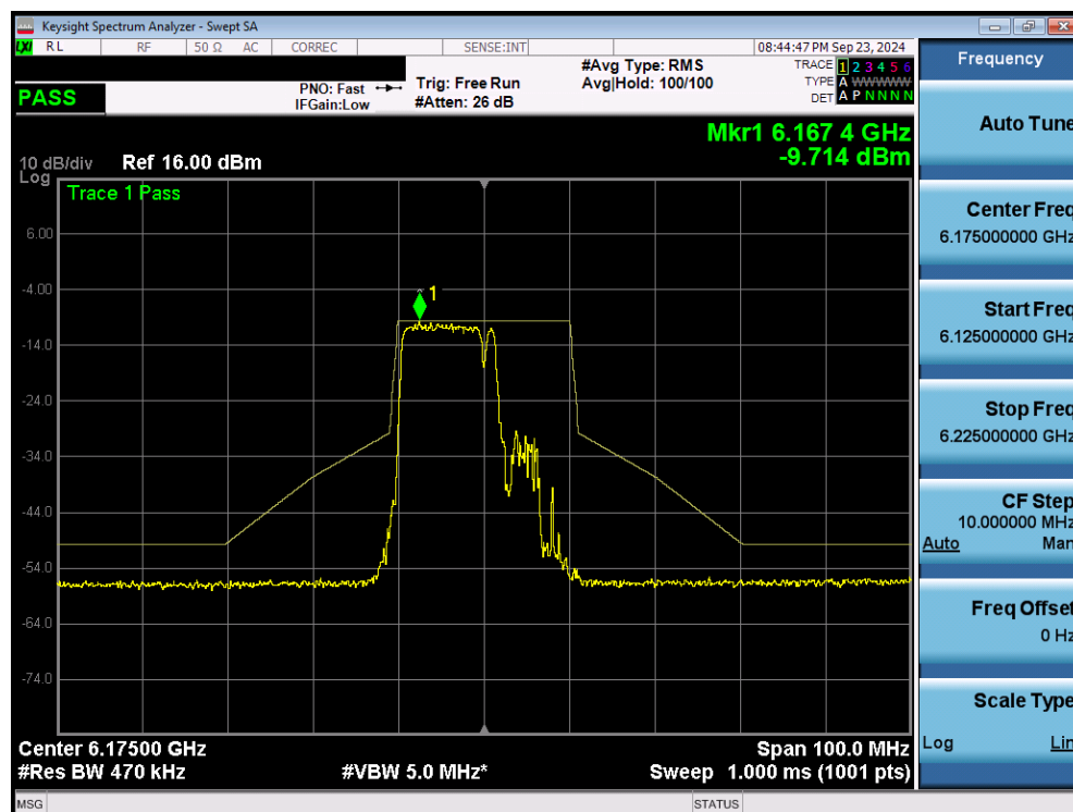
Plot 7-76. In Band Emissions Plot MIMO ANT2 (20MHz 802.11be (106+26 Tones) (UNII Band 5) – Ch. 45) - VLP
