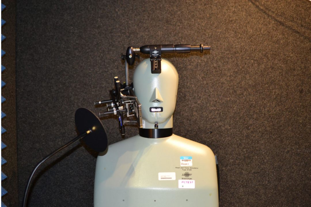
Figure 17-1 Test Setup for Wireless Device
