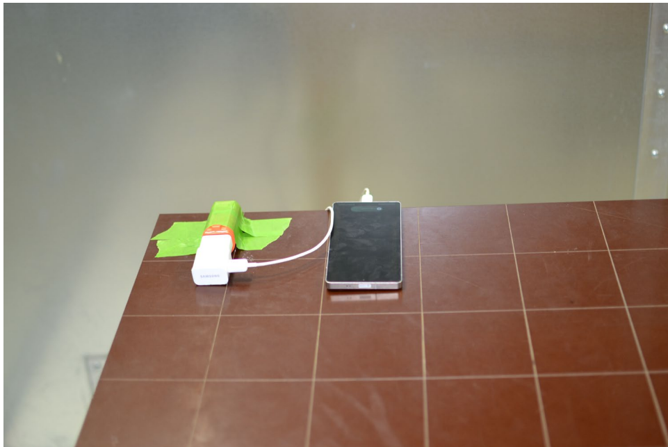
Figure 2. Test Setup – ACLC– <30MHz
