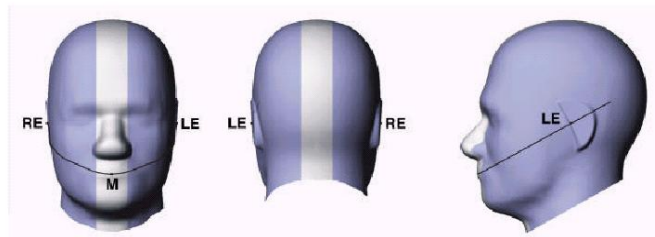
Figure 6-2 Front, back and side view of SAM Twin Phantom
