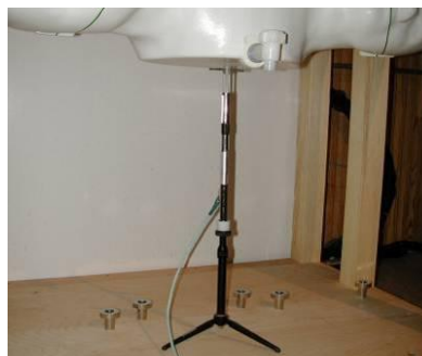
Figure 11-2 System Verification Setup Photo
