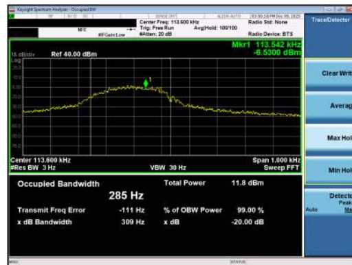
Figure 1-1 WPT Occupied Bandwidth
