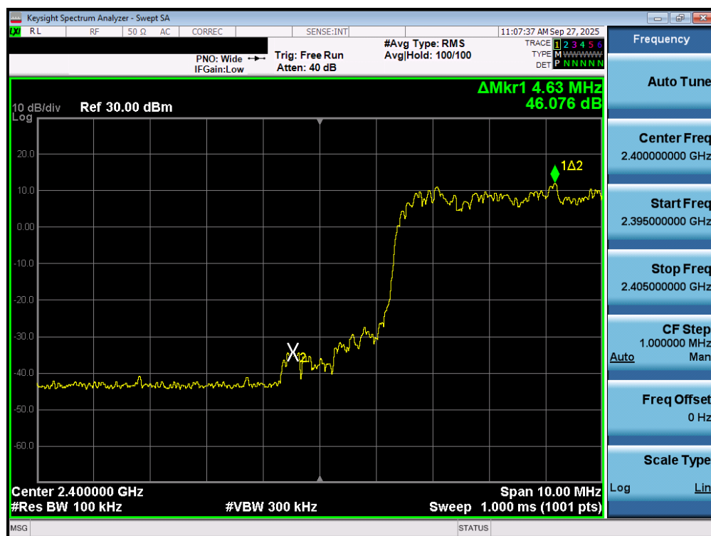
Plot 7-115. Band Edge Plot (Bluetooth with Hopping Enabled, 3 Mbps) – Ant 2
