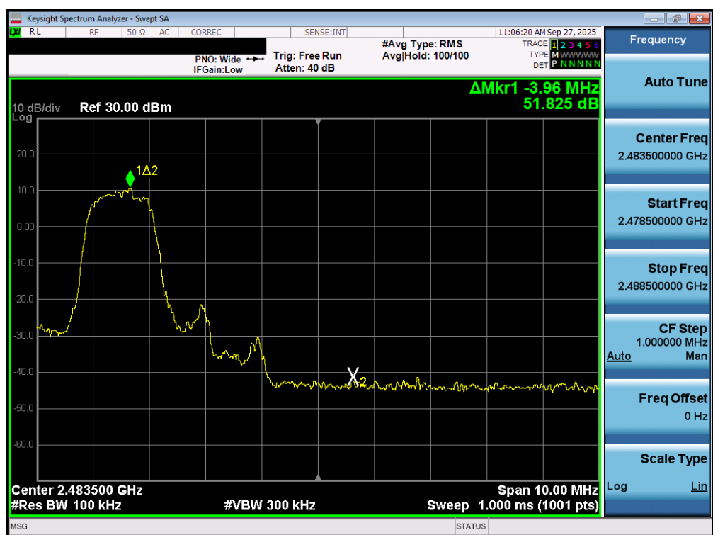
Plot 7-114. Band Edge Plot (Bluetooth with Hopping Disabled, 3 Mbps – Ch. 78) – Ant 2
