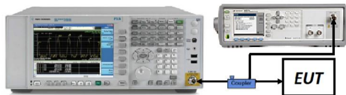
Figure 7-3. Test Instrument & Measurement Setup
