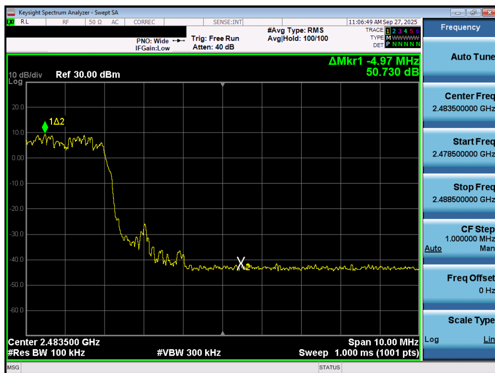
Plot 7-116. Band Edge Plot (Bluetooth with Hopping Enabled, 3 Mbps) – Ant 2
