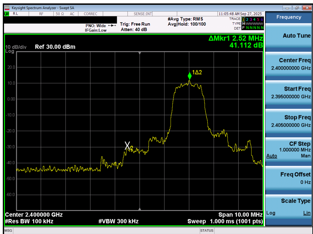
Plot 7-113. Band Edge Plot (Bluetooth with Hopping Disabled, 3 Mbps – Ch. 0) – Ant 2
