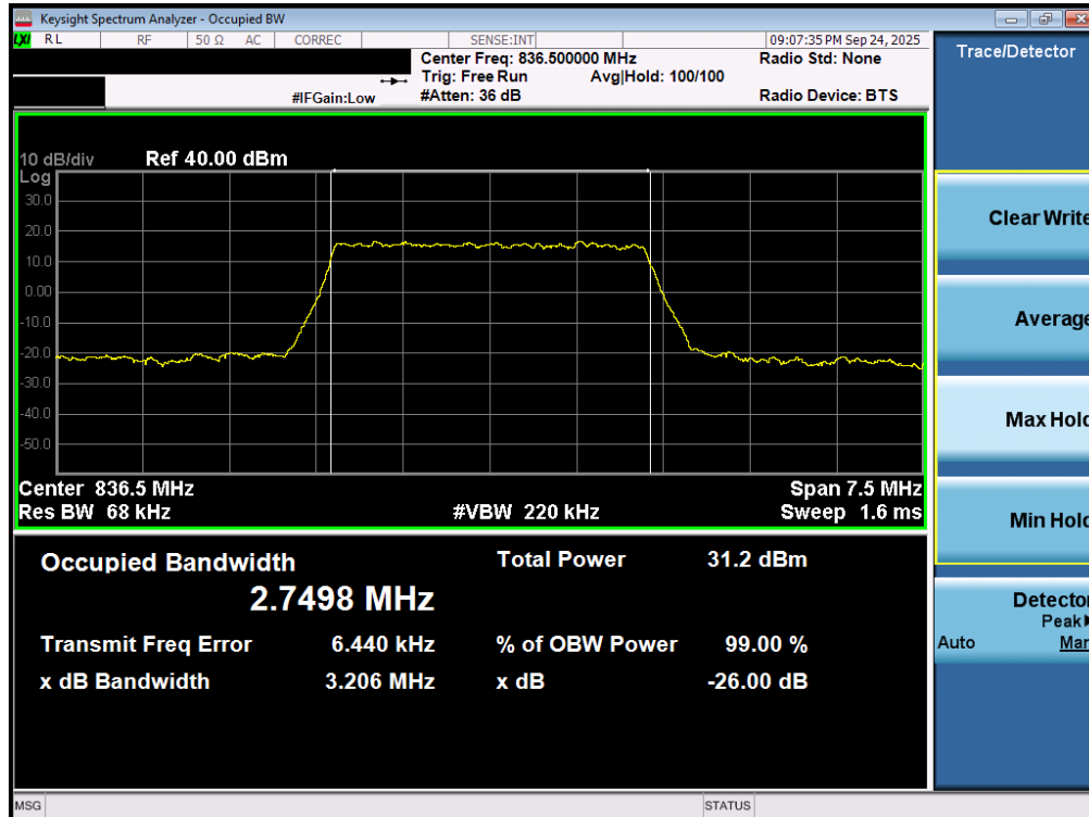
Plot 7-33. Occupied Bandwidth Plot (LTE Band 26/5 - 3MHz 16-QAM - Full RB - Ant2)
