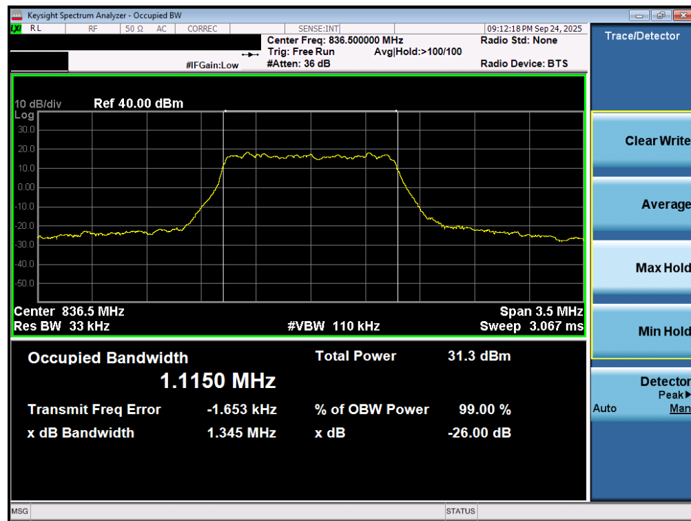
Plot 7-35. Occupied Bandwidth Plot (LTE Band 26/5 - 1.4MHz 16-QAM - Full RB - Ant2)
