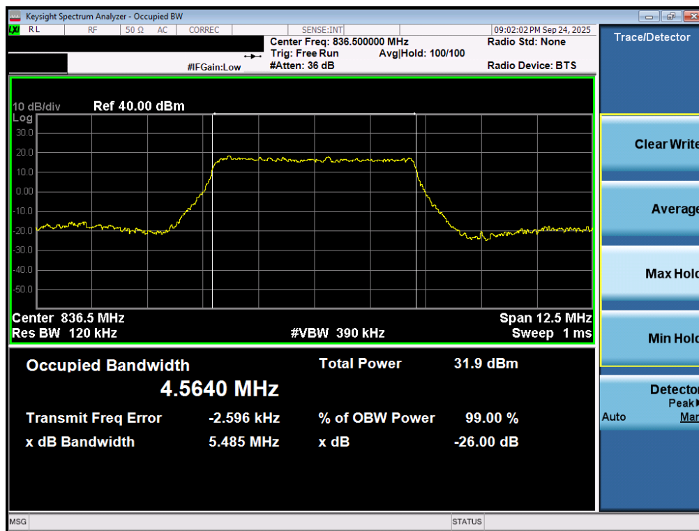
Plot 7-30. Occupied Bandwidth Plot (LTE Band 26/5 - 5MHz QPSK - Full RB - Ant2)
