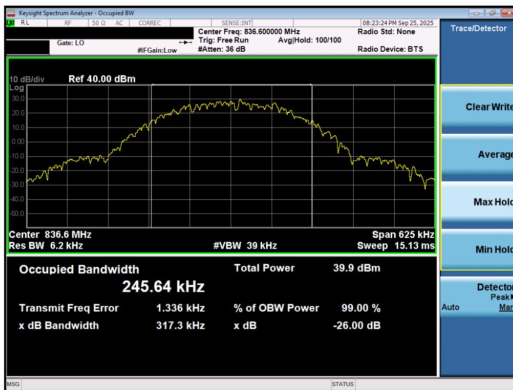
Plot 7-48. Occupied Bandwidth Plot (GPRS, Ch. 190 – Ant2)
