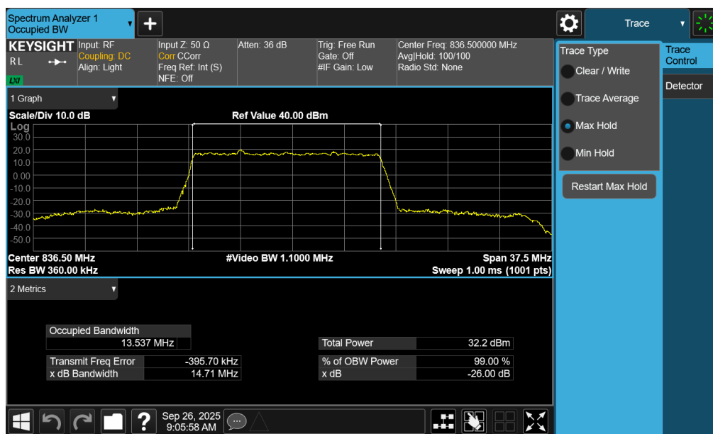
Plot 7-39. Occupied Bandwidth Plot (NR Band n26/5 - 15MHz \pi/2 BPSK - Full RB - Ant2)
