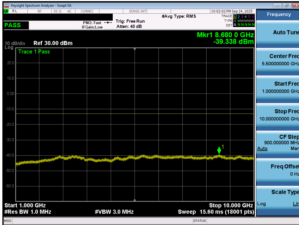
Plot 7-80. Conducted Spurious Plot (WCDMA Ch. 4132 – Ant1)
