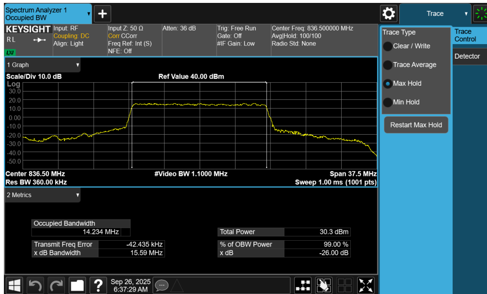
Plot 7-16. Occupied Bandwidth Plot (NR Band n26/5 - 15MHz 16-QAM - Full RB - Ant1)
