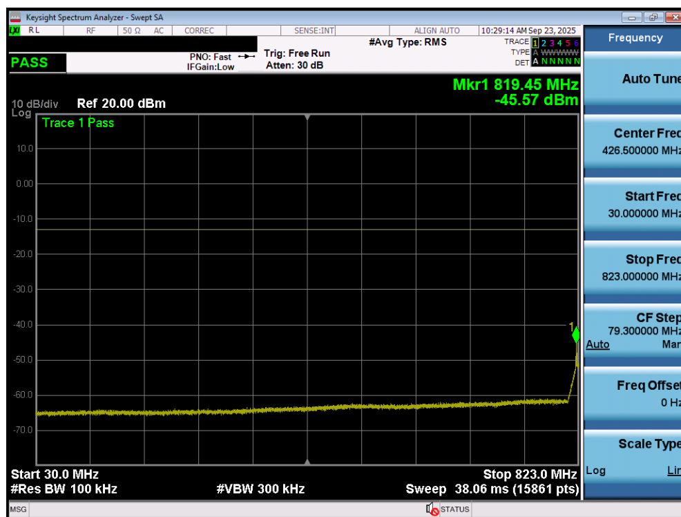
Plot 7-51. Conducted Spurious Plot (LTE Band 26/5 - 15MHz QPSK – 1 RB - Low Channel – Ant1)
