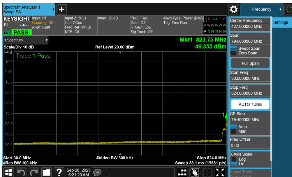
Plot 7-63. Conducted Spurious Plot (NR Band n26/5 - 20.0MHz - 1 RB - Mid Channel - Ant1)
