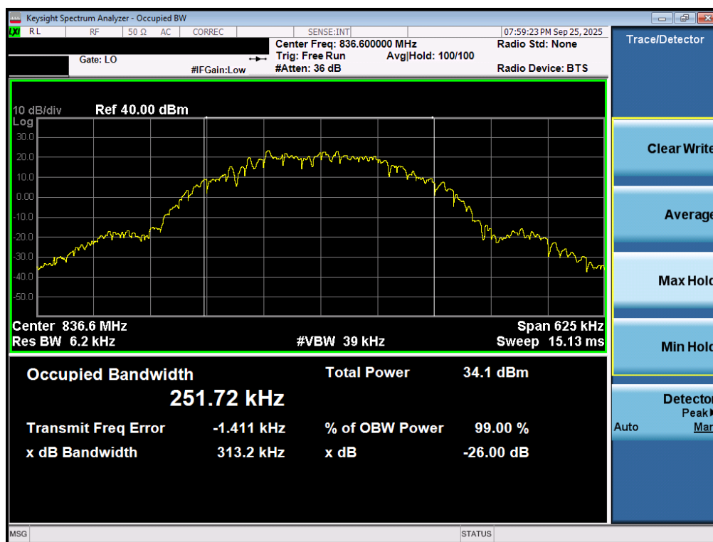
Plot 7-24. Occupied Bandwidth Plot (EDGE, Ch. 190 – Ant1)
