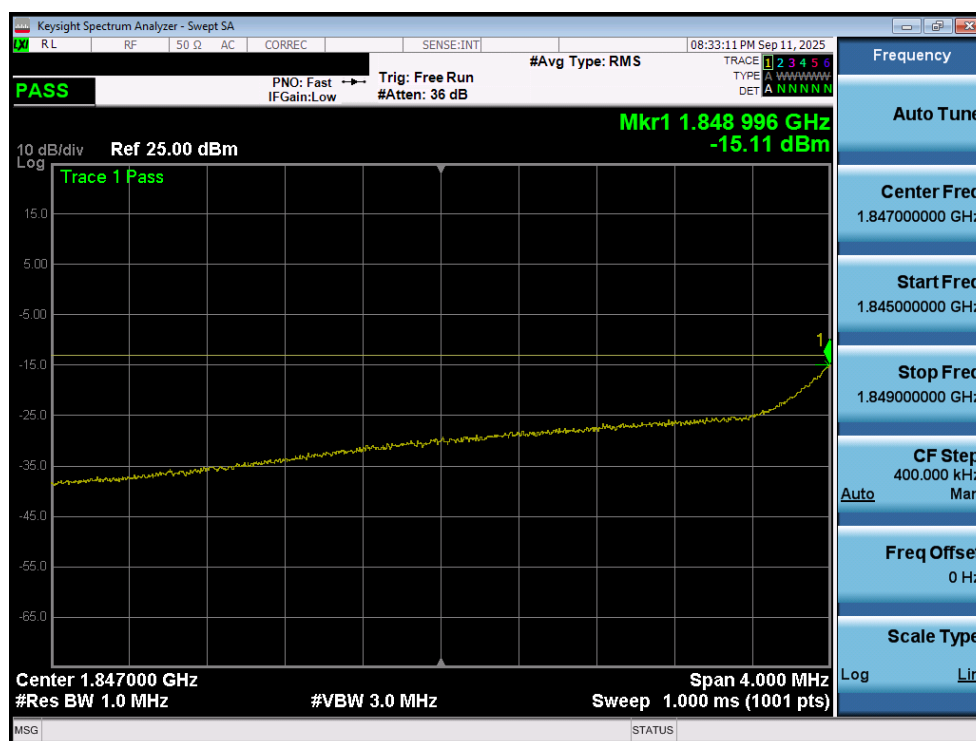
Plot 7-205. Extended Lower Band Edge Plot (WCDMA PCS – Ch. 9262 - Ant1)
