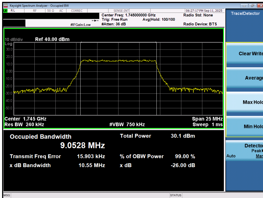
Plot 7-74. Occupied Bandwidth Plot (LTE Band 66/4 - 10MHz 16-QAM - Full RB - ANT2)
