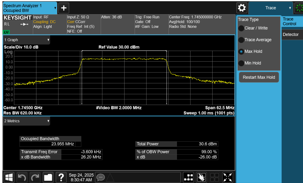
Plot 7-43. Occupied Bandwidth Plot (NR Band n66 - 25.0MHz CP-OFDM 16QAM - Full RB – ANT1)
