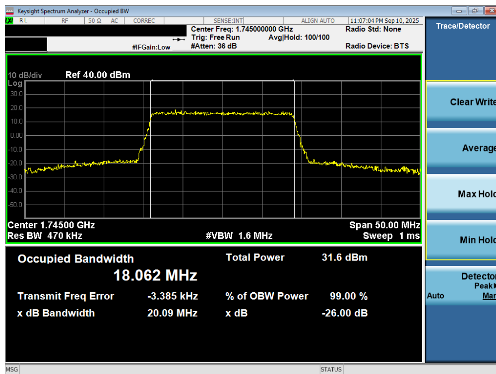
Plot 7-14. Occupied Bandwidth Plot (LTE Band 66/4 - 20MHz QPSK - Full RB - ANT1)
