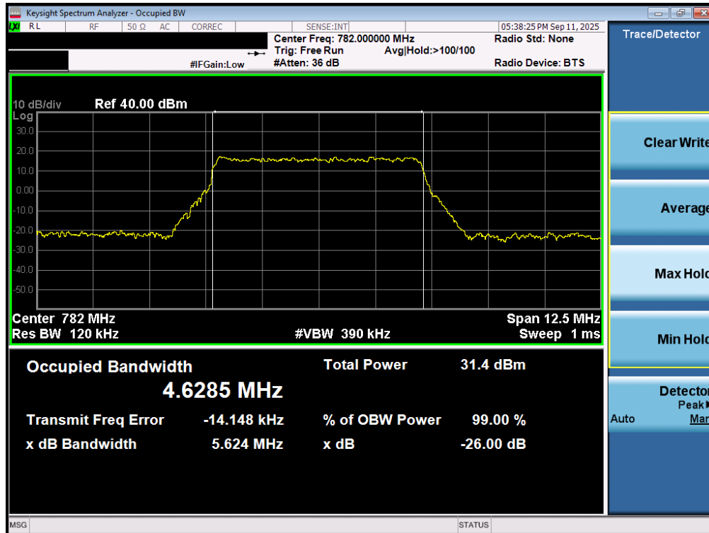
Plot 7-67. Occupied Bandwidth Plot (LTE Band 13 - 5MHz QPSK - Full RB – ANT2)
