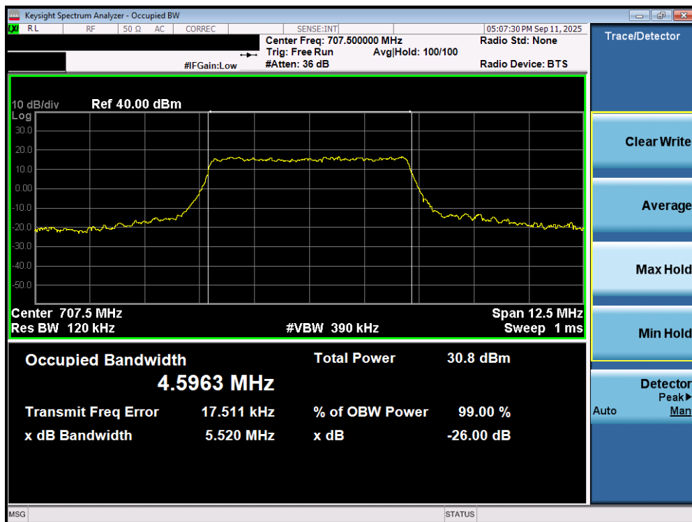
Plot 7-60. Occupied Bandwidth Plot (LTE Band 12/17 - 5MHz 16-QAM - Full RB - ANT2)
