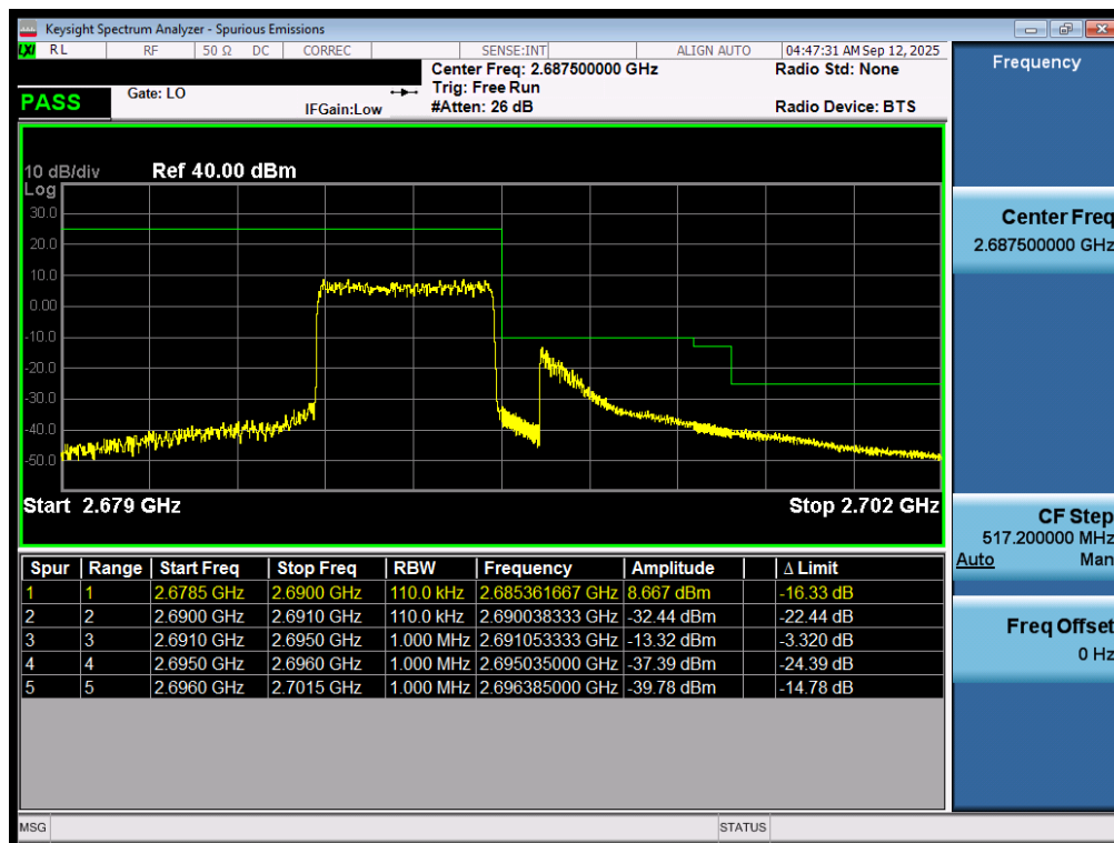
Plot 7-118. Upper ACP Plot (LTE Band 41(PC2) - 5MHz QPSK – Full RB - Ant1)
