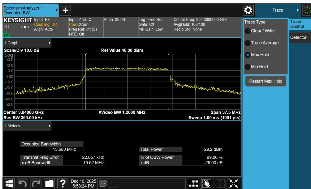
Plot 7-63. Occupied Bandwidth Plot (NR Band n77 - 15MHz 16-QAM - Full RB - Ant1 - C-Band)
