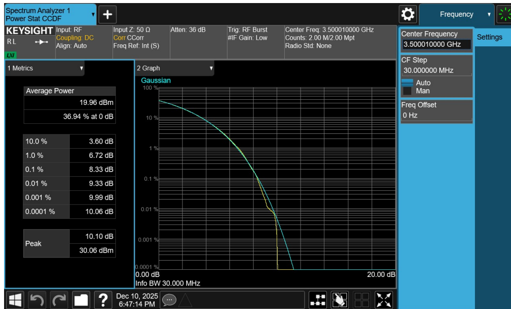
Plot 7-90. PAR Plot (NR Band n77 - 30MHz CP-OFDM 256-QAM - Full RB - Ant1 – DoD-Band)
