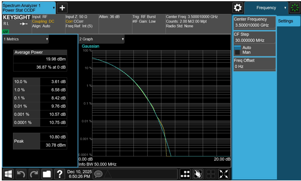
Plot 7-88. PAR Plot (NR Band n77 - 50MHz CP-OFDM 256-QAM - Full RB - Ant1 – DoD-Band)
