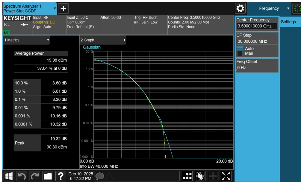
Plot 7-89. PAR Plot (NR Band n77 - 40MHz CP-OFDM 256-QAM - Full RB - Ant1 – DoD-Band)
