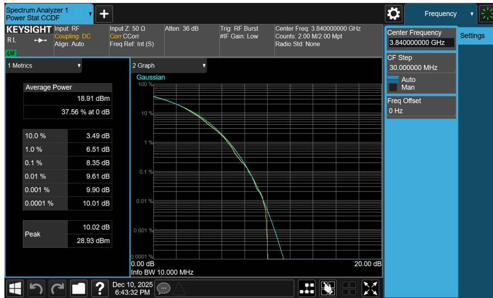
Plot 7-104. PAR Plot (NR Band n77 - 10MHz CP-OFDM 256-QAM - Full RB - Ant1 – C-Band)
