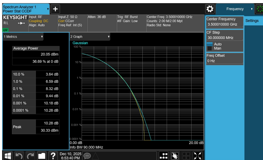
Plot 7-84. PAR Plot (NR Band n77 - 90MHz CP-OFDM 256-QAM - Full RB - Ant1 – DoD-Band)
