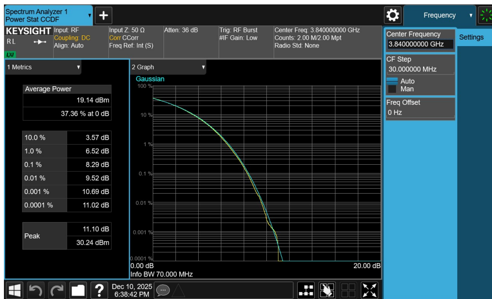
Plot 7-97. PAR Plot (NR Band n77 - 70MHz CP-OFDM 256-QAM - Full RB - Ant1 – C-Band)
