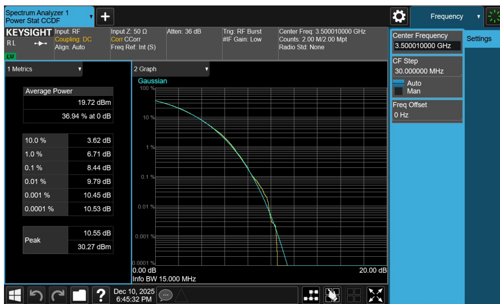
Plot 7-92. PAR Plot (NR Band n77 - 15MHz CP-OFDM 256-QAM - Full RB - Ant1 – DoD-Band)
