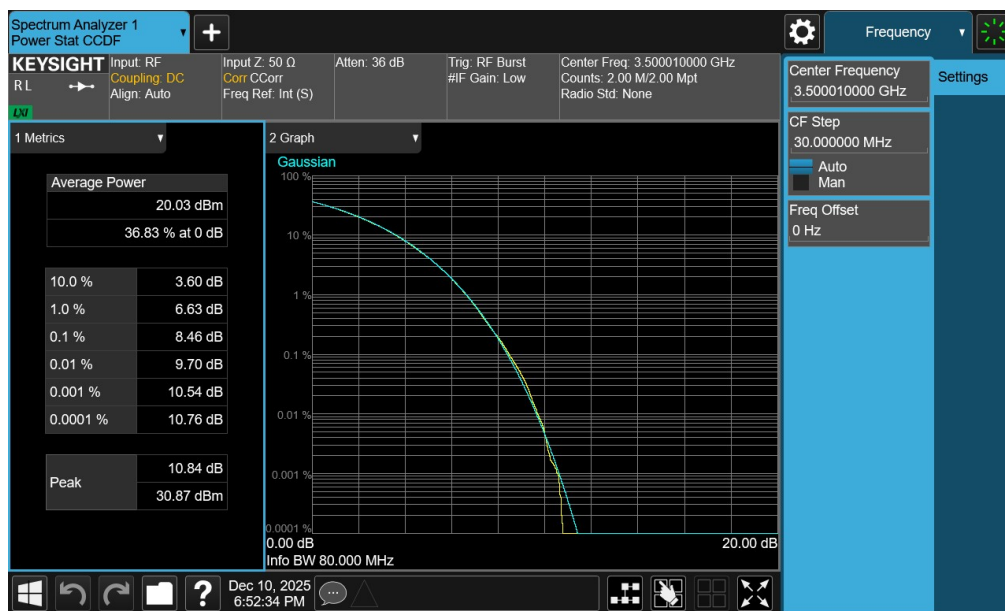
Plot 7-85. PAR Plot (NR Band n77 - 80MHz CP-OFDM 256-QAM - Full RB - Ant1 – DoD-Band)
