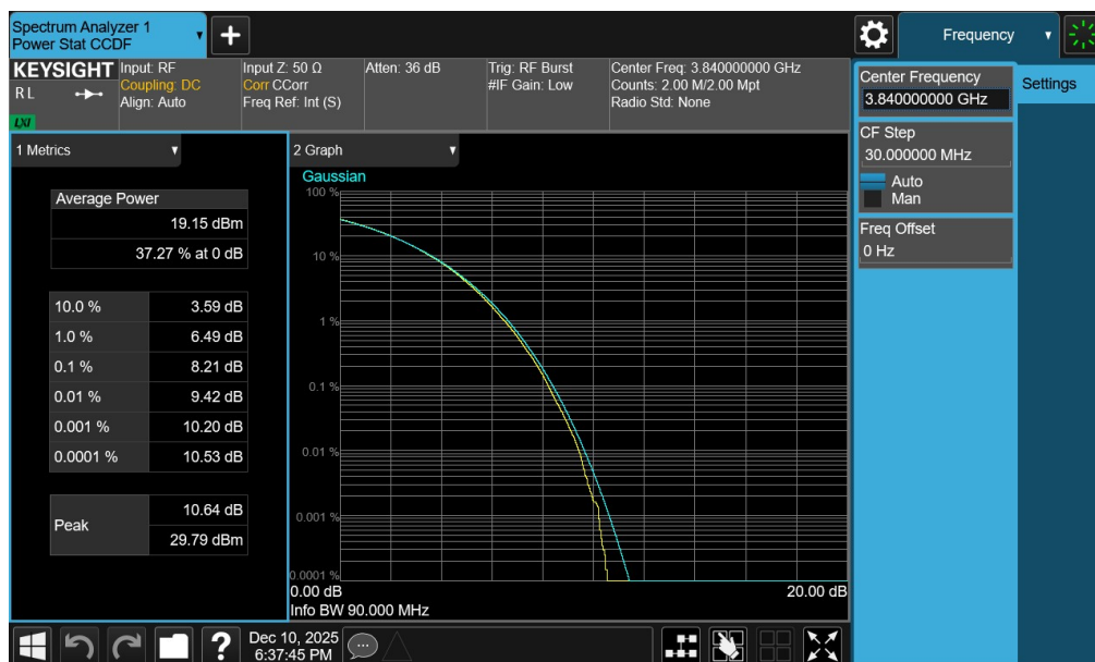
Plot 7-95. PAR Plot (NR Band n77 - 90MHz CP-OFDM 256-QAM - Full RB - Ant1 – C-Band)
