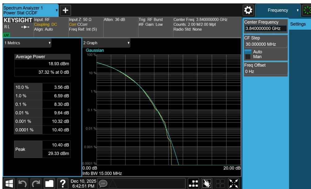
Plot 7-103. PAR Plot (NR Band n77 - 15MHz CP-OFDM 256-QAM - Full RB - Ant1 - C-Band)
