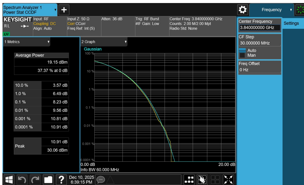
Plot 7-98. PAR Plot (NR Band n77 - 60MHz CP-OFDM 256-QAM - Full RB - Ant1 – C-Band)
