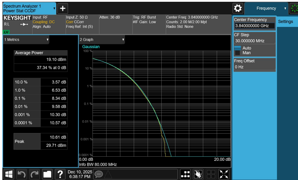
Plot 7-96. PAR Plot (NR Band n77 - 80MHz CP-OFDM 256-QAM - Full RB - Ant1 – C-Band)
