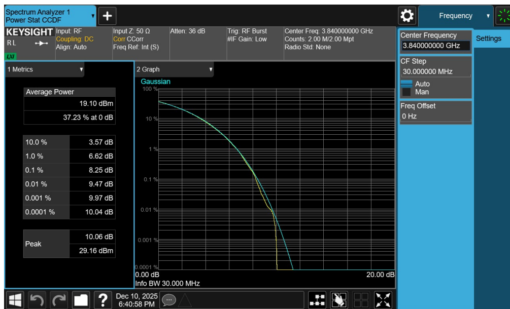
Plot 7-101. PAR Plot (NR Band n77 - 30MHz CP-OFDM 256-QAM - Full RB - Ant1 - C-Band)
