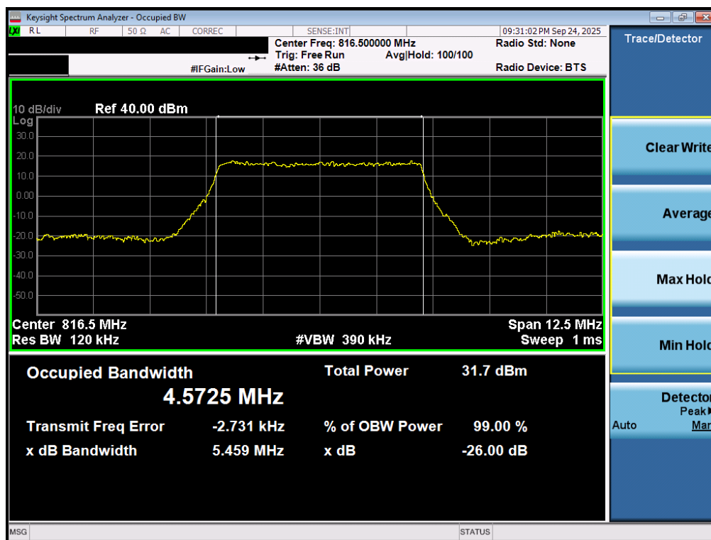
Plot 7-36. Occupied Bandwidth Plot (LTE Band 26 - 5MHz QPSK Low Channel- Full RB)
