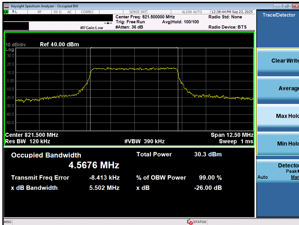
Plot 7-8. Occupied Bandwidth Plot (LTE Band 26 - 5MHz 16-QAM High Channel - Full RB)
