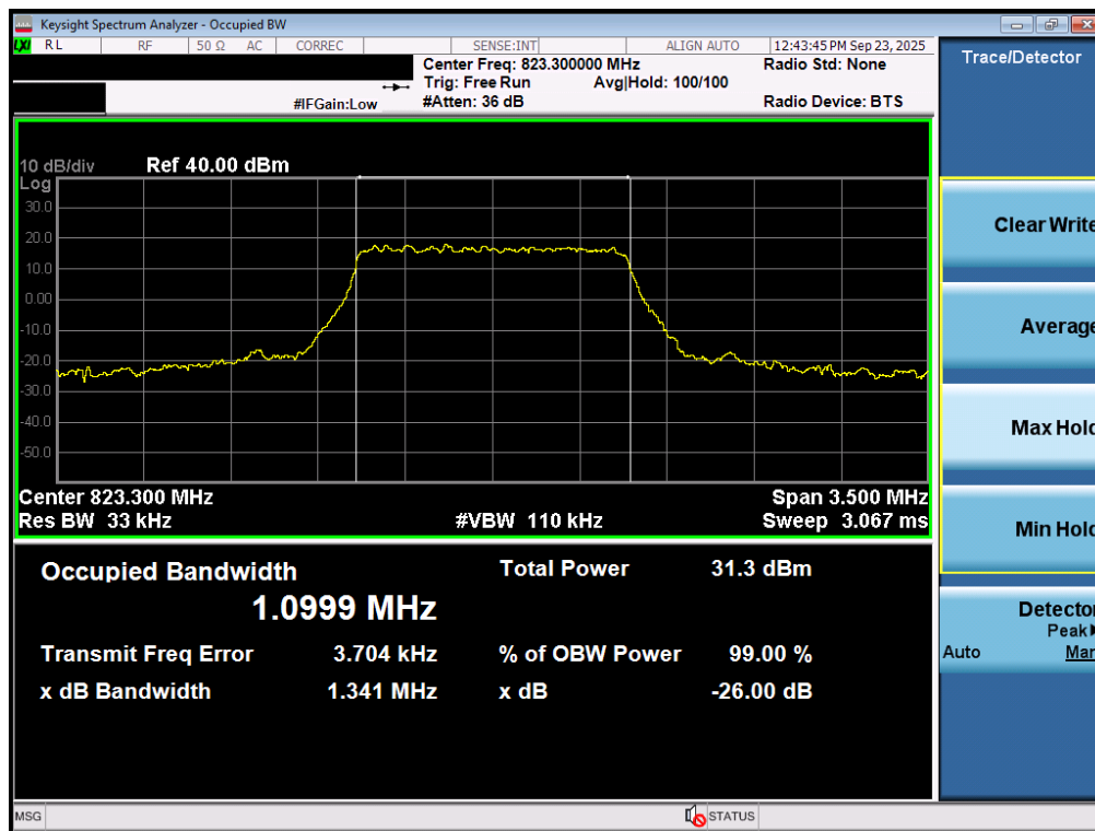
Plot 7-14. Occupied Bandwidth Plot (LTE Band 26 – 1.4MHz QPSK High Channel - Full RB)
