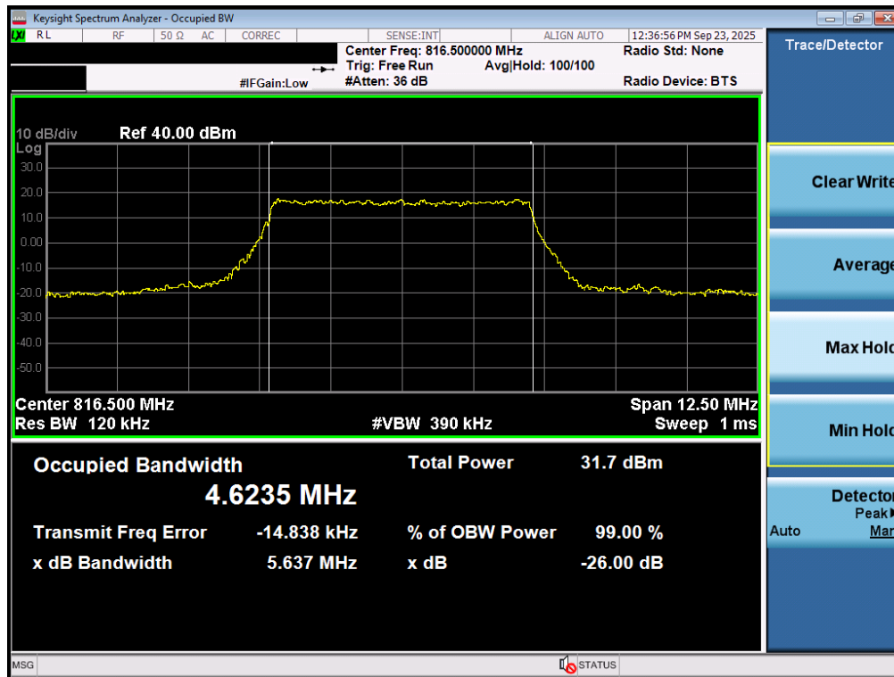
Plot 7-5. Occupied Bandwidth Plot (LTE Band 26 - 5MHz QPSK Low Channel- Full RB)
