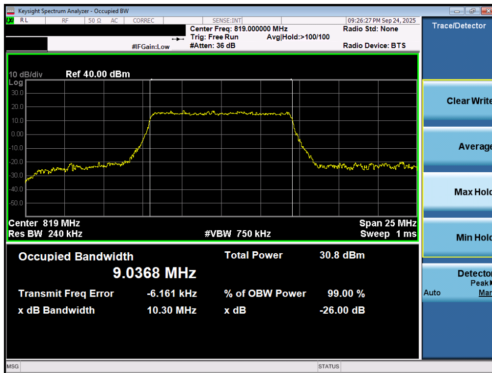
Plot 7-35. Occupied Bandwidth Plot (LTE Band 26 - 10MHz 16-QAM - Full RB)
