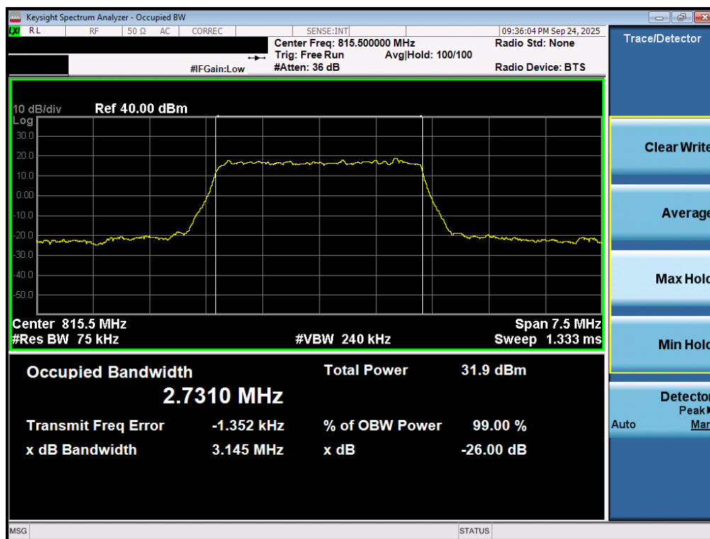
Plot 7-40. Occupied Bandwidth Plot (LTE Band 26 - 3MHz QPSK Low Channel- Full RB)
