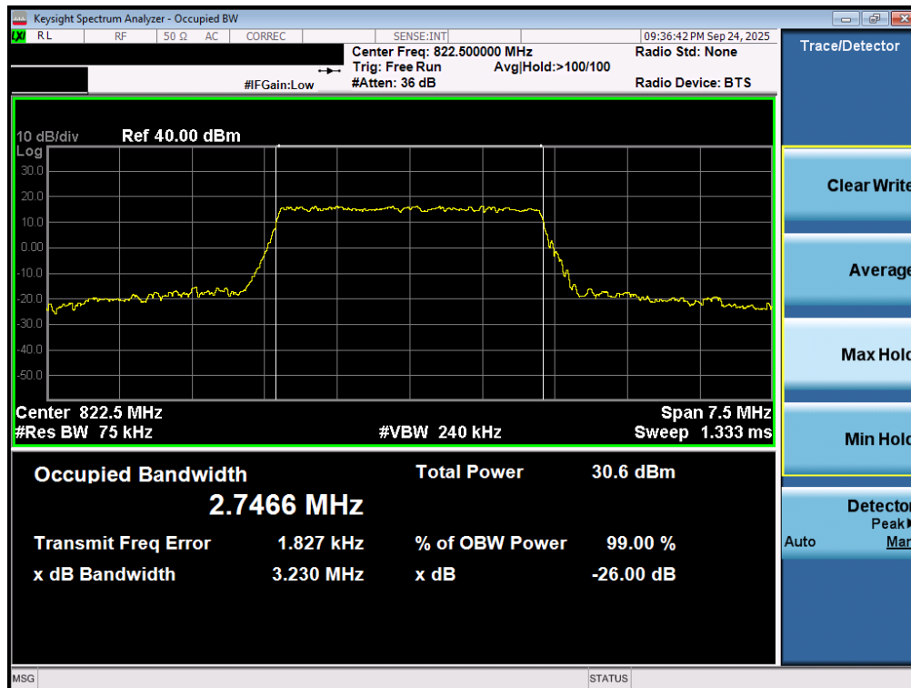
Plot 7-43. Occupied Bandwidth Plot (LTE Band 26 - 3MHz 16-QAM High Channel - Full RB)
