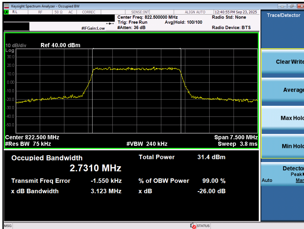
Plot 7-10. Occupied Bandwidth Plot (LTE Band 26 - 3MHz QPSK High Channel - Full RB)
