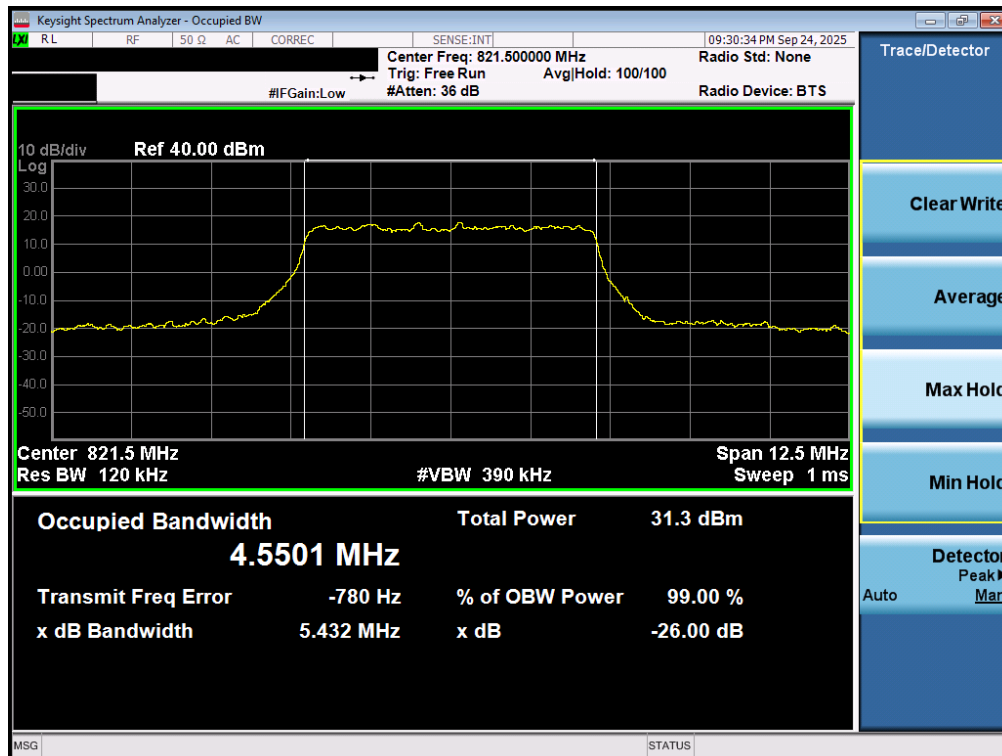
Plot 7-39. Occupied Bandwidth Plot (LTE Band 26 - 5MHz 16-QAM High Channel - Full RB)
