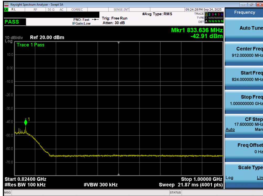
Plot 7-70. Conducted Spurious Plot (LTE Band 26 - 15MHz QPSK - RB Size 1, RB Offset 37)
