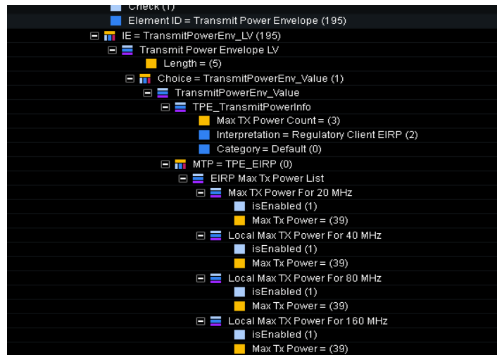
Figure 7-8. Callbox Power Authorization – 19.50dBm
