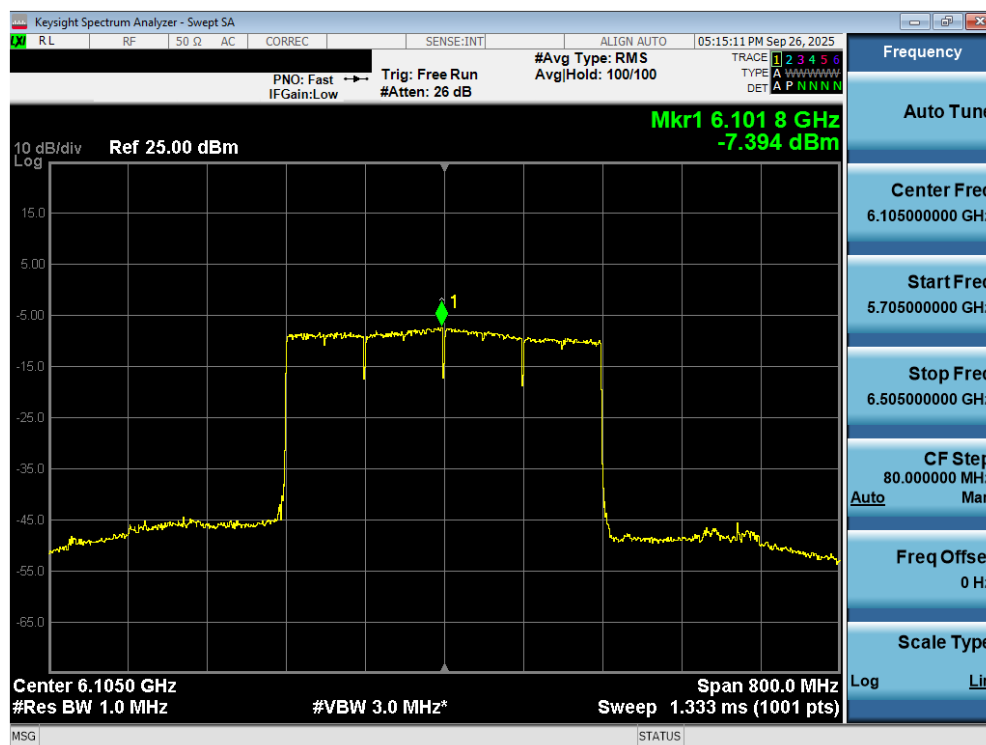
Plot 7-112. Power Spectral Density Plot MIMO ANT2 (320MHz 802.11be (Full Tones) (UNII Band 5) – Ch. 31) - SP
