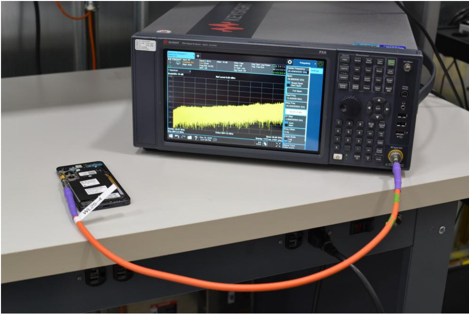
Figure 10. Conducted Test Setup – FTM mode
