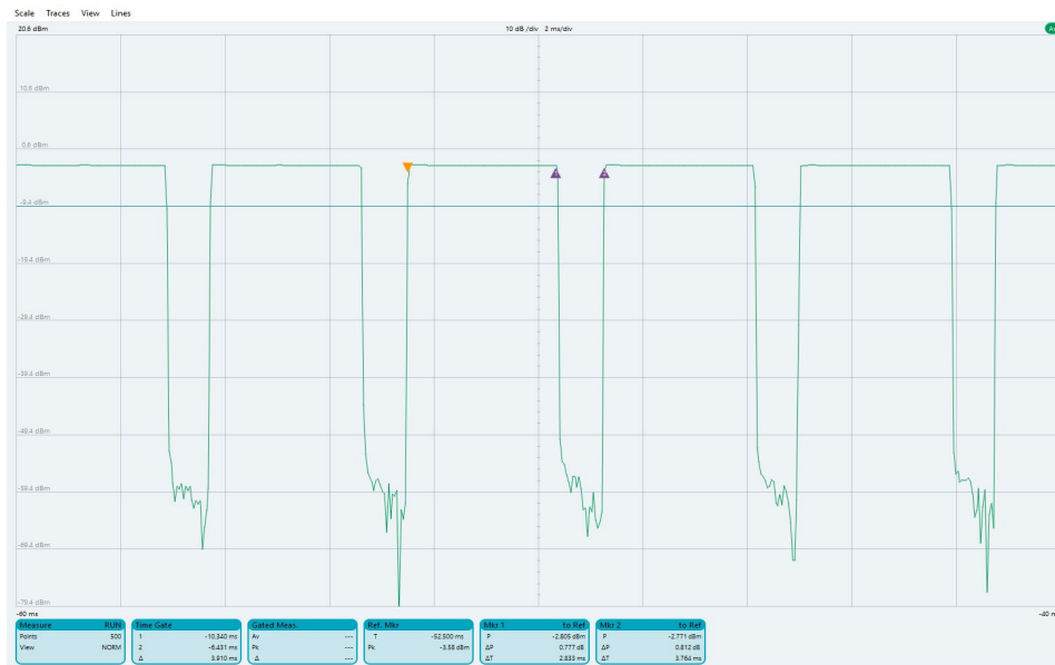
Figure 2-5 2.4 GHz Bluetooth LE MIMO (G&I) Duty Cycle Plot and Calculation
