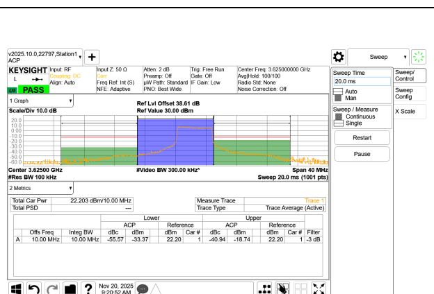
LTE B48 5MHz QPSK Mid Channel RB25-0 (3627.5 MHz)
