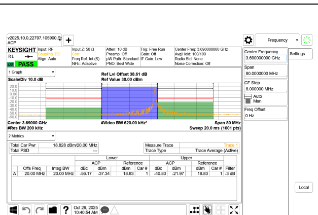
LTE B48 15MHz QPSK High Channel RB1-74
