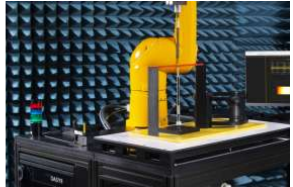
Figure 4.2 DASY8 with Module HAC
