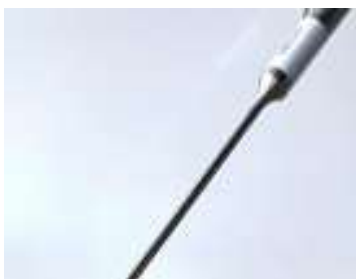
Figure 4.1 AM1DV3 Audio Magnetic Field Probe
