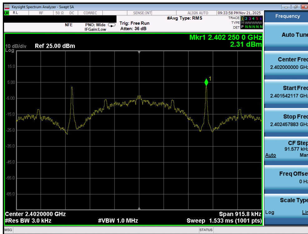
Plot 7-85. Power Spectral Density Plot (Bluetooth (LE), 125kbps – Ch. 37) – Ant 2
