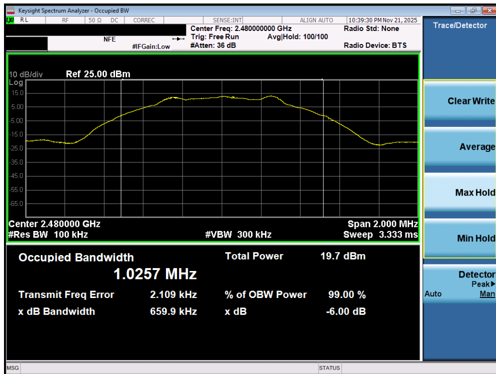
Plot 7-33. 6dB Bandwidth Plot (Bluetooth (LE), 1Mbps – Ch. 39) – Dual Ant 2
