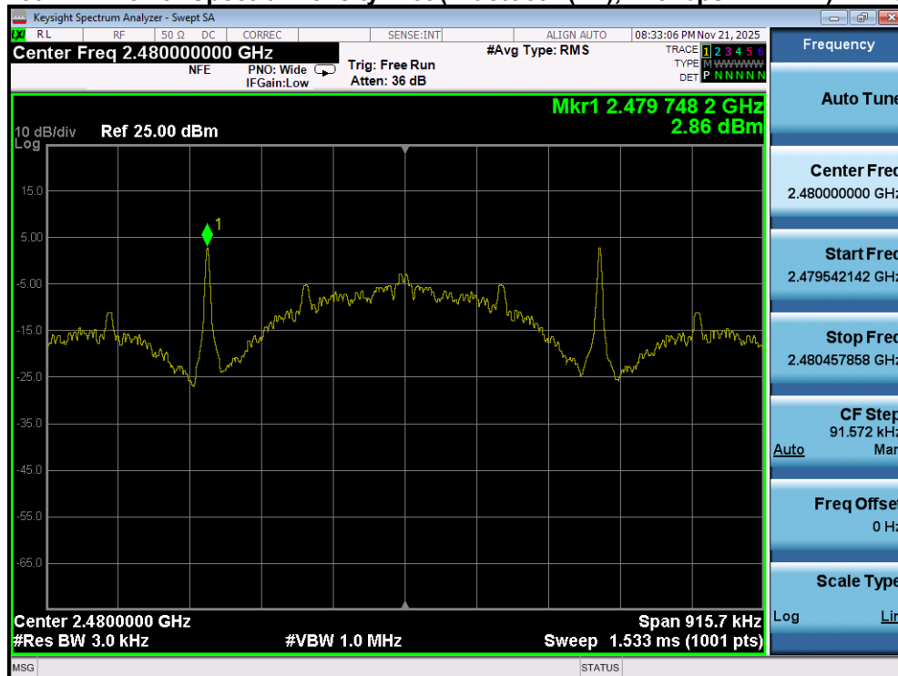
Plot 7-75. Power Spectral Density Plot (Bluetooth (LE), 125kbps – Ch. 39) – Ant 1
