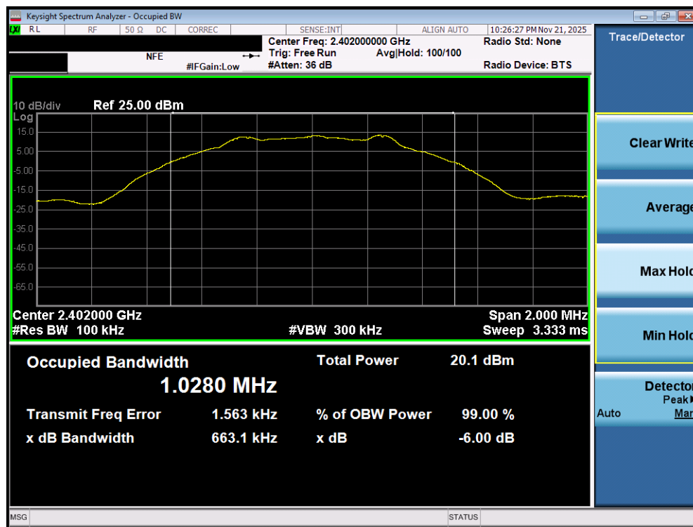
Plot 7-31. 6dB Bandwidth Plot (Bluetooth (LE), 1Mbps – Ch. 37) – Dual Ant 2
