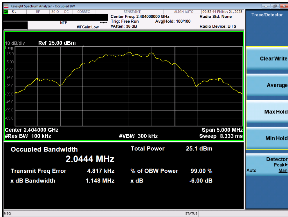
Plot 7-22. 6dB Bandwidth Plot (Bluetooth (LE), 2Mbps – Ch. 0) – Ant 2
