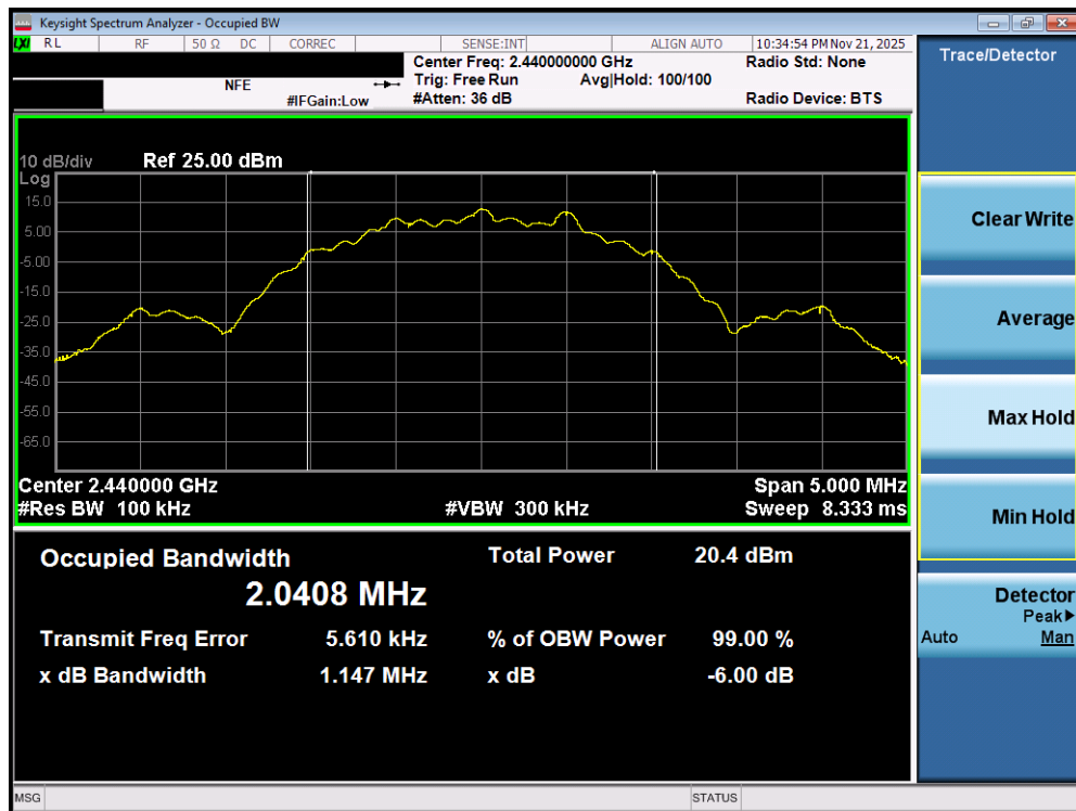
Plot 7-35. 6dB Bandwidth Plot (Bluetooth (LE), 2Mbps – Ch. 17) – Dual Ant 2
