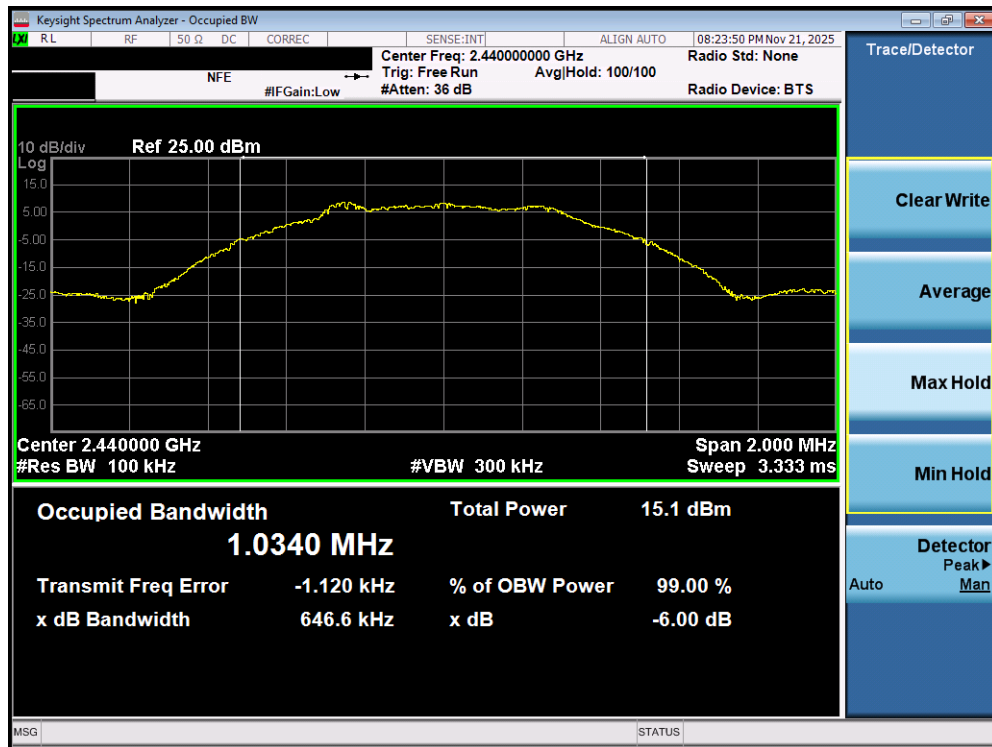
Plot 7-5. 6dB Bandwidth Plot (Bluetooth (LE), 500kbps – Ch. 17) – Ant 1
