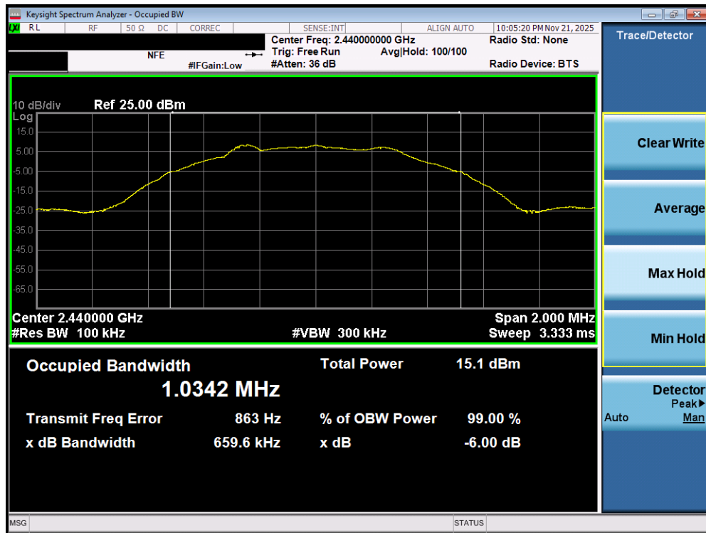
Plot 7-17. 6dB Bandwidth Plot (Bluetooth (LE), 500kbps – Ch. 17) – Ant 2
