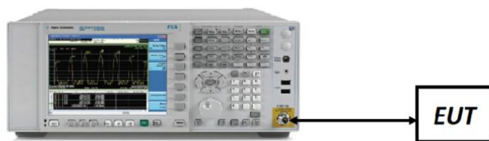
Figure 7-3. Test Instrument & Measurement Setup
