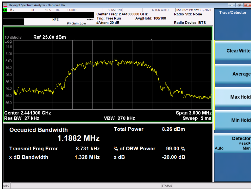
Plot 7-23. 20dB Bandwidth Plot (Bluetooth, 2Mbps – Ch. 39) – Dual Ant 1
