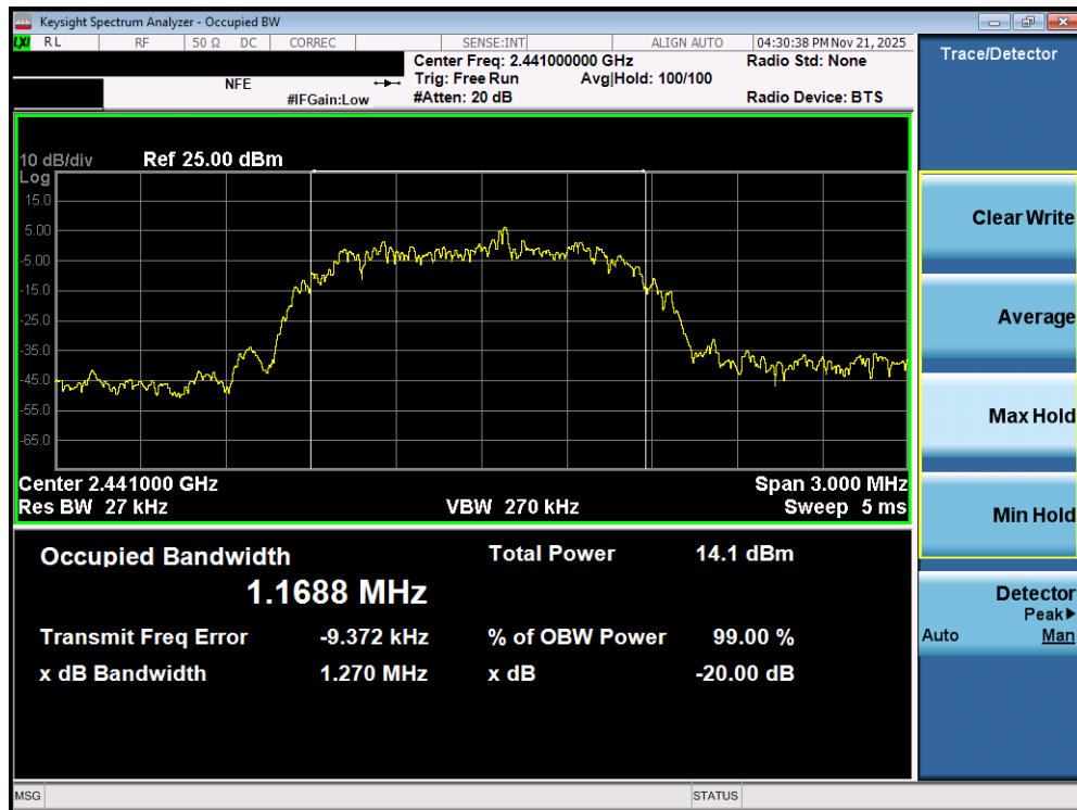
Plot 7-5. 20dB Bandwidth Plot (Bluetooth, 2Mbps – Ch. 39) – Ant 1
