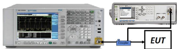
Figure 7-1. Test Instrument & Measurement Setup
