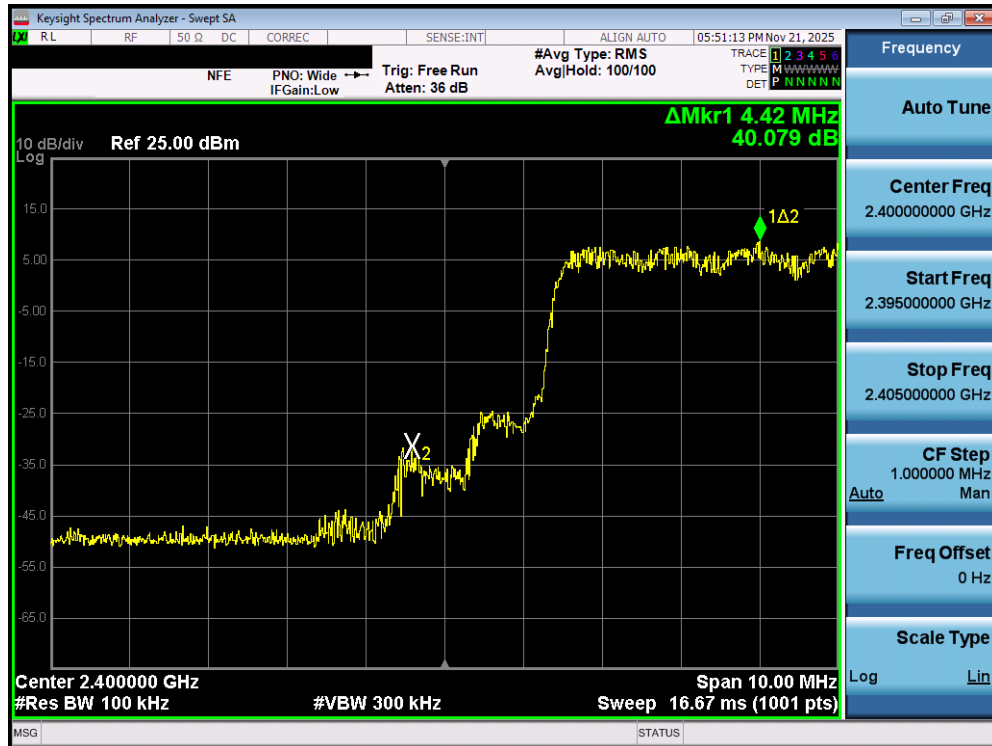
Plot 7-119. Band Edge Plot (Bluetooth with Hopping Enabled, 3 Mbps) – Dual Ant 1
