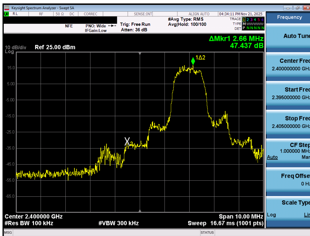
Plot 7-109. Band Edge Plot (Bluetooth with Hopping Disabled, 3 Mbps – Ch. 0) – Ant 1
