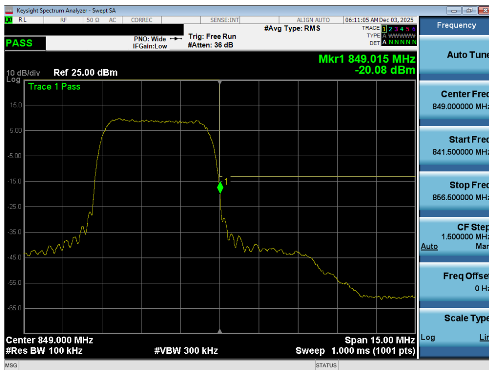
Plot 7-144. Upper Band Edge Plot (WCDMA Cell – Ch. 4233 – Ant1)
