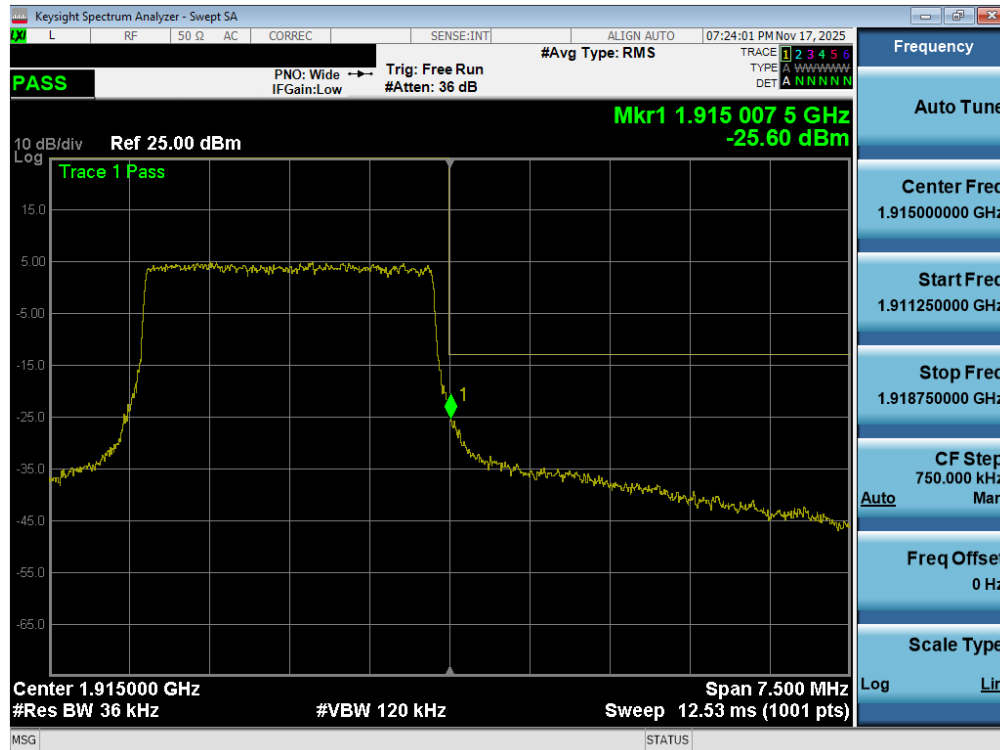
Plot 7-92. Upper Band Edge Plot (LTE Band 25 - 3MHz QPSK – Full RB - Ant1)
