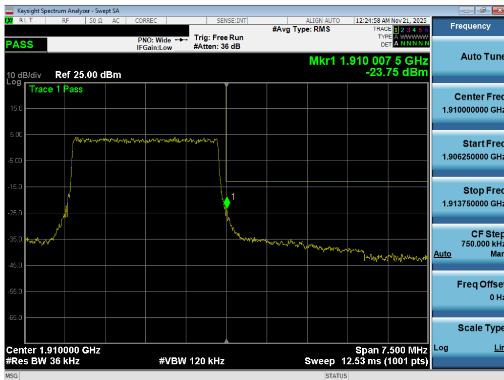
Plot 7-110. Upper Band Edge Plot (LTE Band 2 - 3MHz QPSK - Full RB - Ant2)
