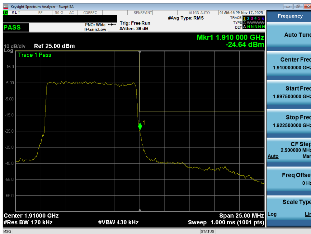
Plot 7-96. Upper Band Edge Plot (NR Band n2 - 10MHz QPSK – Full RB - Ant1)
