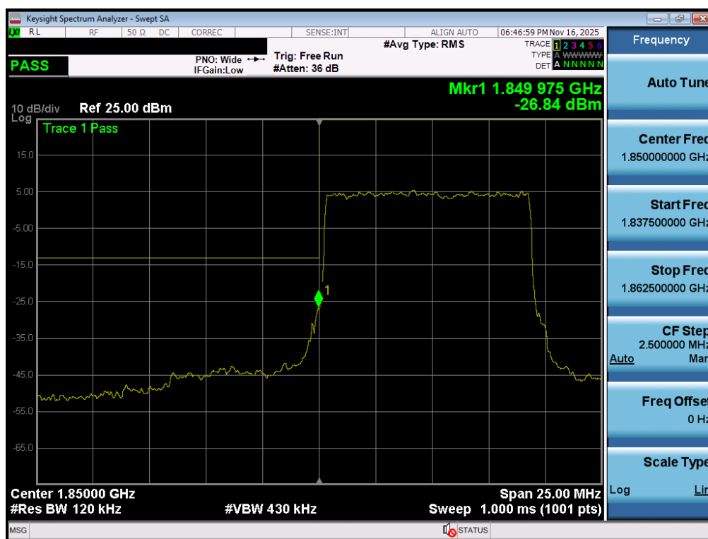
Plot 7-94. Lower Band Edge Plot (NR Band n25/2 - 10MHz QPSK – Full RB - Ant1)
