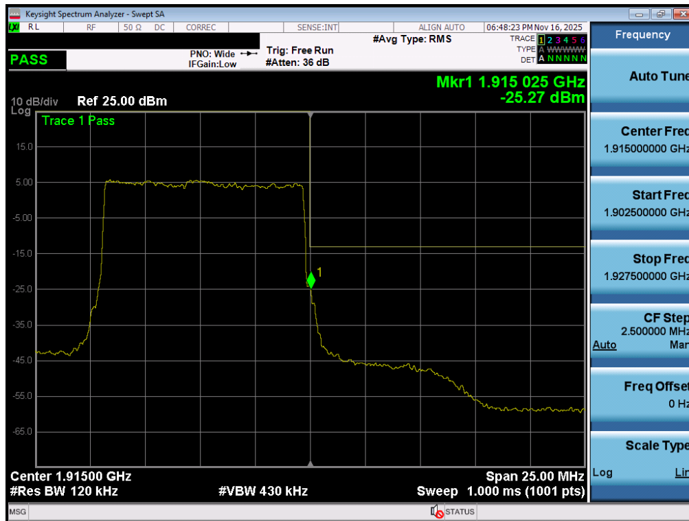
Plot 7-98. Upper Band Edge Plot (NR Band n25 - 10MHz QPSK – Full RB - Ant1)
