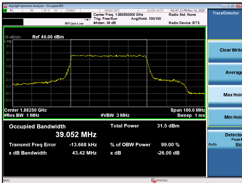
Plot 7-17. Occupied Bandwidth Plot (NR Band n25/2 - 40.0MHz CP-OFDM QPSK - Full RB - ANT1)
