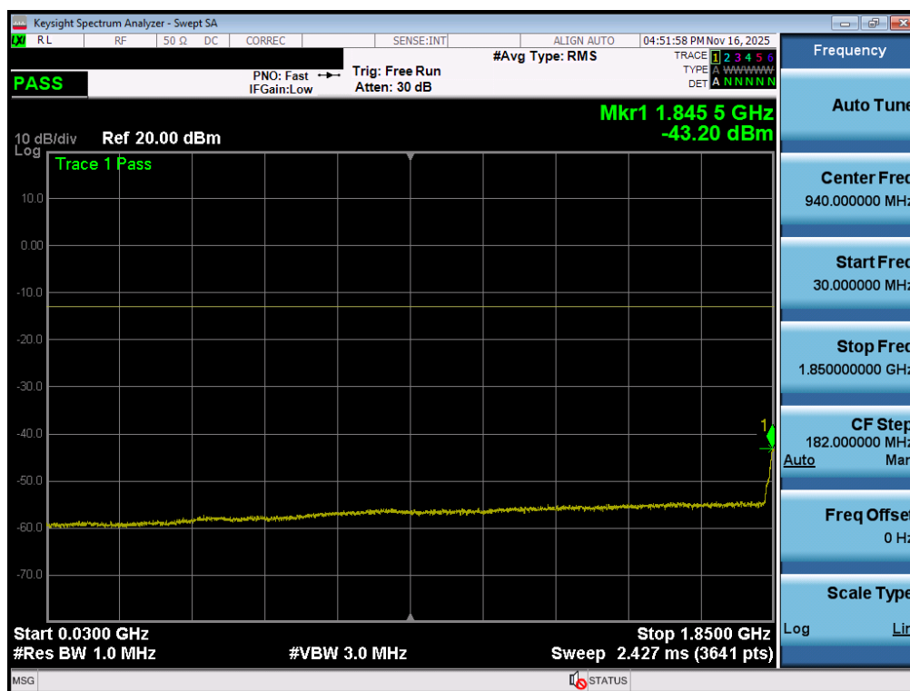
Plot 7-85. Conducted Spurious Plot (NR Band n25/2 - 40.0MHz - 1RB - Low Channel - Ant2)
