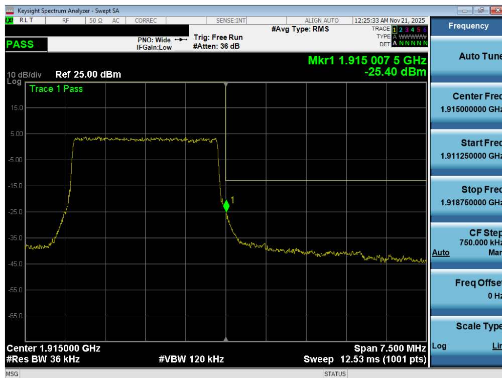
Plot 7-112. Upper Band Edge Plot (LTE Band 25 - 3MHz QPSK – Full RB - Ant2)
