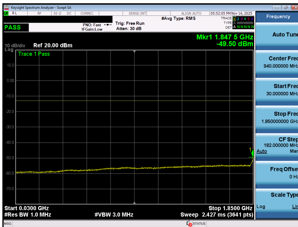
Plot 7-73. Conducted Spurious Plot (NR Band n25/2 - 40.0MHz - 1RB - High Channel - Ant1)
