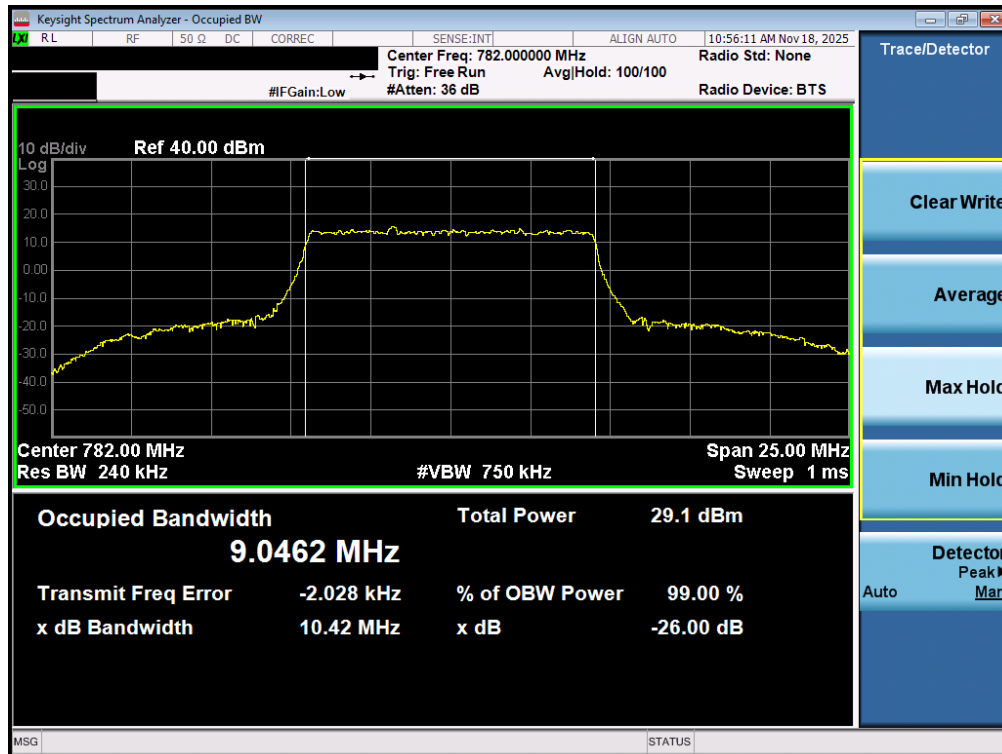
Plot 7-66. Occupied Bandwidth Plot (LTE Band 13 - 10MHz 16-QAM - Full RB – ANT2)
