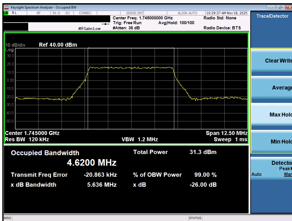
Plot 7-75. Occupied Bandwidth Plot (LTE Band 66/4 - 5MHz QPSK - Full RB - ANT2)
