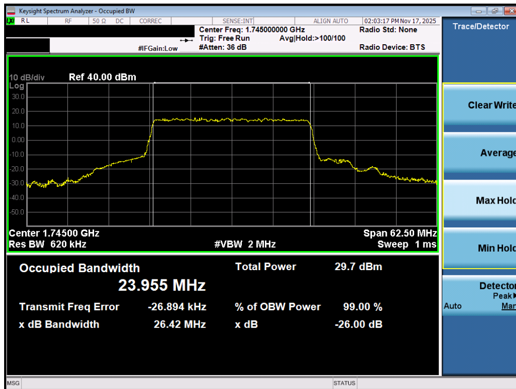
Plot 7-42. Occupied Bandwidth Plot (NR Band n66 - 25.0MHz CP-OFDM QPSK - Full RB – ANT1)
