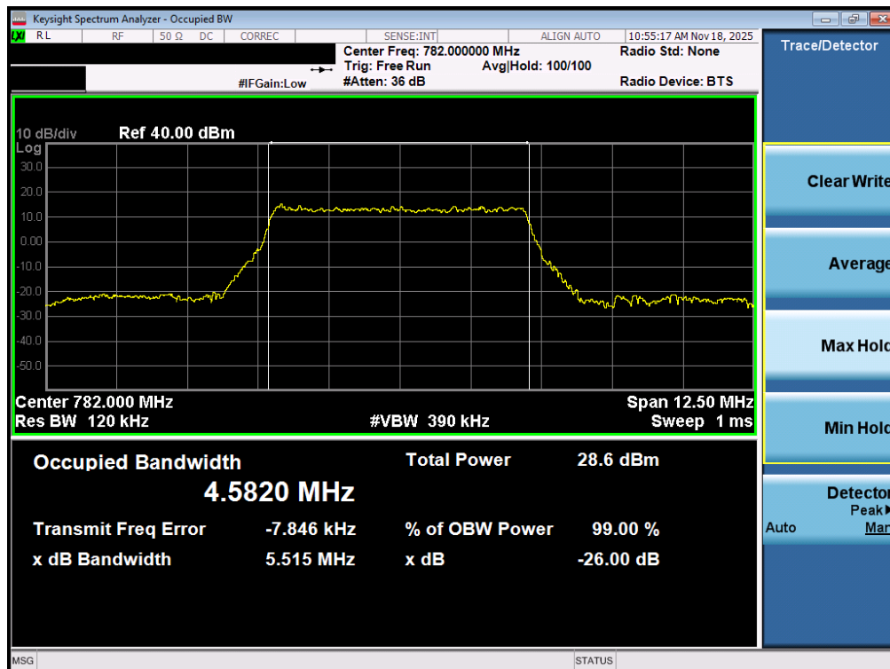
Plot 7-68. Occupied Bandwidth Plot (LTE Band 13 - 5MHz 16-QAM - Full RB – ANT2)
