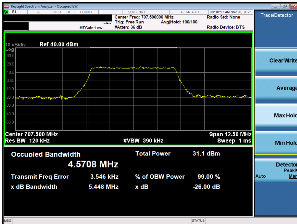
Plot 7-5. Occupied Bandwidth Plot (LTE Band 12/17 - 5MHz 16-QAM - Full RB – ANT1)
