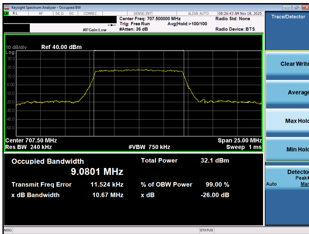
Plot 7-2. Occupied Bandwidth Plot (LTE Band 12/17 - 10MHz QPSK - Full RB – ANT1)
