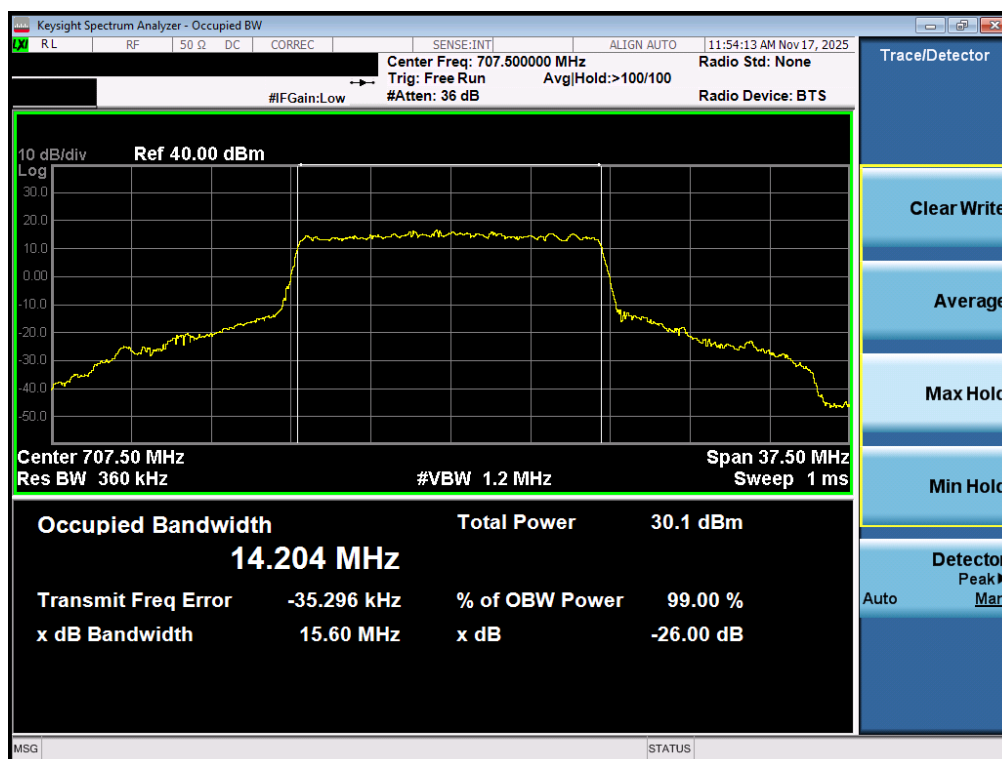
Plot 7-28. Occupied Bandwidth Plot (NR Band n12 - 15MHz CP-OFDM 16-QAM - Full RB - ANT1)
