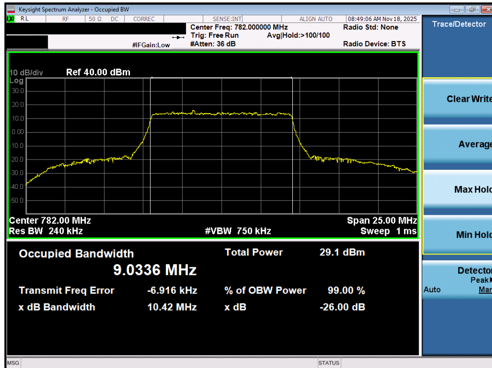
Plot 7-11. Occupied Bandwidth Plot (LTE Band 13 - 10MHz 16-QAM - Full RB – ANT1)
