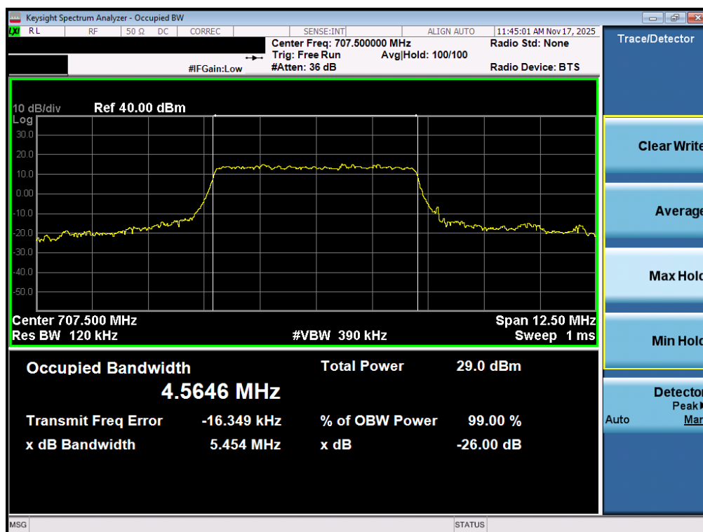
Plot 7-34. Occupied Bandwidth Plot (NR Band n12 - 5MHz CP-OFDM 16-QAM - Full RB - ANT1)
