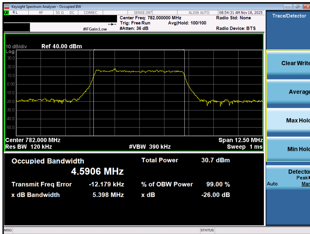
Plot 7-12. Occupied Bandwidth Plot (LTE Band 13 - 5MHz QPSK - Full RB – ANT1)
