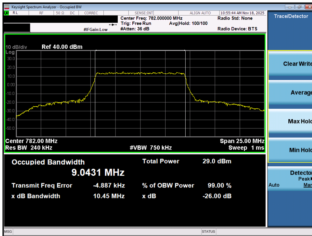
Plot 7-65. Occupied Bandwidth Plot (LTE Band 13 - 10MHz QPSK - Full RB – ANT2)
