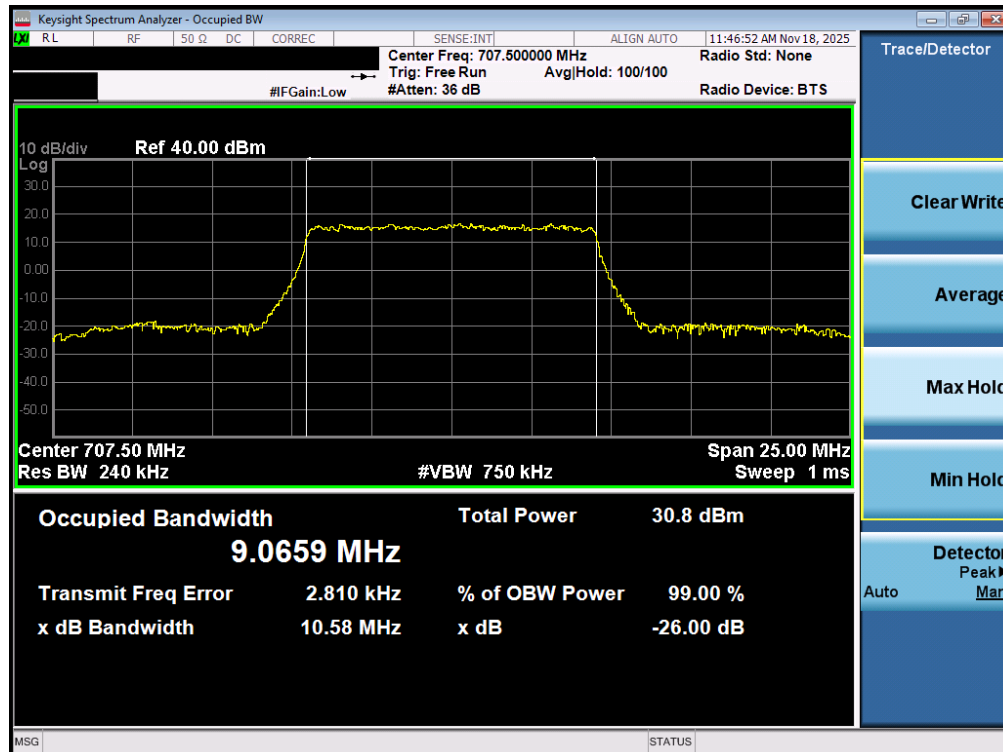
Plot 7-58. Occupied Bandwidth Plot (LTE Band 12/17 - 10MHz 16-QAM - Full RB – ANT2)
