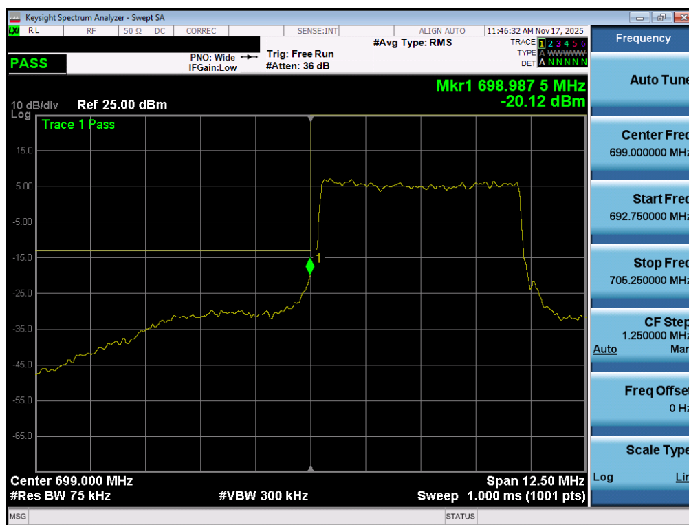
Plot 7-163. Lower Band Edge Plot (NR Band n12 – 5.0MHz - Full RB - ANT1)
