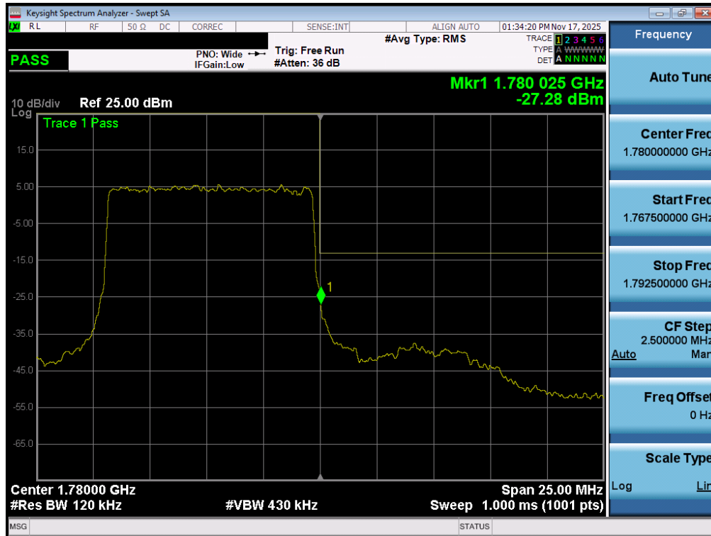
Plot 7-167. Upper Band Edge Plot (NR Band n66 – 10.0MHz - Full RB - ANT1)
