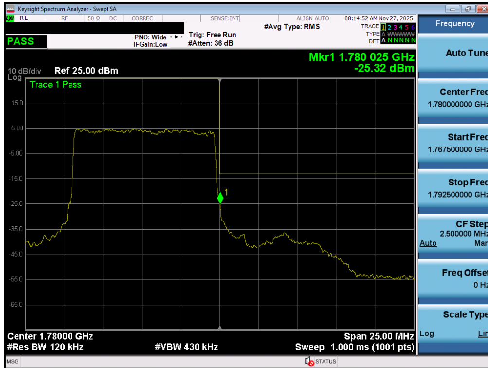
Plot 7-189. Upper Band Edge Plot (NR Band n66 – 10.0MHz - Full RB - ANT2)
