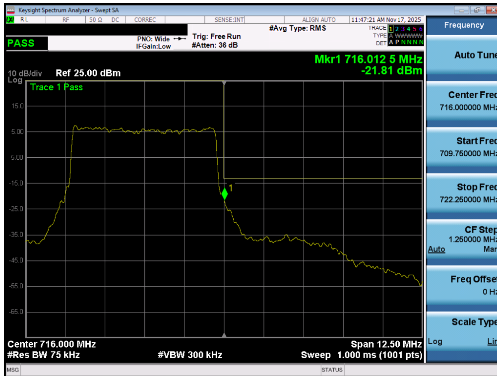
Plot 7-164. Upper Band Edge Plot (NR Band n12 – 5.0MHz - Full RB - ANT1)
