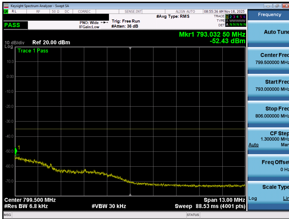
Plot 7-156. Upper Emission Mask Plot (LTE Band 13 - 5MHz QPSK - Full RB - ANT1)
