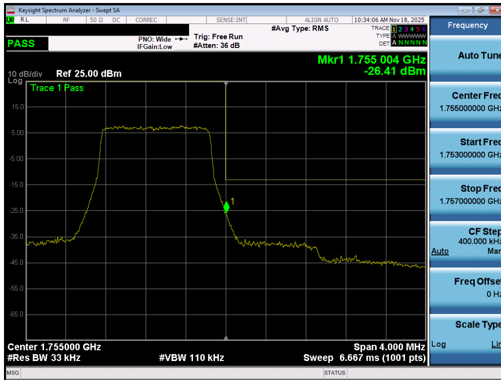
Plot 7-181. Upper Band Edge Plot (LTE Band 4 – 1.4MHz QPSK – Full RB - ANT2)
