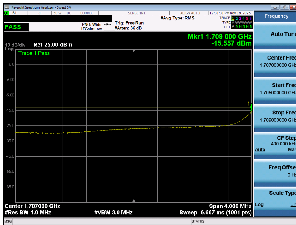
Plot 7-170. Lower Extended Band Edge Plot (WCDMA AWS – Ch. 1312 – ANT2)
