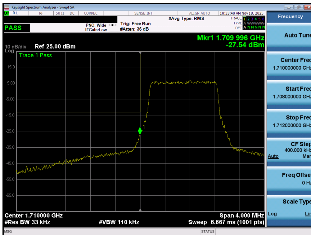
Plot 7-179. Lower Band Edge Plot (LTE Band 66/4 – 1.4MHz QPSK – Full RB - ANT2)
