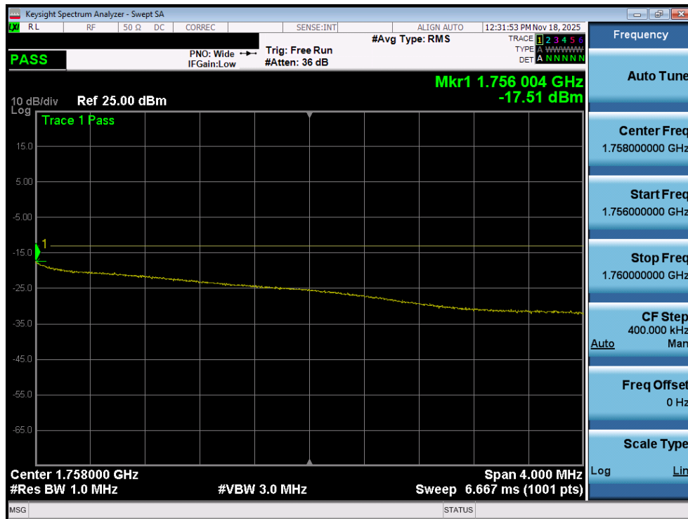
Plot 7-172. Upper Extended Band Edge Plot (WCDMA AWS – Ch. 1513– ANT2)
