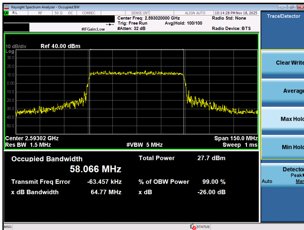
Plot 7-30. Occupied Bandwidth Plot (NR Band n41 PC3 – 60MHz QPSK – Full RB – Ant1)
