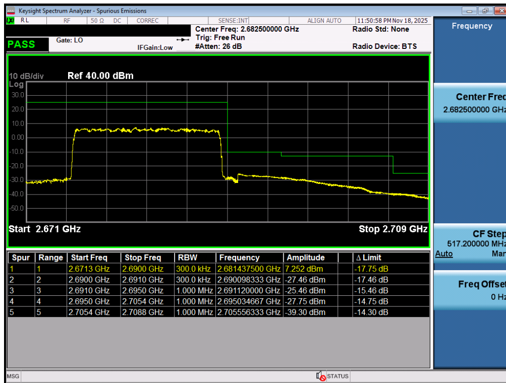
Plot 7-118. Upper ACP Plot (LTE Band 41(PC2) - 15MHz QPSK – Full RB – Ant2)
