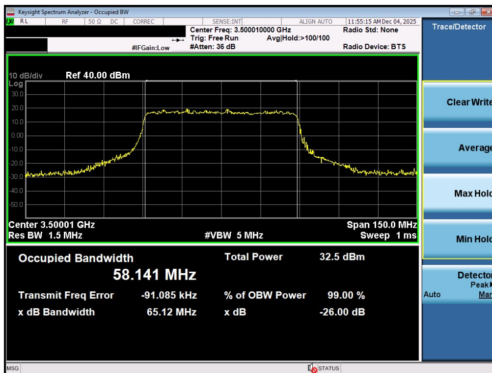
Plot 7-15. Occupied Bandwidth Plot (NR Band n77 - 60MHz 16-QAM - Full RB - Ant1 - DoD Band - Main)
