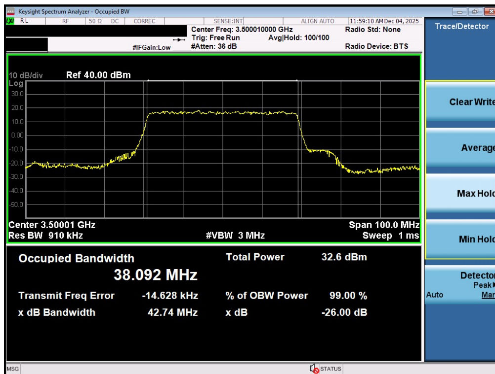
Plot 7-20. Occupied Bandwidth Plot (NR Band n77 - 40MHz QPSK - Full RB - Ant1 - DoD Band - Main)
