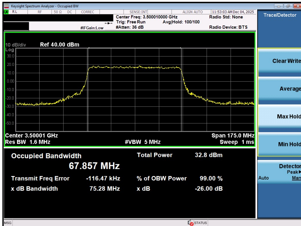
Plot 7-12. Occupied Bandwidth Plot (NR Band n77 - 70MHz 16-QAM - Full RB - Ant1 - DoD Band - Main)
