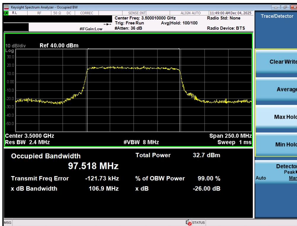
Plot 7-3. Occupied Bandwidth Plot (NR Band n77PC2 - 100MHz 16-QAM - Full RB - Ant1 - DoD Band - Main)
