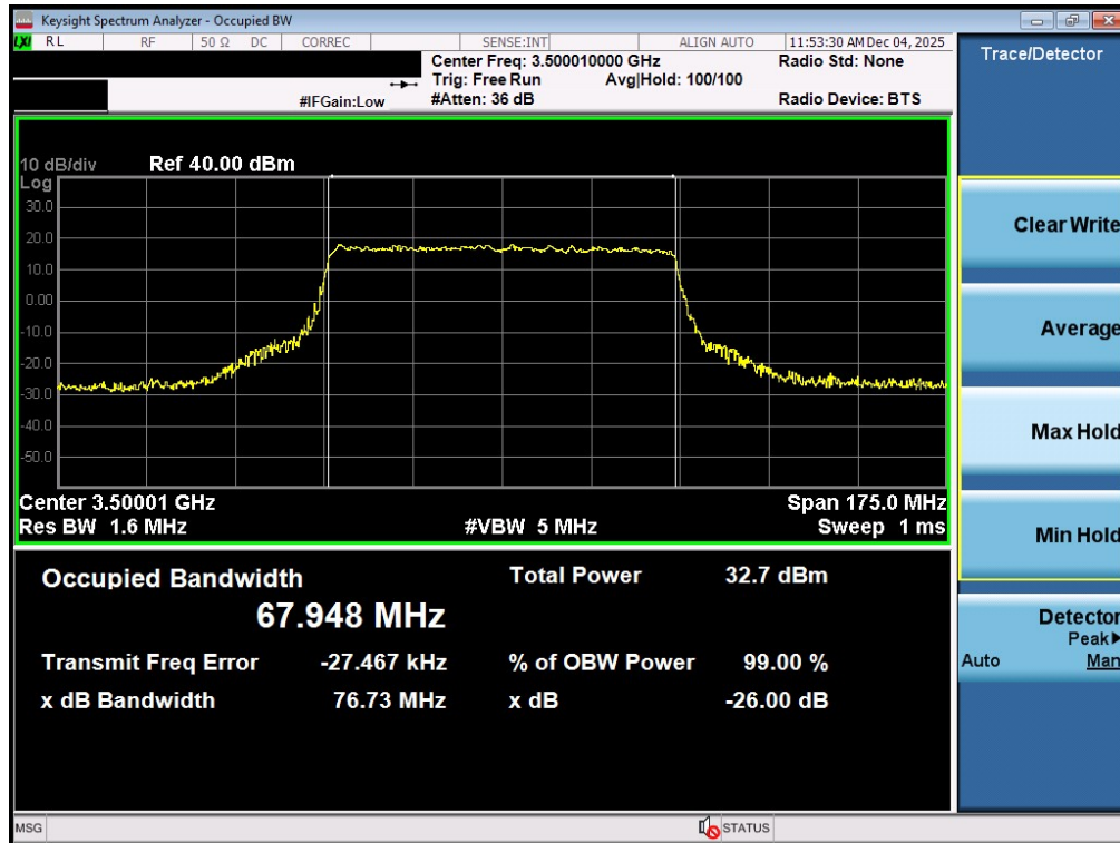
Plot 7-11. Occupied Bandwidth Plot (NR Band n77 - 70MHz QPSK - Full RB - Ant1 - DoD Band - Main)
