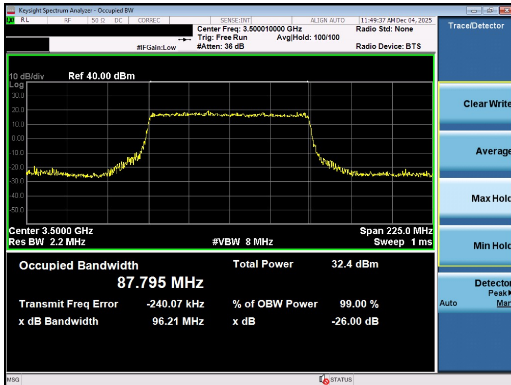
Plot 7-6. Occupied Bandwidth Plot (NR Band n77 - 90MHz 16-QAM - Full RB - Ant1 - DoD Band - Main)
