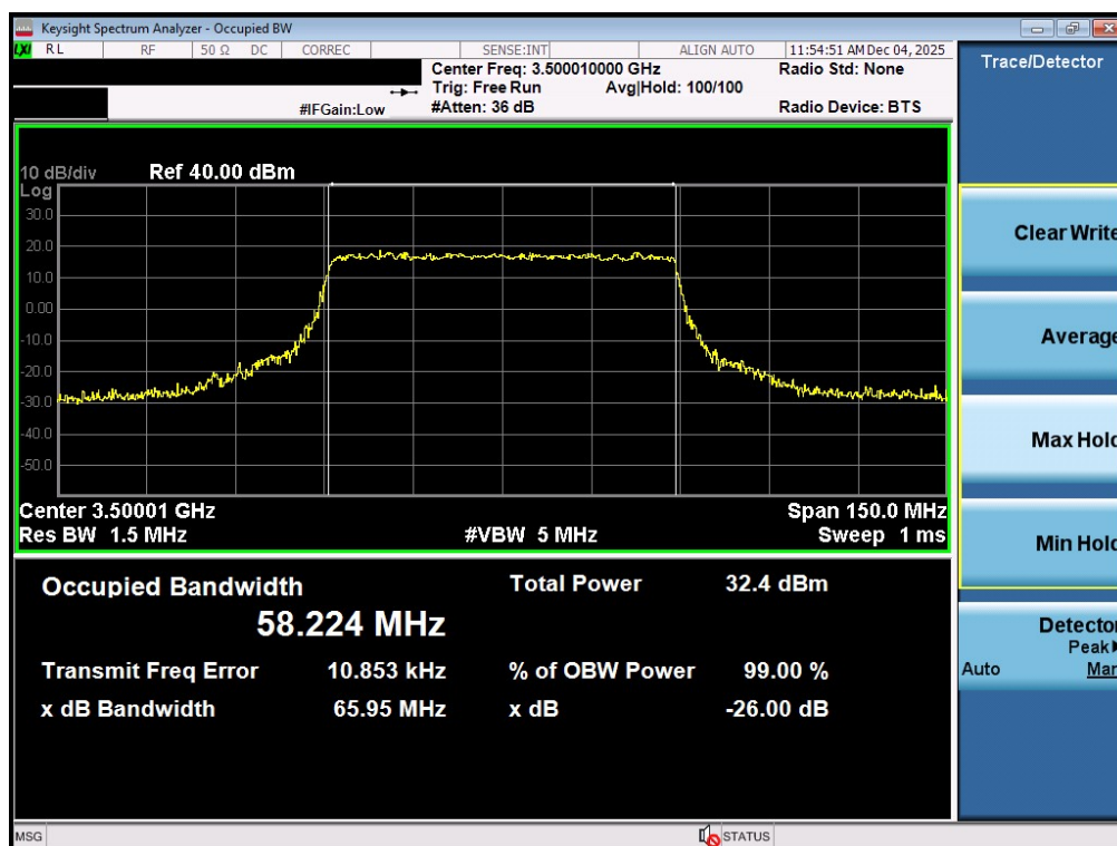
Plot 7-14. Occupied Bandwidth Plot (NR Band n77 - 60MHz QPSK - Full RB - Ant1 - DoD Band - Main)
