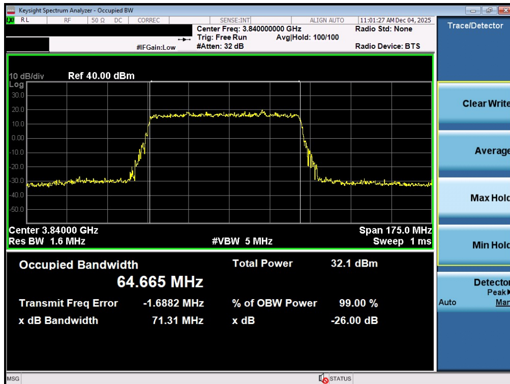
Plot 7-43. Occupied Bandwidth Plot (NR Band n77 - 70MHz \pi/2 BPSK - Full RB - Ant1 - C-Band - Main)
