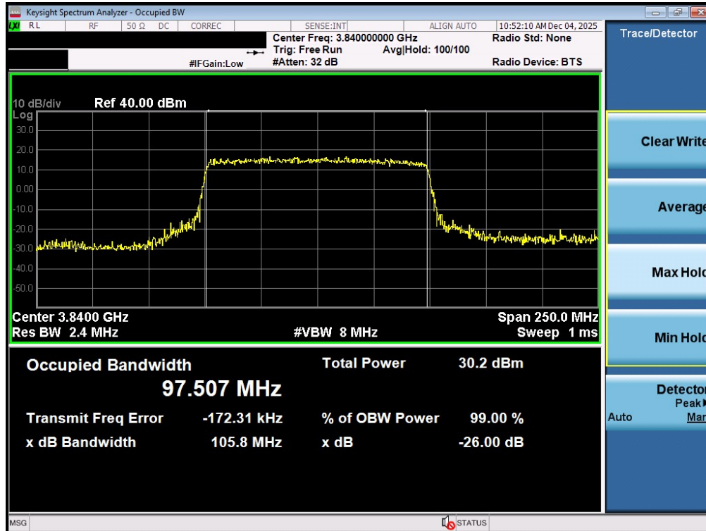
Plot 7-35. Occupied Bandwidth Plot (NR Band n77PC2 - 100MHz QPSK - Full RB - Ant1 - C-Band - Main)
