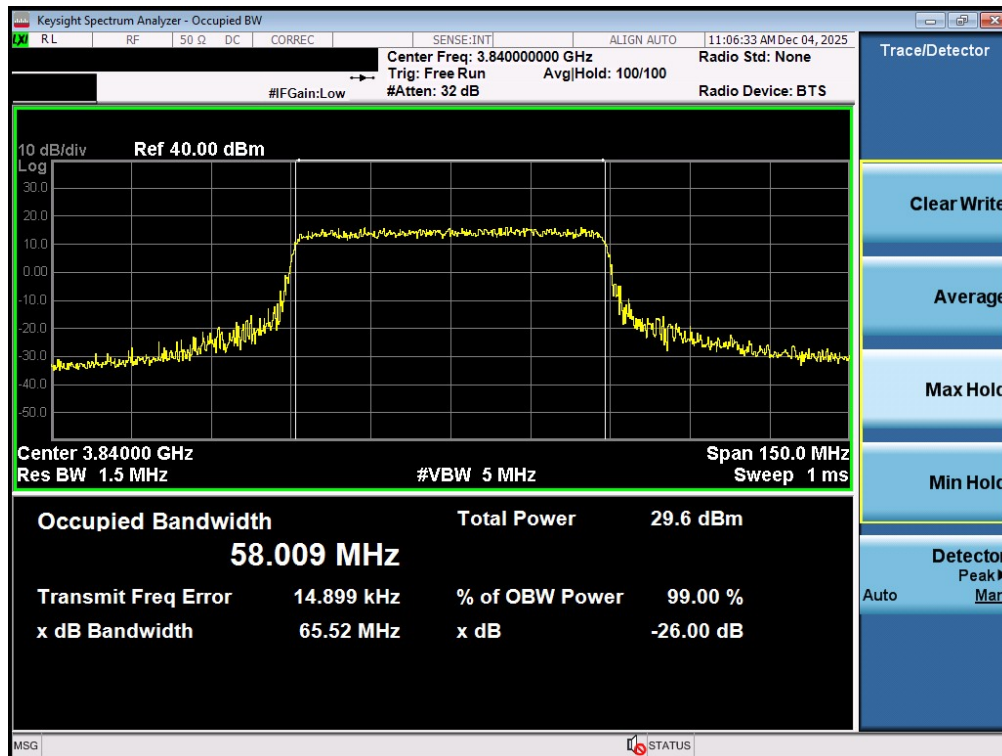
Plot 7-47. Occupied Bandwidth Plot (NR Band n77 - 60MHz QPSK - Full RB - Ant1 - C-Band - Main)
