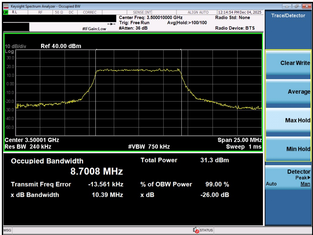
Plot 7-33. Occupied Bandwidth Plot (NR Band n77 - 10MHz 16-QAM - Full RB - Ant1 - DoD Band - Main)
