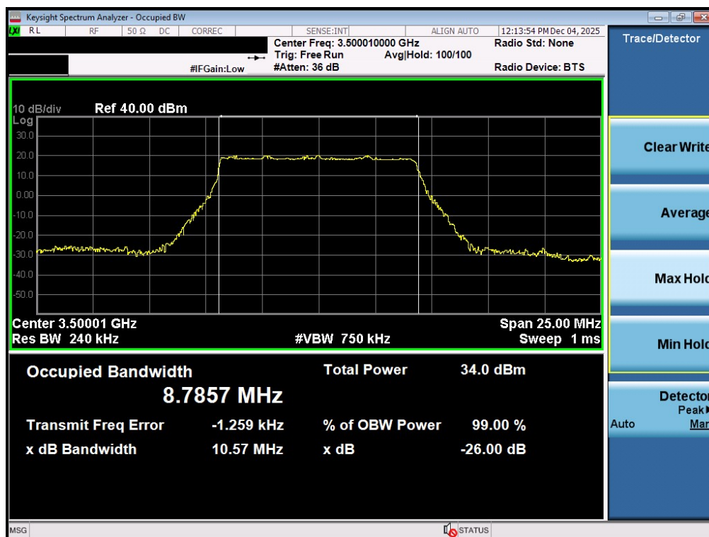
Plot 7-31. Occupied Bandwidth Plot (NR Band n77 - 10MHz \pi/2 BPSK - Full RB - Ant1 - DoD Band - Main)
