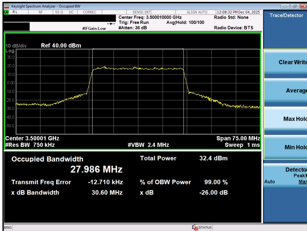
Plot 7-23. Occupied Bandwidth Plot (NR Band n77 - 30MHz QPSK - Full RB - Ant1 - DoD Band - Main)
