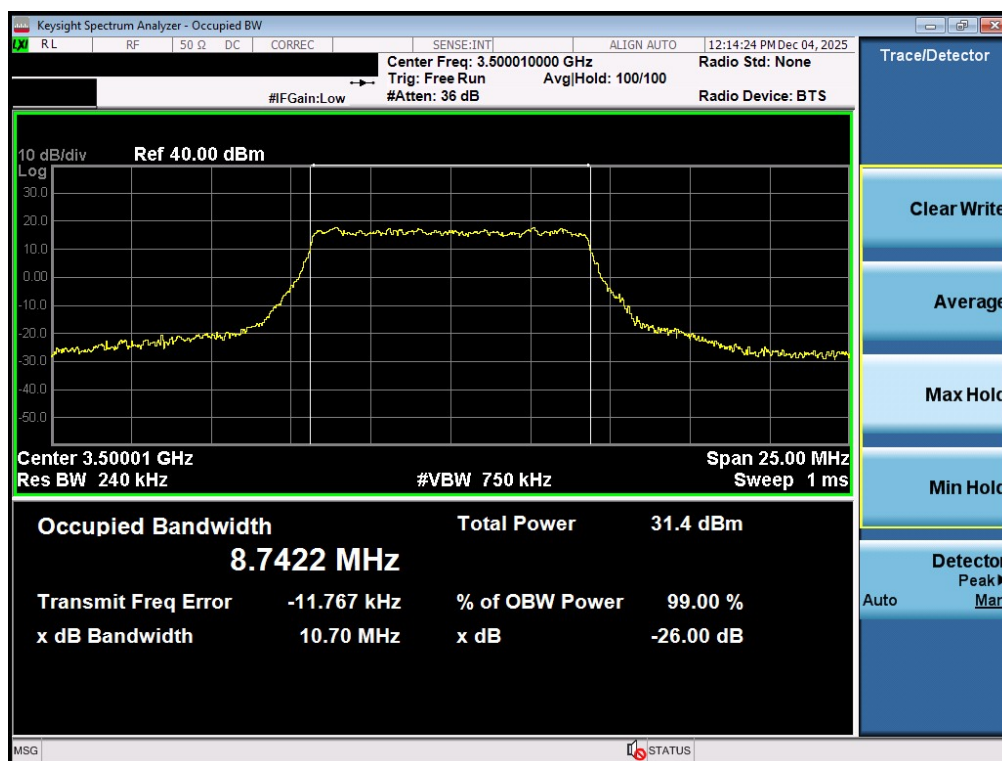
Plot 7-32. Occupied Bandwidth Plot (NR Band n77 - 10MHz QPSK - Full RB - Ant1 - DoD Band - Main)
