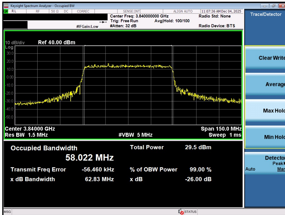
Plot 7-48. Occupied Bandwidth Plot (NR Band n77 - 60MHz 16-QAM - Full RB - Ant1 - C-Band - Main)
