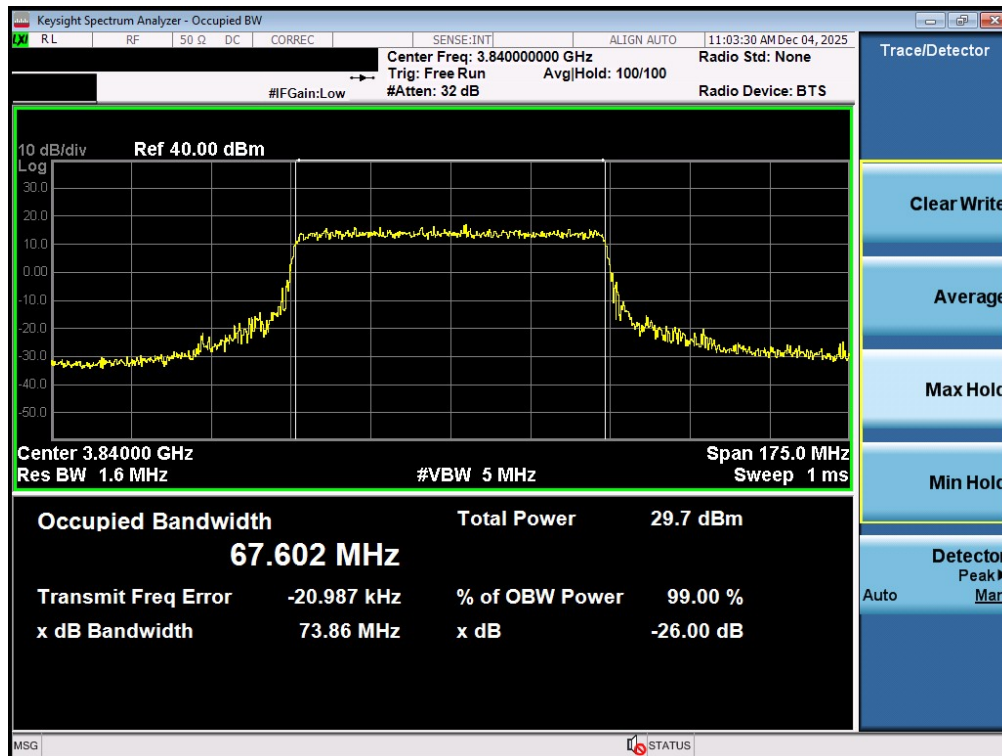
Plot 7-45. Occupied Bandwidth Plot (NR Band n77 - 70MHz 16-QAM - Full RB - Ant1 - C-Band - Main)
