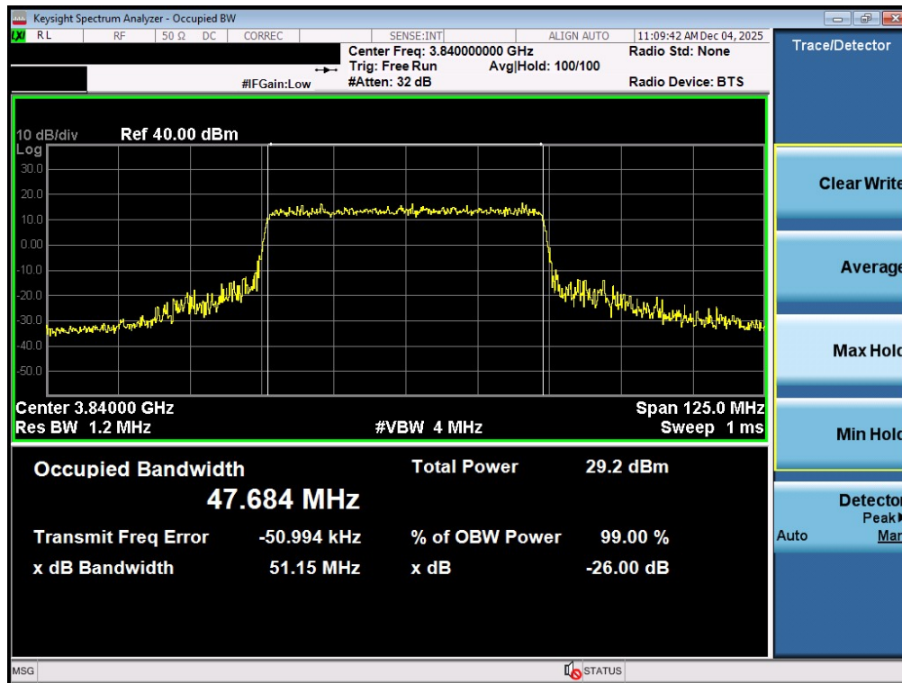
Plot 7-50. Occupied Bandwidth Plot (NR Band n77 - 50MHz QPSK - Full RB - Ant1 - C-Band - Main)
