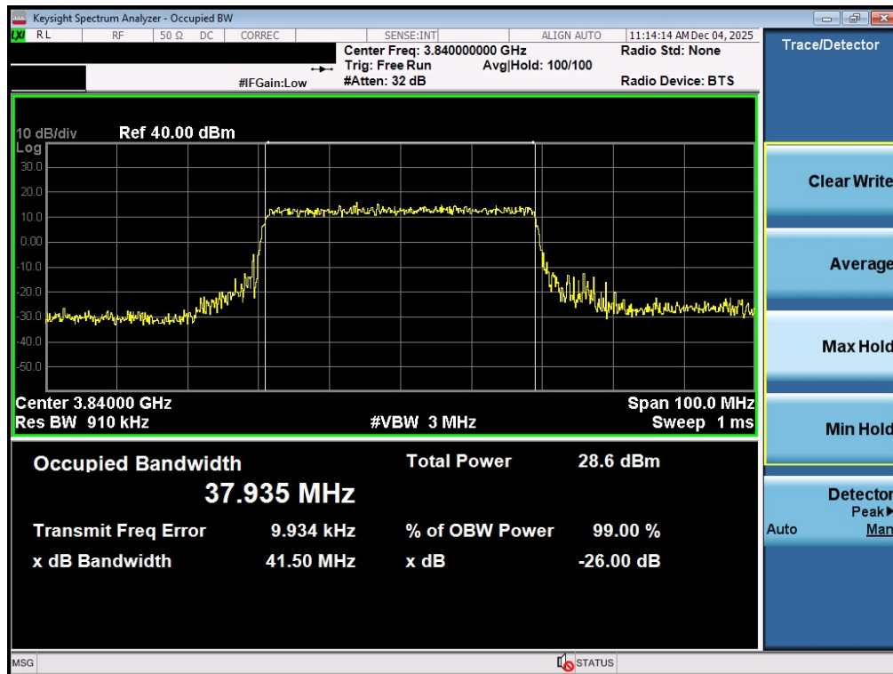
Plot 7-53. Occupied Bandwidth Plot (NR Band n77 - 40MHz QPSK - Full RB - Ant1 - C-Band - Main)
