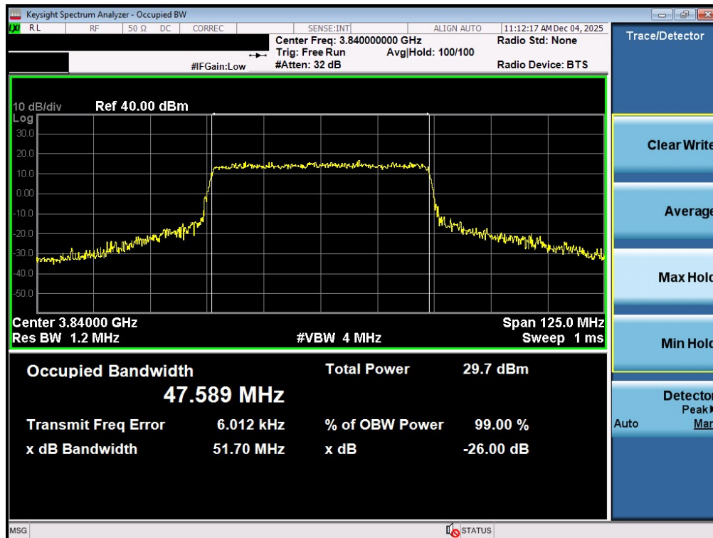
Plot 7-51. Occupied Bandwidth Plot (NR Band n77 - 50MHz 16-QAM - Full RB - Ant1 - C-Band - Main)
