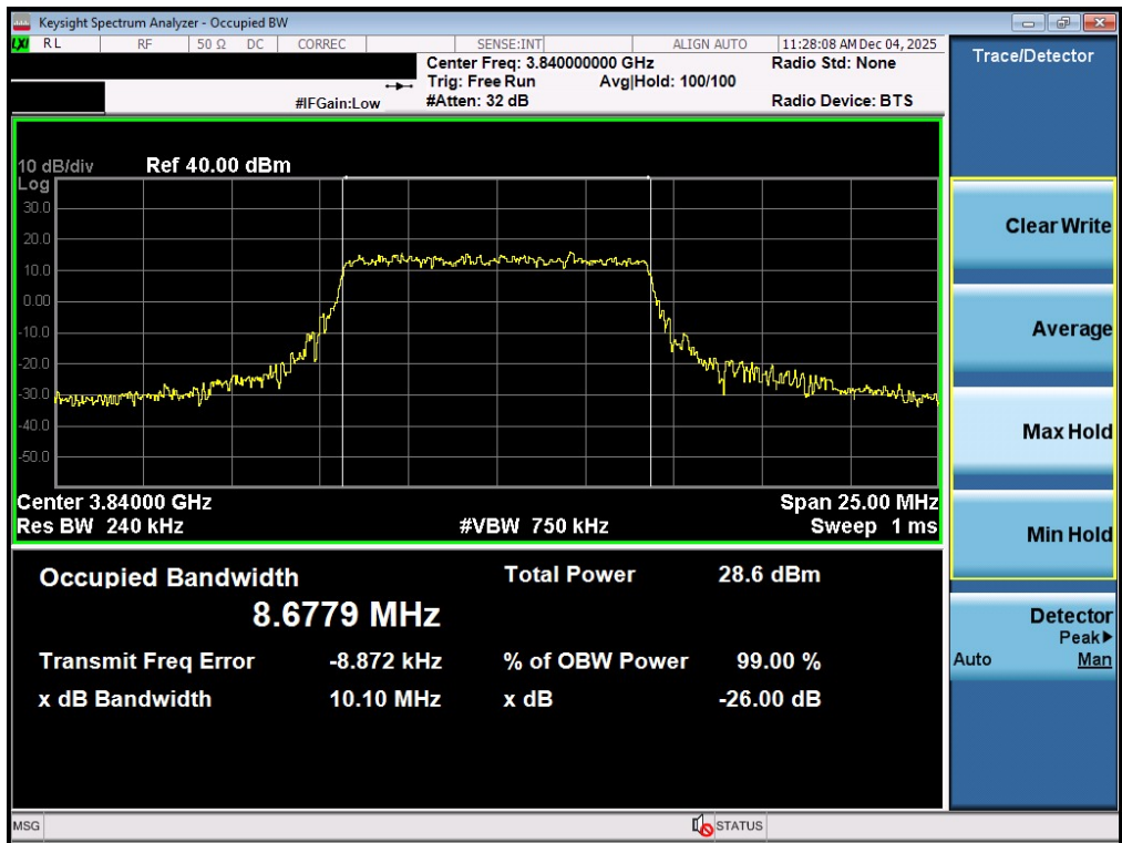
Plot 7-66. Occupied Bandwidth Plot (NR Band n77 - 10MHz 16-QAM - Full RB - Ant1 - C-Band - Main)
