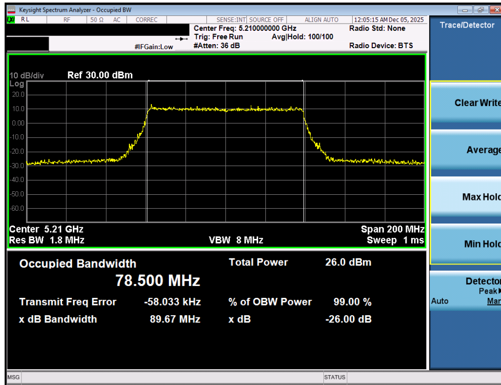
Plot 7-7. 26dB Bandwidth Plot MIMO ANT1 (80MHz BW 802.11be (UNII Band 1) – Ch. 42)
