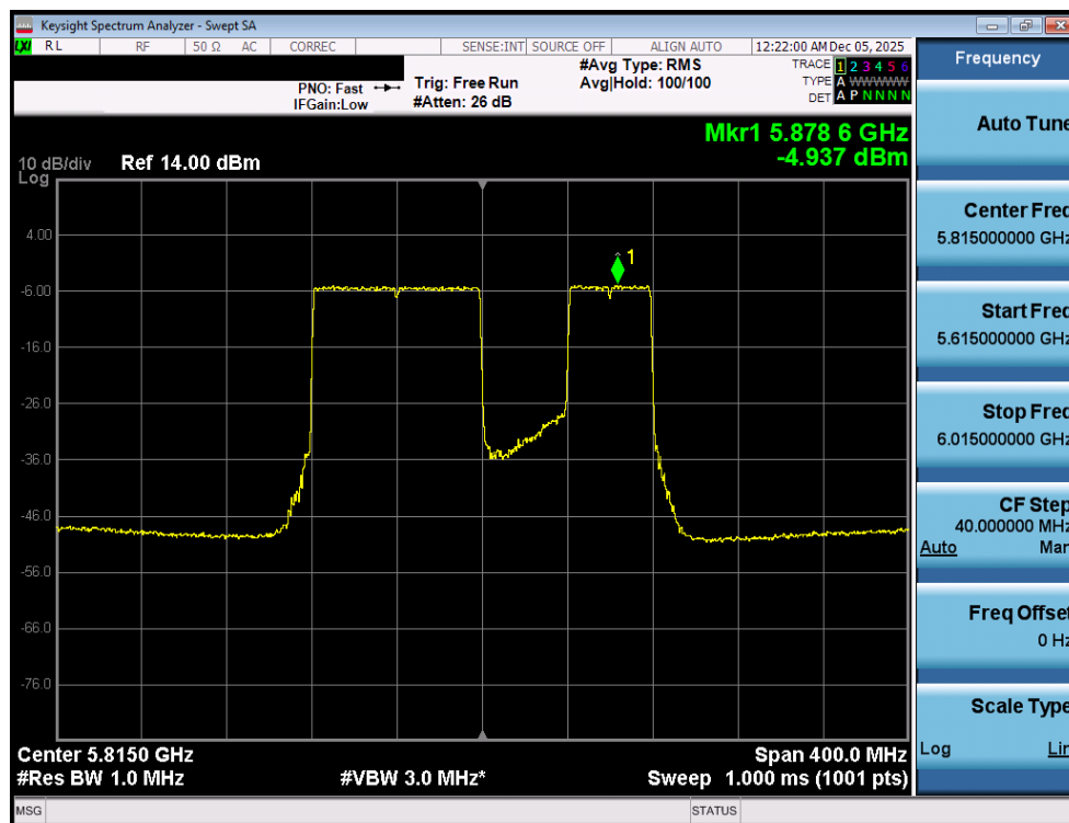
Plot 7-91. Power Spectral Density Plot MIMO ANT1 (160MHz BW 802.11be (40MHz Puncture) (UNII Band 3/4) – Ch. 163)
