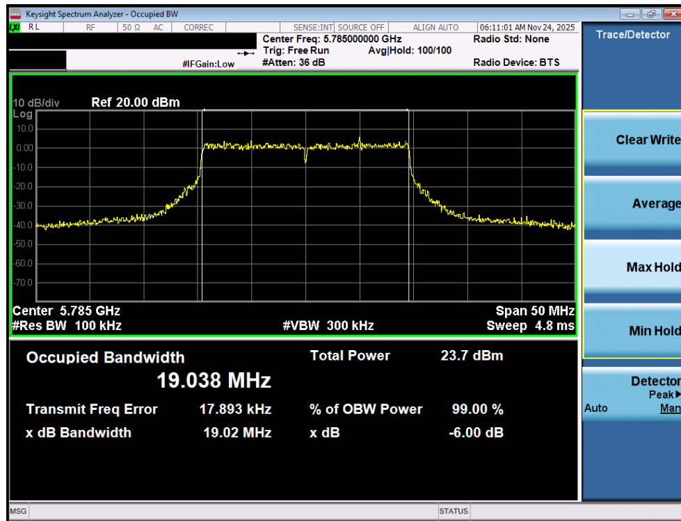
Plot 7-26. 6dB Bandwidth Plot MIMO ANT1 (20MHz BW 802.11be (UNII Band 3) – Ch. 157)
