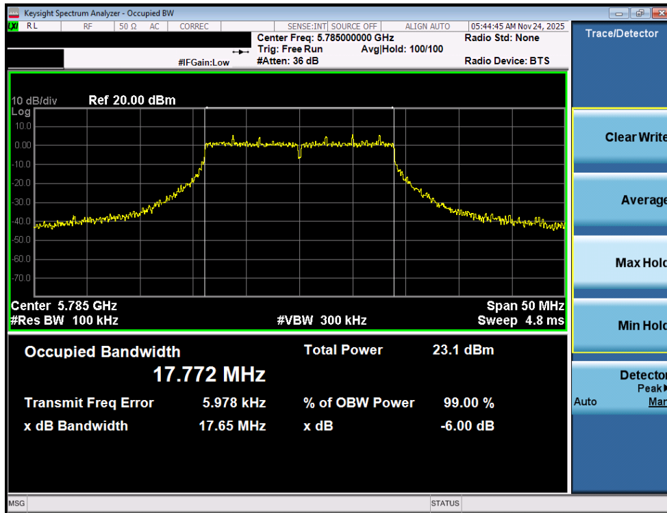
Plot 7-25. 6dB Bandwidth Plot MIMO ANT1 (20MHz BW 802.11n (UNII Band 3) – Ch. 157)
