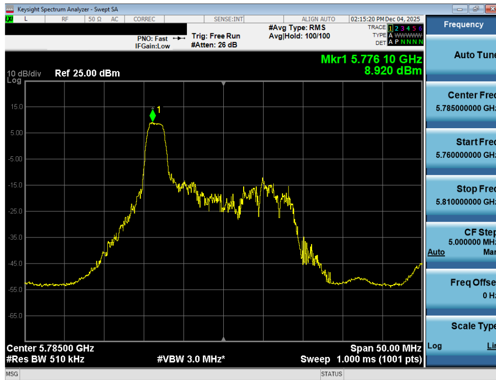
Plot 7-71. Power Spectral Density Plot MIMO ANT2 (20MHz BW 802.11be – 26 Tones (UNII Band 3) – Ch. 157)
