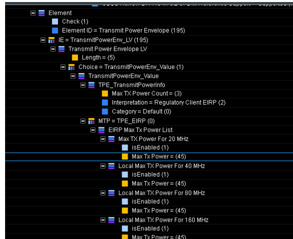
Figure 7-7. Callbox Power Authorization – 22.50dBm
