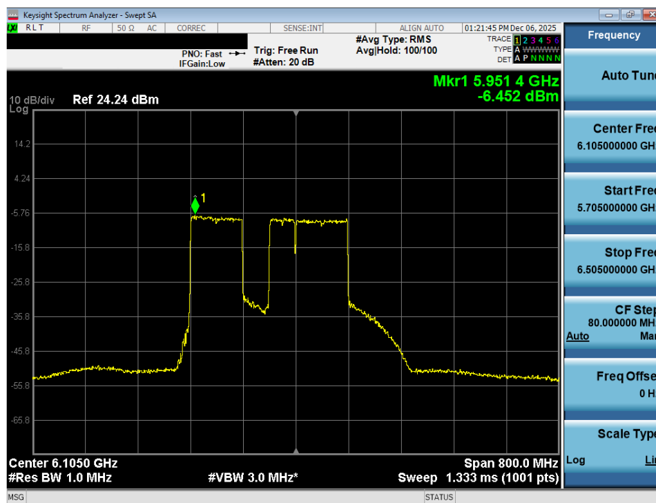
Plot 7-45. Power Spectral Density Plot MIMO ANT2 (320MHz 802.11be (UNII Band 5) – Ch. 31) – 120MHz Punctured – LPI/SP
